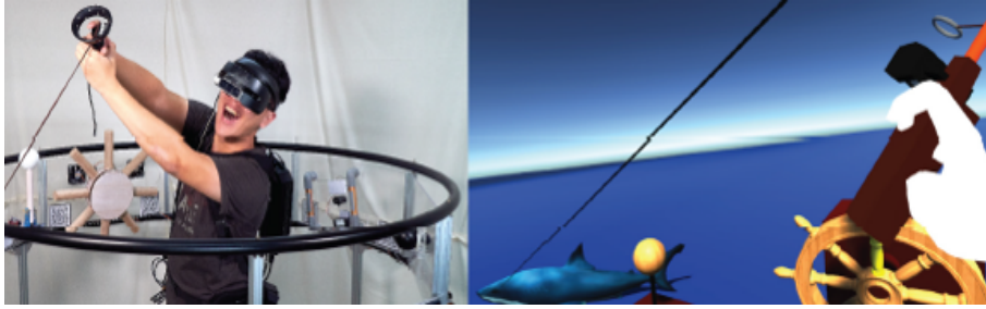
Figure 1.41 – Grounded fixed platform ETHD presented by Huang et al. [4]. This work presented several ludic scenarios. The scenario depicted in this figure recreated a virtual boat. Users could navigate the boat, go fishing, and shoot cannonballs thanks to the passive props used as tangible elements in their virtual scenario.
