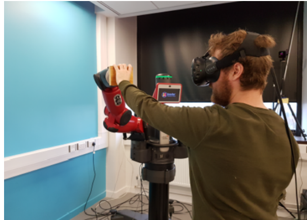
Figure 1.27 – VR-based HMD used in the ETHD system by Brice et al. [44]. The proposed ETHD used an HTC Vive VR-based HMD as a tool to display the VE that contextualized the haptic feedback coming from the occluded haptic display.
