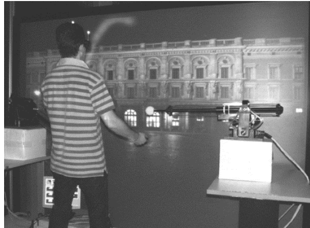
Figure 1.26 – Screen display used in the ETHD system by Ruffaldi et al. [40]. The proposed ETHD used an stereoscopic projection over a screen to display the juggling balls that were rendered by their system for the task of virtual juggling in a VE.
