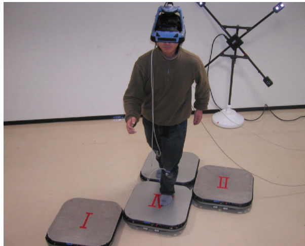
Figure 1.38 – Ungrounded mobile platform ETHD presented by Iwata et al. [28]. This device was designed mainly for locomotion.
