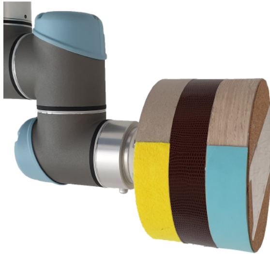
Figure 4.3 – The designed cylindrical prop for representing our approach. This prop can hold different textures which are used to render flat surfaces in a VE. Textures such as cork, foam, felt, leather, cardboard and wood are displayed on this figure. In this case, the leather texture covers the prop’s whole circumference, this permits to render this texture in an infinite way as long as the prop spins below users’ fingers.
