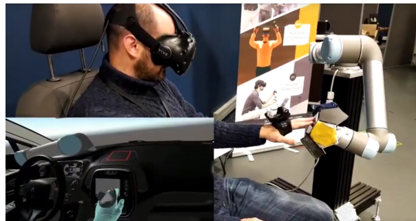
Figure 2 – The LobbyBot project setup. This figure showcases the "LobbyBot" prototype using a Universal Robots UR5 robotic arm and a multi-textured prop for rendering haptic feedback when users explored a car cockpit in virtual reality with their sense of touch.
