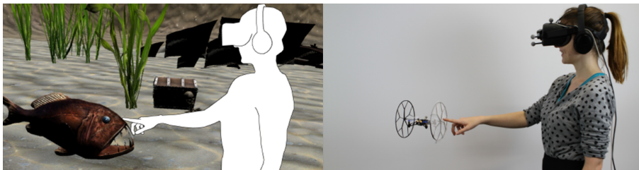
Figure 1.9 – Ungrounded UAV ETHD proposed by Hoppe et al. [5]. This research work presents an ETHD using an ungrounded UAV holding a static surface display that served as the part that physically represented the surfaces to touch in their VE.
