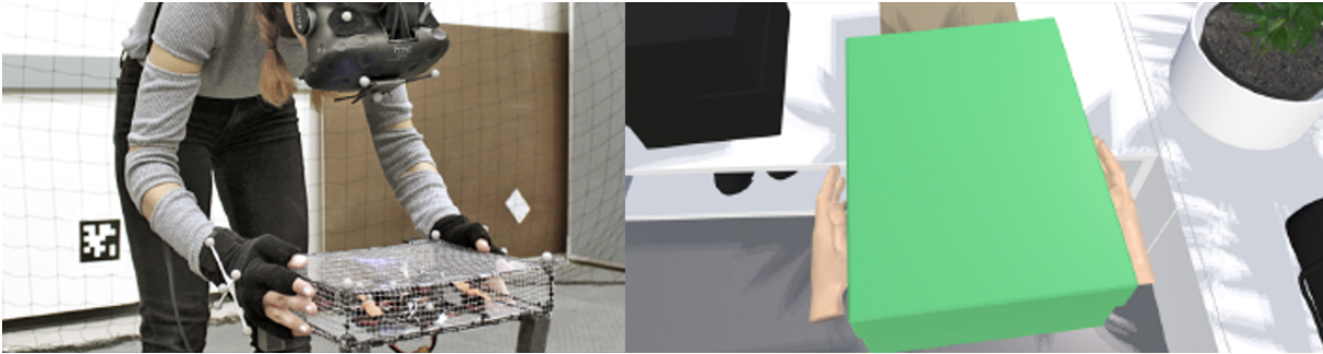
Figure 1.15 – The volume shape display presented by Abtahi et al. [15]. This research work profits from the cage surrounding the UAV by using it as a shape display for representing objects that can be grasped in their use-case scenario.
