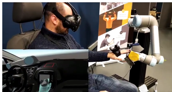
Figure 2 – The LobbyBot project setup. This figure showcases the "LobbyBot" prototype using a Universal Robots UR5 robotic arm and a multi-textured prop for rendering haptic feedback when users explored a car cockpit in virtual reality with their sense of touch.
