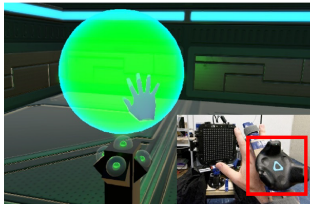
Figure 1.24 – Marker-based tracking system presented by Howard et al. [51] (Highlighted in red). The proposed ETHD used a Vive Tracker as a tool to track the users' hand in their system.
