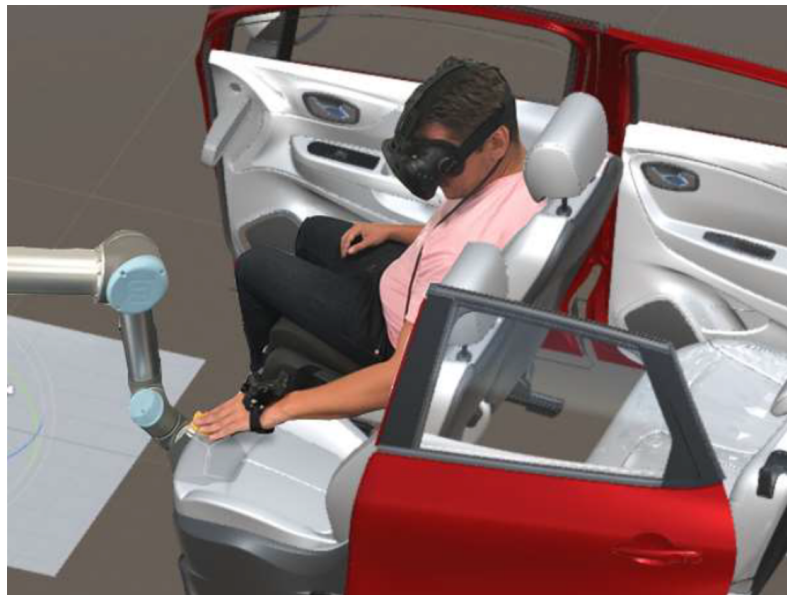
Figure 1.40 – Grounded robotic arm ETHD by Posselt et al. [2]. The VE consists of a recreation of an automobile interior. This research work uses a multi-textured prop attached to a grounded ETHD’s surface display. This configuration permitted to recreate the different textures available to touch at a virtual car cockpit. This ETHD system was conceived for industry applications related to virtual prototyping.
