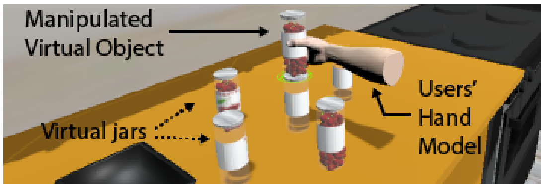
Figure 5.7 – Unconstrained manipulation of multiple objects. In this scenario, the user faces a table holding five jars in arbitrary locations. Users are free to pick up any jar, manipulate it and place it back wherever they please, which includes stacking jars on top of each other.
