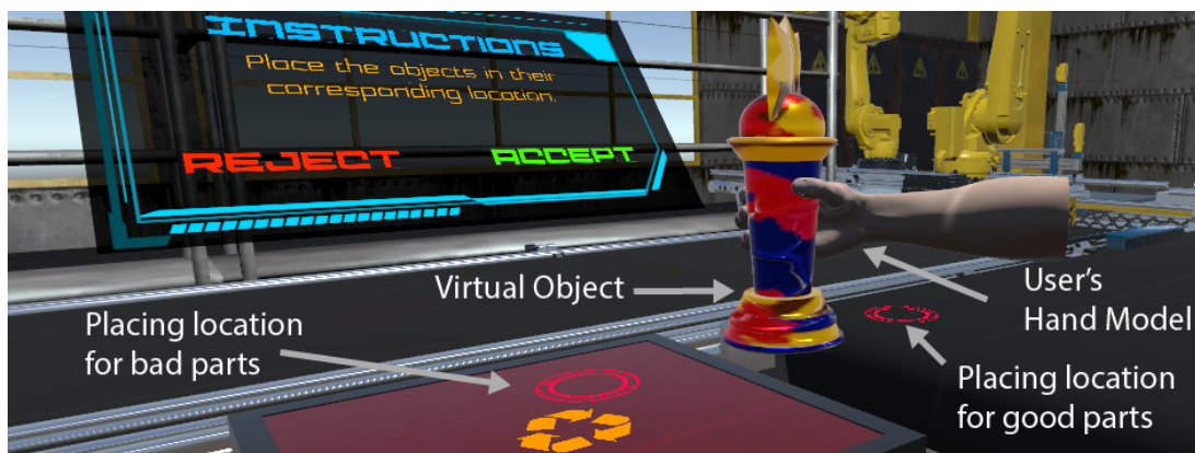
Figure 5.5 – Users face a table onto which a virtual part is extruded. They can pick it up and inspect it, then they select whether the part is flawed or good. This explicitly indicates their future to place the part either into the disposal bin or onto the conveyor belt. The robot drives to the chosen release position to preempt the user's release of the part, after which it removes the tangible object from the interaction space as the virtual part is either destroyed or removed from the scene.
