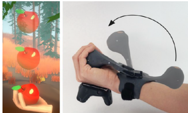
Figure 1.36 – Ungrounded wearable platform ETHD presented by Kovacs et al. [60]. This device was designed mainly for object manipulation.
