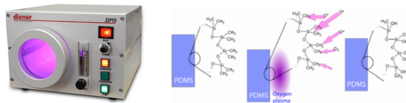
Figure C.1: Plasma cleaner A standard procedure with plasma cleaner(left) is used to increase adhesion potential through a process called surface activation.
