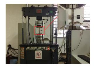
Fig. 3.5 MTS 809 servohydraulic testing machine system
