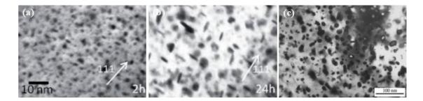
Fig. 2.2 TEM images of (a) GP zones at underaged state, (b)  $\eta$ ' phase at peak-aged state [51] and (c)  $\eta$  phase at overaged state [52].
