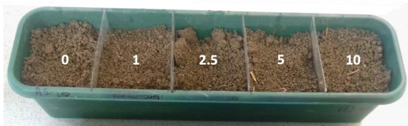
Figure 20: Linear gradient mesocosm (0.6 m x 0.13 m x 0.1 m) with nominal MA treatment ( \text{t ha}^{-1} ) used in the avoidance test.
