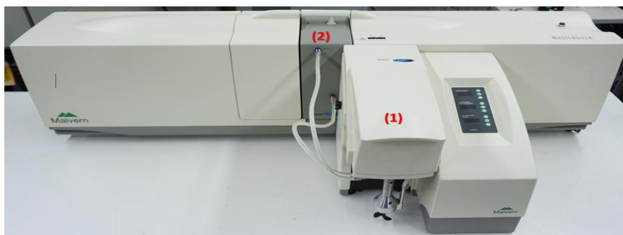
Figure 2. 1. Mastersizer 2000 apparatus. (1) Hydro 2000; (2) Optical bench
