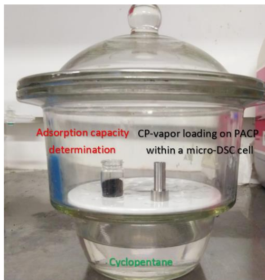
Figure C-1.1. Closed-vessel, partially filled with CP (adsorption chamber), used for adsorption capacity determination of the PACP and preparation of CP-saturated PACP for the hydrate formation experiments.
