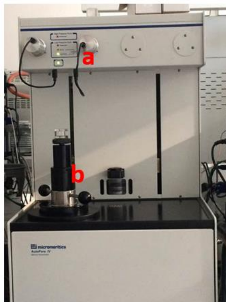
Figure 2. 6. Autopore IV 9500 instrument. a) low pressure port; b) high pressure port.
