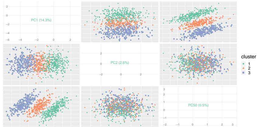
Figure 4.6: Subspaces found by PCA on a simulation with p = 50 , color and shape indicate the true cluster membership. Once again, the most discriminative subspace is given by the first and last components, the other corresponding to noisy directions.
