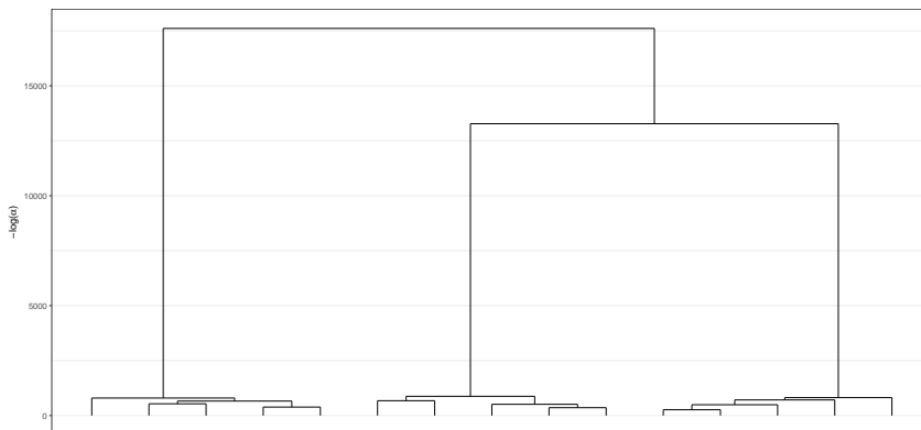
Figure 1.5: Dendrogram extracted by the hierarchical algorithm of Chapter 4 (see motivating example of Figure 5.1). The leaves are iteratively merged, the smaller height representing the first fusions. The y -axis quantifies the marginal cost of each fusion and the elbow heuristics would cut the tree at 3 clusters, which corresponds to the true hierarchical structure in this simulation.
