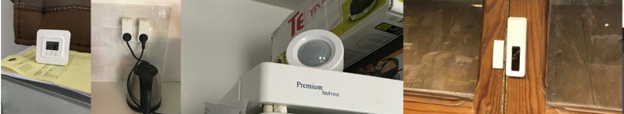
Figure 4.3 – The positioning of PIR sensors, power sensors, contact sensors and some of their images in Cestas site
