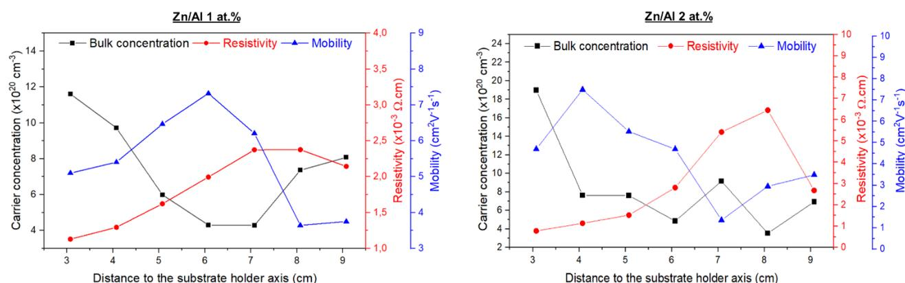
**Figure 70:** Hall effect measurements of the AZO films deposited from a Zn/Al target with 1 and 2 at.% of Al. They represent the variation of the carrier concentration ( $\text{cm}^{-3}$ ), the resistivity ( $\Omega \cdot \text{cm}$ ) and mobility ( $\text{cm}^2 \text{V}^{-1} \text{s}^{-1}$ ) as a function of the distance to the substrate holder axis (cm).
