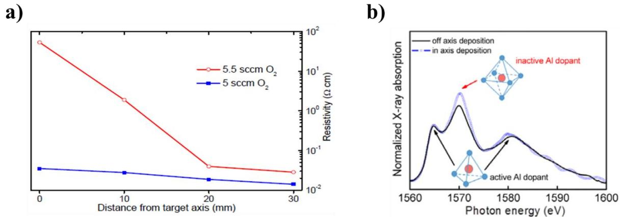
**Figure 9:** a) Resistivity ( $\Omega \cdot \text{cm}$ ) of AZO films deposited by reactive DCMS under 5 and 5.5 sccm flow of oxygen as a function of the distance to the target axis (mm) and b) Al-K edge XANES spectra of the AZO films deposited at 0 mm (facing the target axis) and 30 mm from the target axis [3].
