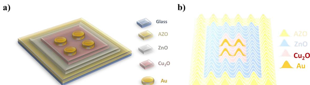
**Figure 36:** Scheme of the solar cell structure of the fourth solar cells series fabricated on two different substrates: **a)** Flat glass and **b)** Structured glass of  $p = 1.5 \mu\text{m}$  periodicity. Each solar cell was made twice with two different applied voltages of AZO, 545 and 550 V.
