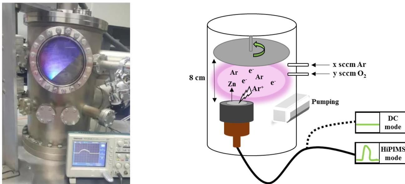
**Figure 24:** (Left) Picture of the PVD chamber used in this work during an AZO film HiPIMS deposition; and (Right) Schematic representation of the PVD chamber used for the AZO films deposition in this study, as well as a portrayal of the deposition parameters and conditions. The black cable represents the possibility to plug the magnetron to a DC or to a HiPIMS generator.
