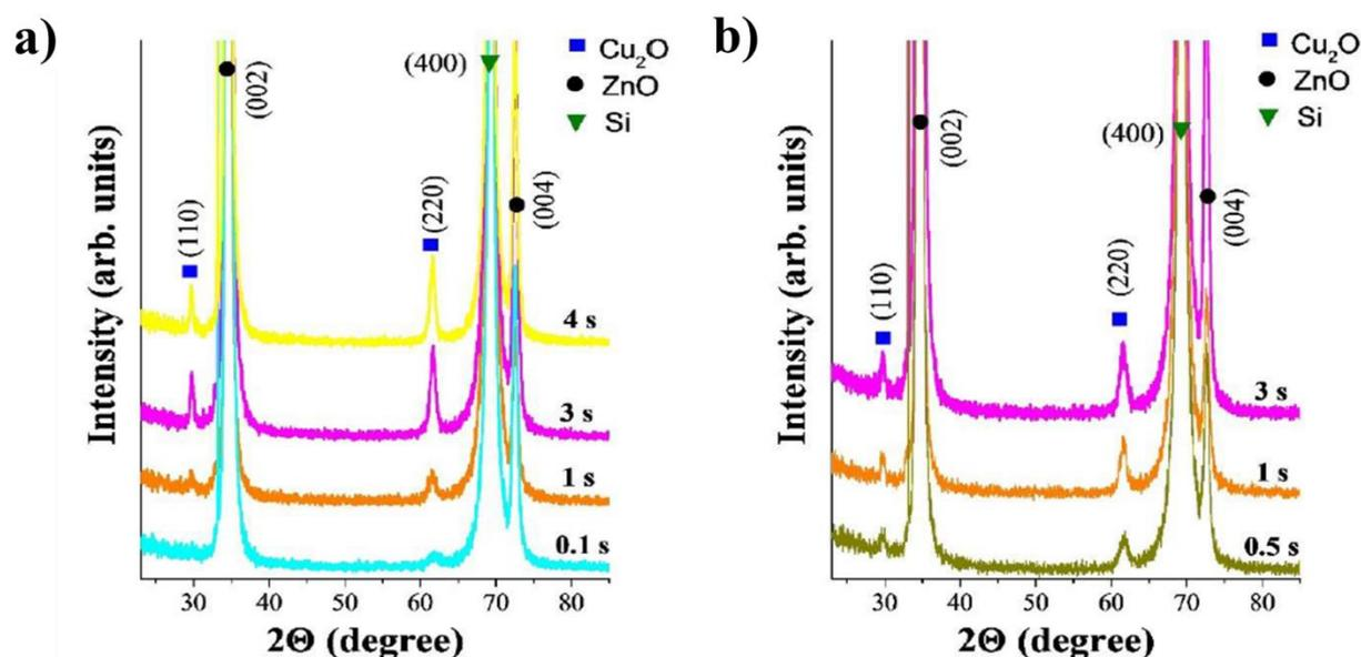
**Figure 28:** XRD diffractograms of a  $\text{Cu}_2\text{O}$  film deposited on ZnO when **a)** the  $\text{Cu}(\text{hfac})_2$  pulse is kept constant at 3 s while the  $\text{H}_2\text{O}$  pulse is varied from 0,1 to 4 s and when **b)** the  $\text{H}_2\text{O}$  pulse is kept constant at 3 s while the  $\text{Cu}(\text{hfac})_2$  pulse is varied from 0,5 to 3 s [14].
