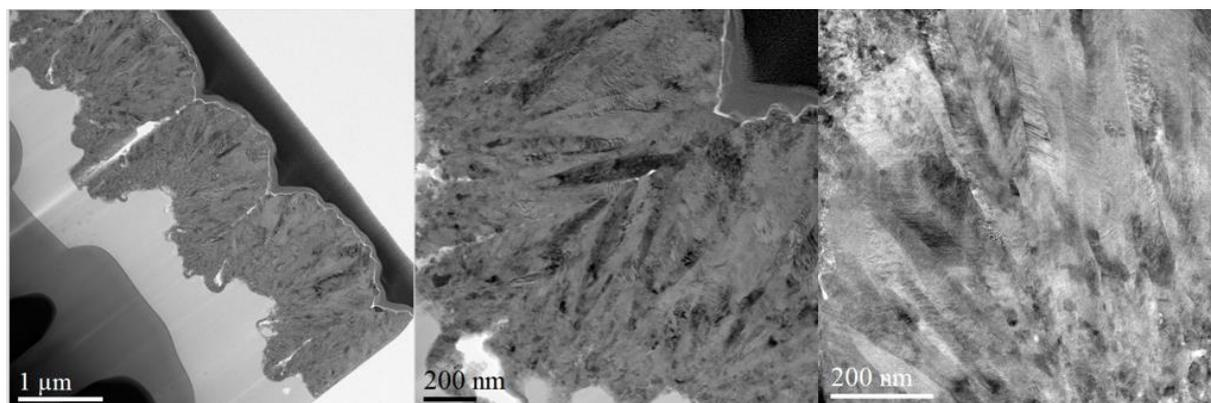
**Figure 91:** TEM images of the Structured glass 1.5 $\mu\text{m}$ /AZO 1 at. %/ZnO/Cu<sub>2</sub>O sample.
