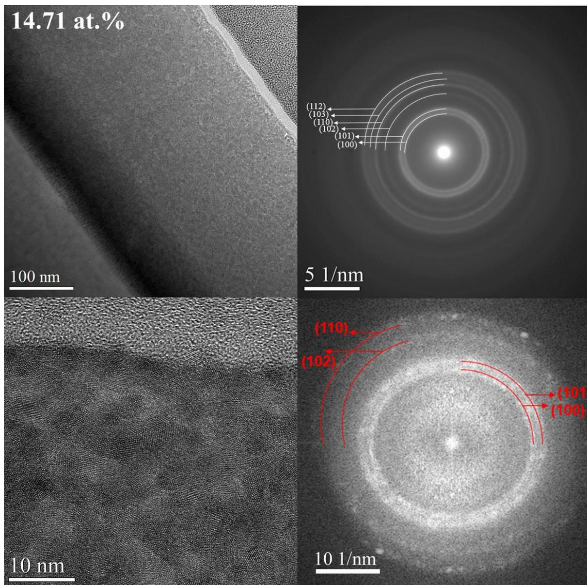
**Figure 62:** Panels of the main results obtained by TEM measurements including a TEM image, a SAED, a HR-TEM image and its indexed FFT for the AZO film containing 14.71 at.% of Al deposited from a Zn/Al 15 at.% target with the indicated content representing the measured Al concentration (at.%) in the AZO films *in-axis*. ZA stands for Zone Axis.
