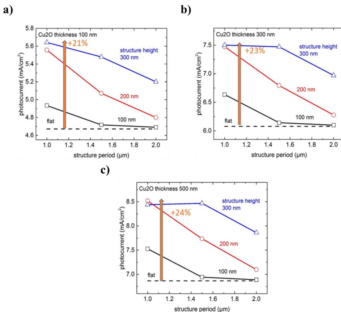
**Figure 83:** Photocurrent (mA/cm<sup>2</sup>) as a function of structure period (μm) for Cu<sub>2</sub>O layer thicknesses of **a)** 100, **b)** 300 and **c)** 500 nm. In each graph, the case of a flat cell and a structured cell with 100, 200 and 300 nm structure height are considered. The arrows represent the maximum relative photocurrent increase.
