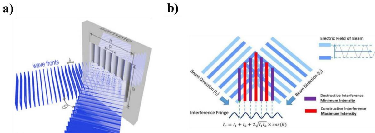
**Figure 31:** Schematic representation of **a**) the interference of two laser beams separated by an angle  $\theta$  on a ( $axa$ ) sample to form a structure with a  $p$  periodicity; and **b**) the laser interference of two beams on a surface showing the constructive and destructive interferences at maximum and minimum intensities respectively, responsible for the structure creation [153,154].
