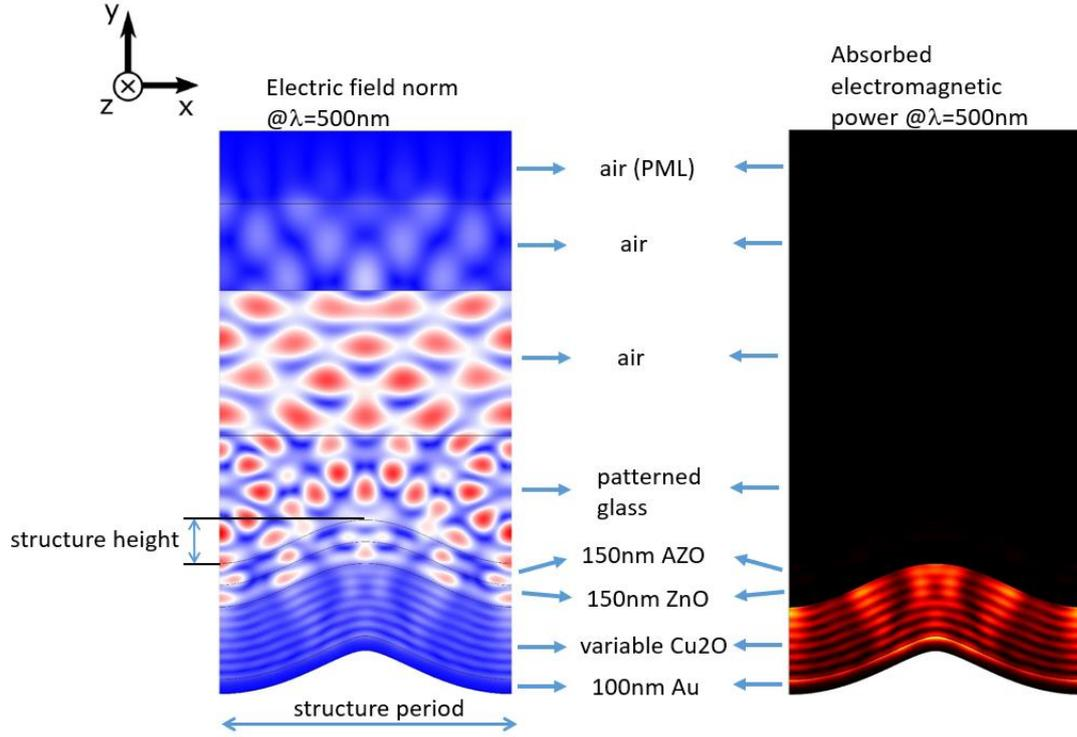
**Figure 34:** Simulation of the electric field norm (**Left**) and the absorbed electromagnetic power (**Right**) at 500 nm wavelength for a solar cell comprised of a patterned glass substrate with a specific structure height and period, a 150 nm AZO layer, a 150 nm ZnO layer, a Cu<sub>2</sub>O with variable thickness and a 100 nm gold (Au) layer [1].
