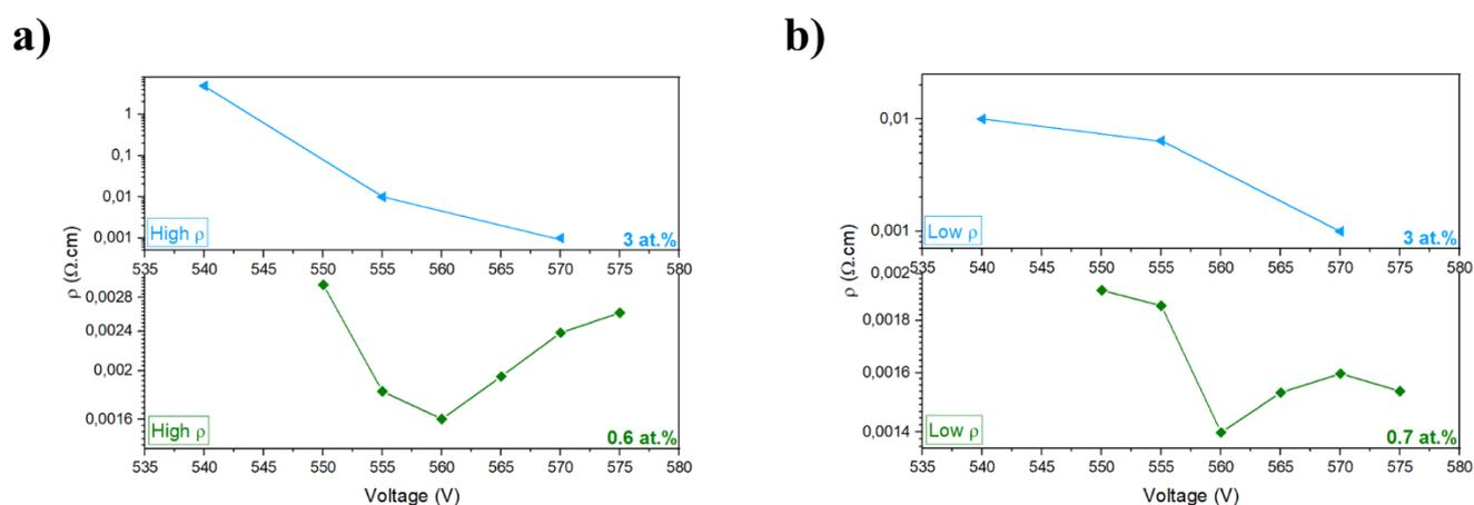
**Figure 75:** Graphs of the resistivity as a function of the applied voltage for AZO films deposited from a new Zn/Al target with 3 at.% of Al [52] and a used Zn/Al target with 1 at.% of Al in the **a)** *high*  $\rho$  and **b)** *low*  $\rho$  positions. **Changer % 1% ?**
