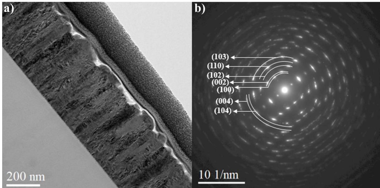
**Figure 89:** a) TEM image of the Glass/ZnO/Cu<sub>2</sub>O sample and b) SAED image of the ZnO layer of the sample.
