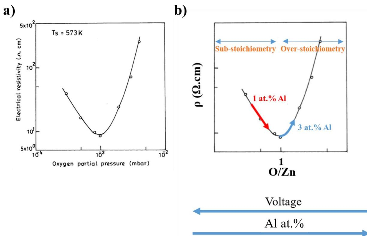
**Figure 76:** a) Graph representing the electrical resistivity as a function of the oxygen partial pressure  $P_{\text{O}_2}$  at a substrate temperature of 573 K of a ZnO film deposited by DC magnetron sputtering extracted from [182] and b) An adaptation of the previous graph to correspond to our results with the  $x$  axis replaced by the O/Zn value to represent the film’s stoichiometry.
