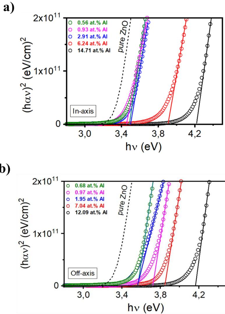
**Figure 66:** Energy band gap graphs of the AZO films deposited from a 0.56/0.68 at.% of Al deposited from a Zn/Al 1 at.% target, 0.93/0.97 at.% of Al deposited from a Zn/Al 2 at.% target, 2.91/1.95 at.% of Al deposited from a Zn/Al 5 at.% target, 6.24/7.04 at.% of Al deposited from a Zn/Al 10 at.% target and 14.71/12.09 at.% of Al deposited from a Zn/Al 15 at.% target with the at.% values representing the real Al at.% in the AZO films in the **a)** *in-axis* and **b)** *off-axis* positions.
