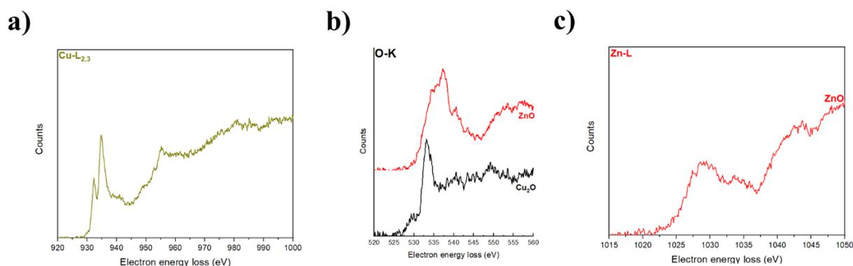
**Figure A9:** ELNES spectra from the glass/ZnO/Cu<sub>2</sub>O sample of the a) Cu-L<sub>2,3</sub> edge of the Cu<sub>2</sub>O layer, b) O-K edge of the Cu<sub>2</sub>O and ZnO layers and c) Zn-L edge of the ZnO layer.
