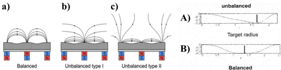
**Figure 18:** On the left, a representation of the racetrack for all three types of magnetron: **a)** Balanced, **b)** Unbalanced type 1 and **c)** Unbalanced type II [108]. On the right, the target erosion profile for **A)** an unbalanced and **B)** an balanced magnetron [109].
