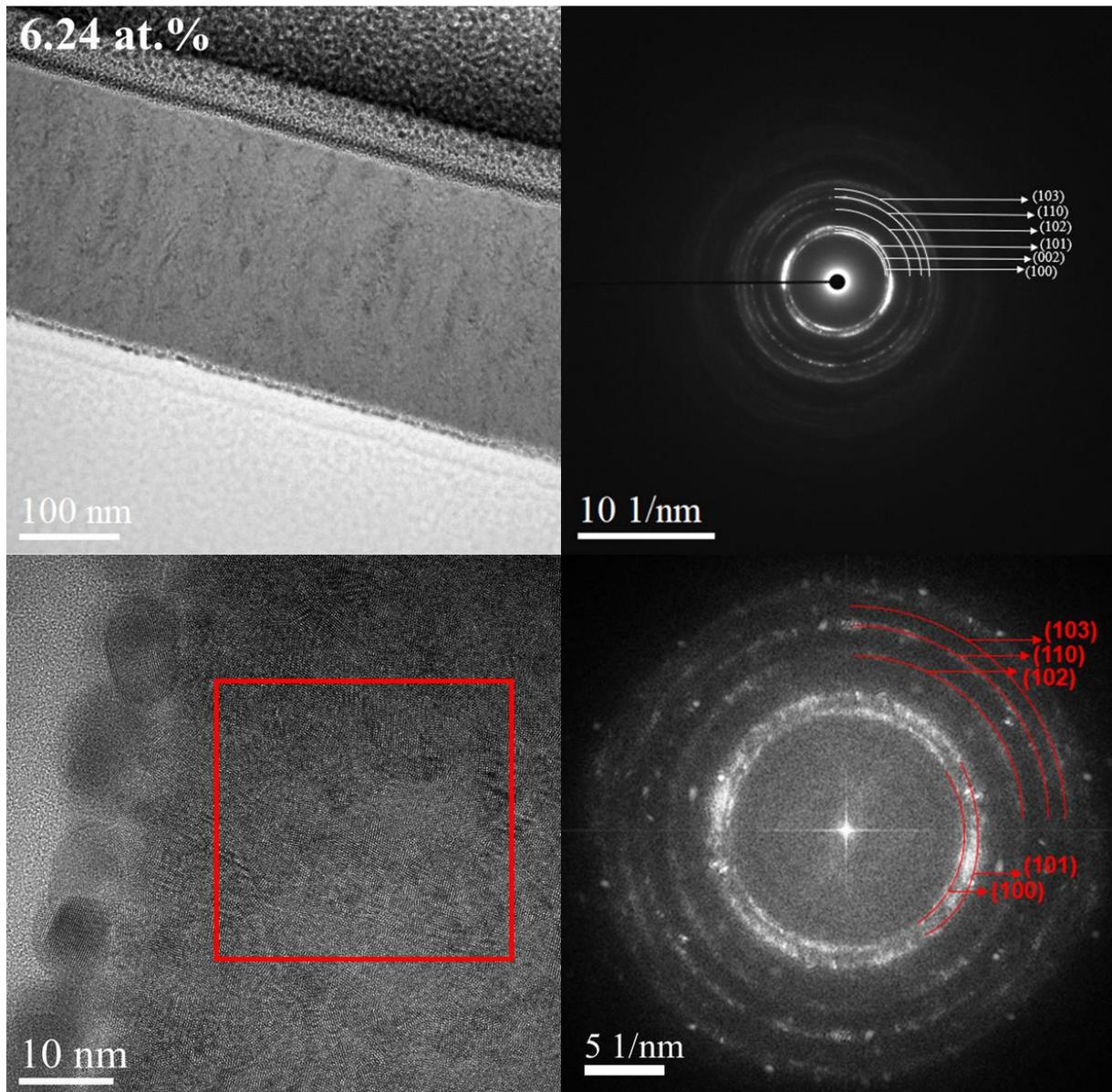
**Figure 61:** Panels of the main results obtained by TEM measurements including a TEM image, a SAED, a HR-TEM image and its indexed FFT for the AZO film containing 6.24 of Al deposited from a Zn/Al 10 at.% target with the indicated content representing the measured Al concentration (at.%) in the AZO films *in-axis*. ZA stands for Zone Axis.
