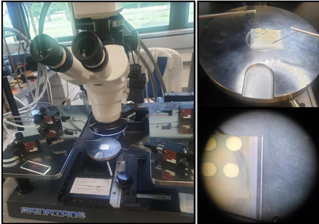
**Figure 50:** Photos taken at the LMOPS laboratory showing **a)** the equipment used to perform the I-V measurements on a solar cell and **b,c)** a zoom-in on the process where one probe is placed on the AZO back-contact layer (light yellow) and the other on the Au front-contact layer (gold dots).
