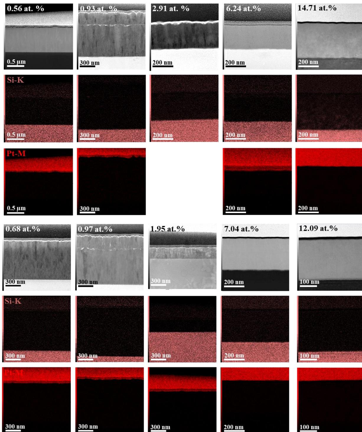
**Figure A1:** STEM images in the *in-axis* (Top image) and *off-axis* (Bottom image) positions of the AZO films deposited from a Zn/Al target with 1, 2, 5, 10 and 15 at.% of Al respectively and their corresponding EDS mapping of the Si (Gold rose) and Pt (red) compositions.
