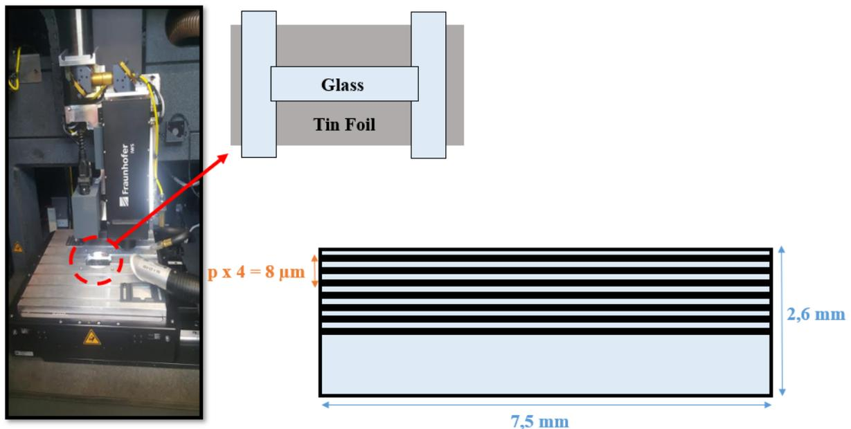
**Figure 33:** Photographic image of the experimental setup, and a scheme showing the to be structured sample position and the structure geometry on a glass slide.
