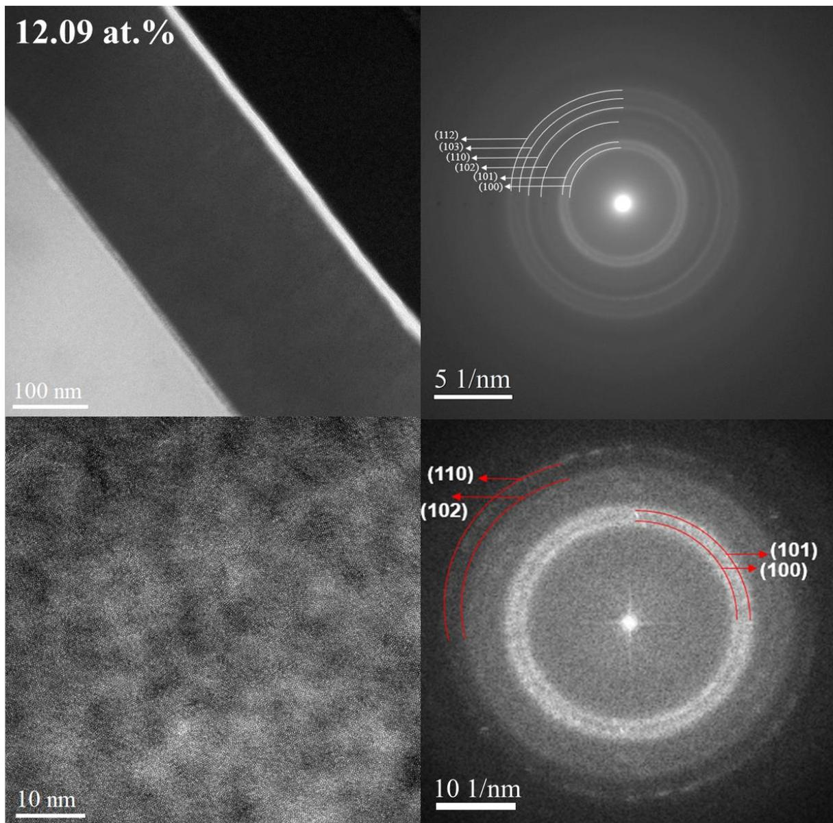
**Figure A3:** Panels of the main results obtained by TEM measurements including a TEM image, a SAED, a HR-TEM image and its indexed FFT for the AZO film containing 12.09 at.% of Al deposited from a Zn/Al 15 at.% target with the at.% values representing the real Al at.% in the AZO films *off-axis* position.
