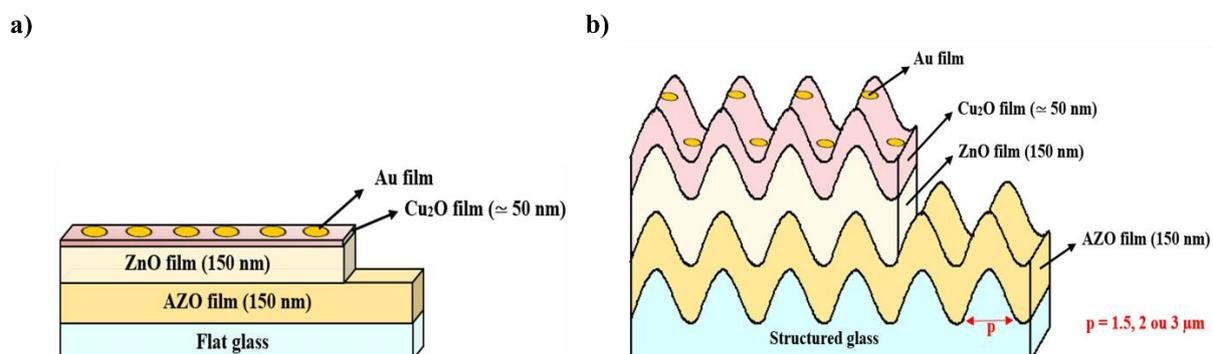
**Figure 35:** Scheme of the solar cell structure of the third solar cells series fabricated on four different substrates : a) Flat glass and b) Structured glass of three different periodicities  $p = 1.5, 2$  and  $3 \mu\text{m}$ .
