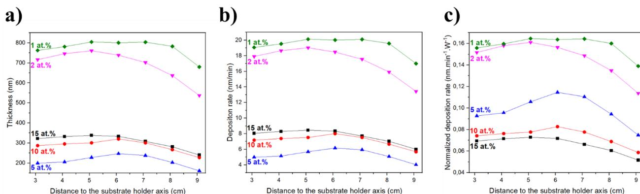
**Figure 52:** **a)** Thickness (nm), **b)** Deposition rate (nm/min) and **c)** Normalized deposition rate ( $\text{nm}\cdot\text{min}^{-1}\cdot\text{W}^{-1}$ ) as a function of the distance to the substrate holder axis (cm) for the AZO films obtained from the Zn/Al targets with 1, 2, 5, 10 and 15 at.% of Al respectively.
