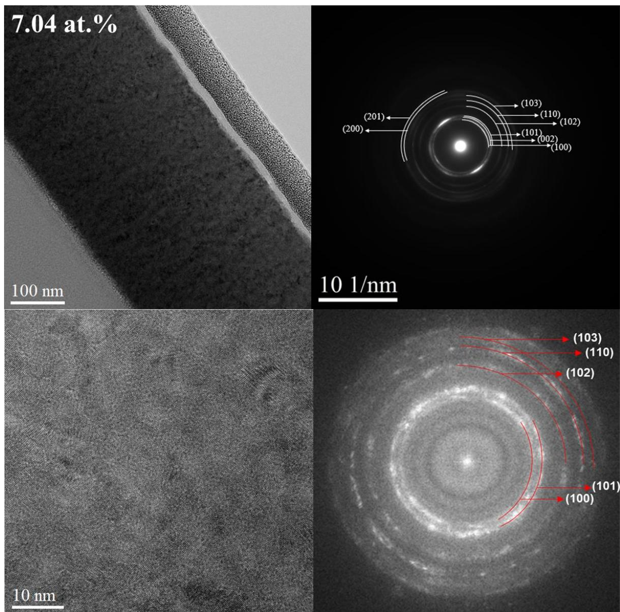
**Figure A2:** Panels of the main results obtained by TEM measurements including a TEM image, a SAED, a HR-TEM image and its indexed FFT for the AZO film containing 7.04 at.% of Al deposited from a Zn/Al 10 at.% target with the at.% values representing the real Al at.% in the AZO films *off-axis* position.
