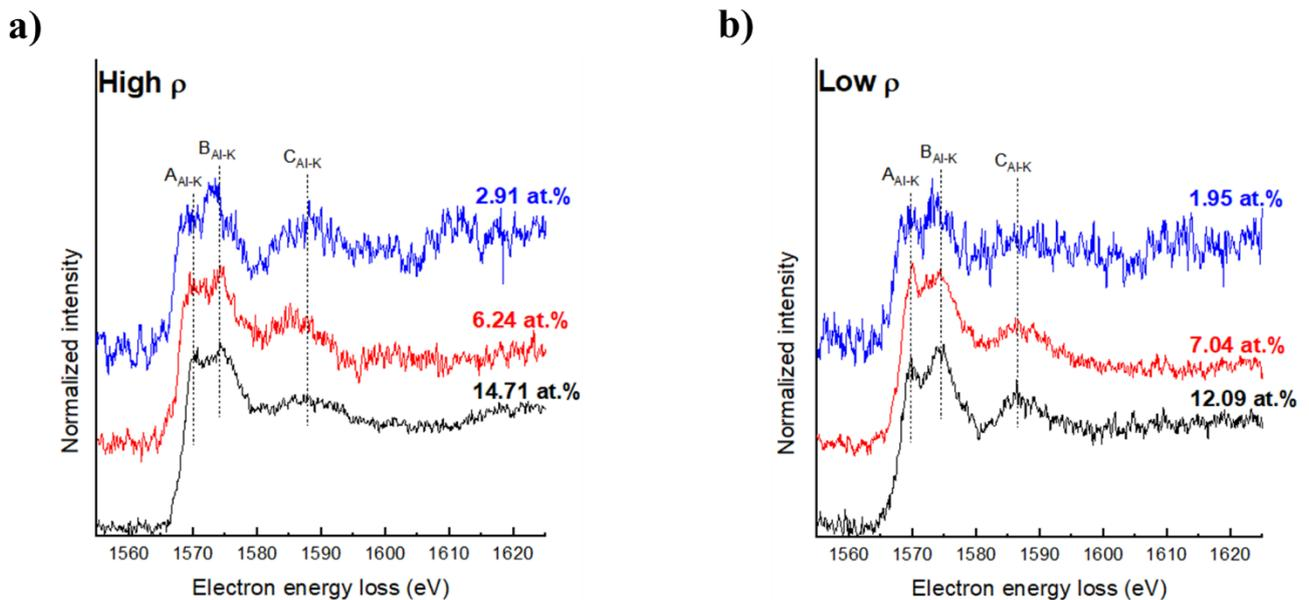
**Figure 79:** Al-K electron energy loss near edge structure at the **a)** *high ρ* and **b)** *low ρ* positions of the AZO films with 2.91/1.95 at.% of Al deposited from a Zn/Al 5 at.% target, 6.24/7.04 at.% of Al deposited from a Zn/Al 10 at.% target and 14.71/12.09 at.% of Al deposited from a Zn/Al 15 at.% target with the at.% values representing the real Al at.% in the AZO films *high ρ/low ρ* positions.
