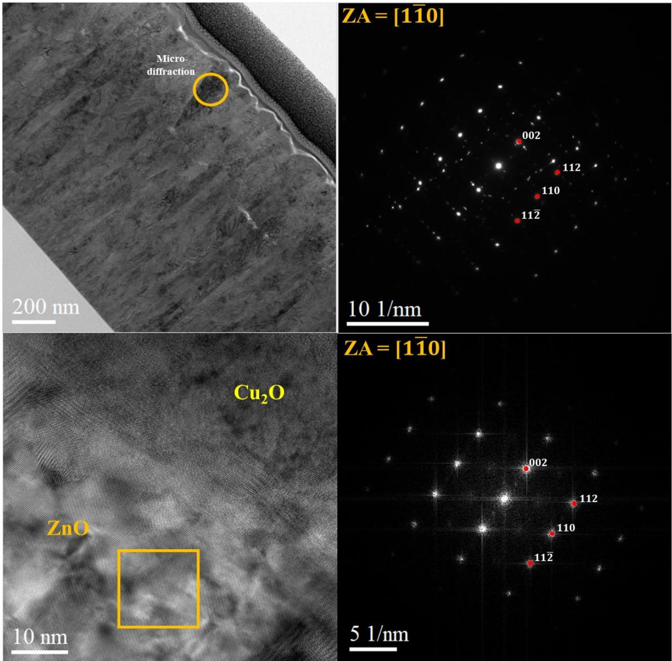
**Figure 90:** a) (Left) TEM image of the Glass/AZO1at.%/ZnO/Cu<sub>2</sub>O sample and (Right) the micro-diffraction image of the orange area shown on the ZnO layer; b) (Left) HR-TEM image at the ZnO/Cu<sub>2</sub>O heterojunction and (Right) the corresponding FFT image of the orange area shown on the ZnO layer.
