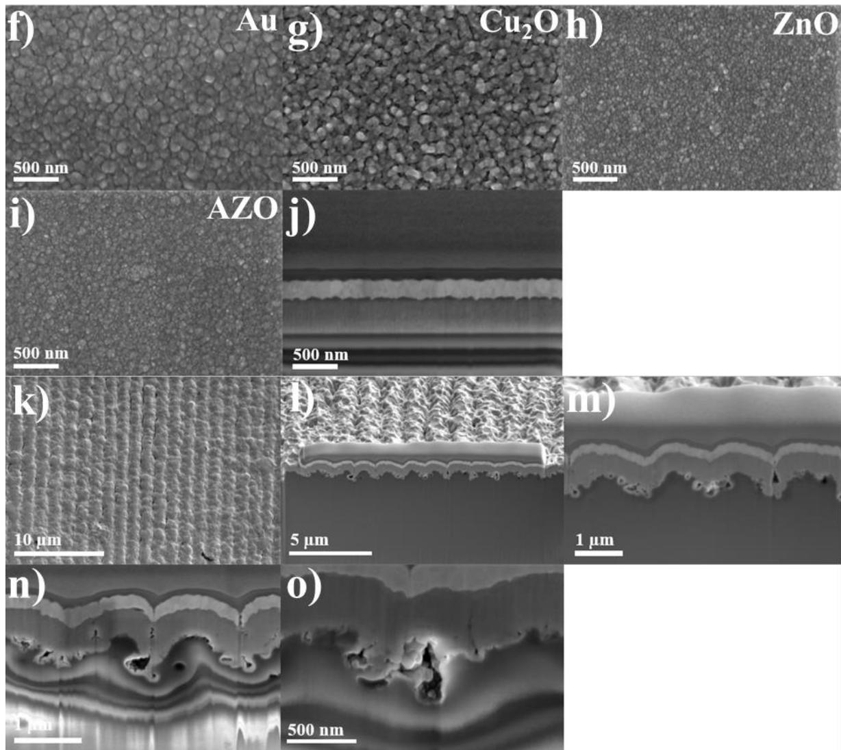
**Figure 95:** Top view SEM images and cross-sections of the **a)** Glass/AZO2at.%/ZnO/Cu<sub>2</sub>O/Au (3-A); **b) to e)** Structuredglass1.5μm/AZO2at.%/ZnO/Cu<sub>2</sub>O/Au (3-B); **f) to j)** Glass/AZO2at.%/ZnO/Cu<sub>2</sub>O/Au (4-A) and **k) to o)** Structuredglass1.5μm/AZO2at.%/ZnO/Cu<sub>2</sub>O/Au (4-B).
