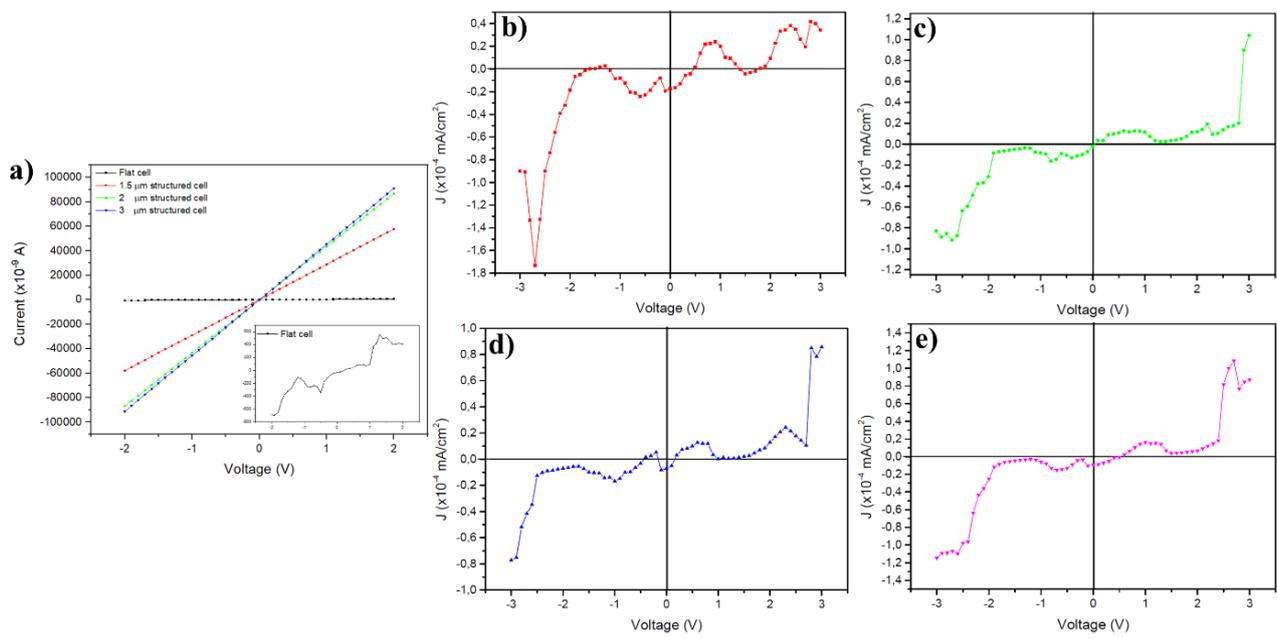
**Figure 98:** a) Current as a function of voltage for the AZO layer in all the samples of the third series solar cells; I-V measurements of the solar cells on b) flat glass, c) 1.5 μm, d) 2 μm and e) 3 μm structured glass.
