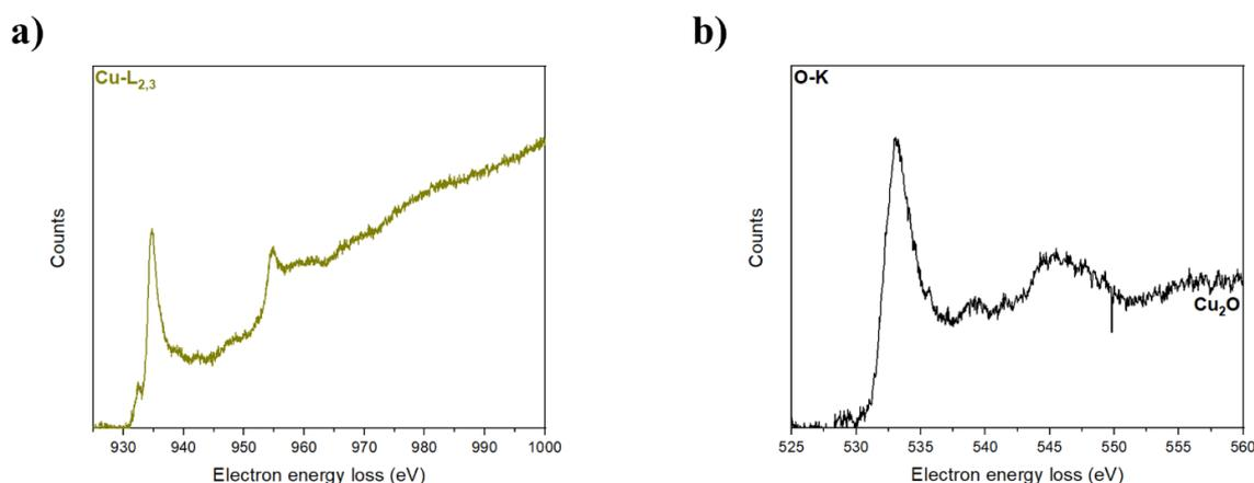
**Figure A10:** ELNES spectra from the Si-2cm/ZnO/Cu<sub>2</sub>O sample of the a) Cu-L<sub>2,3</sub> edge and b) O-K edge of the Cu<sub>2</sub>O layer.
