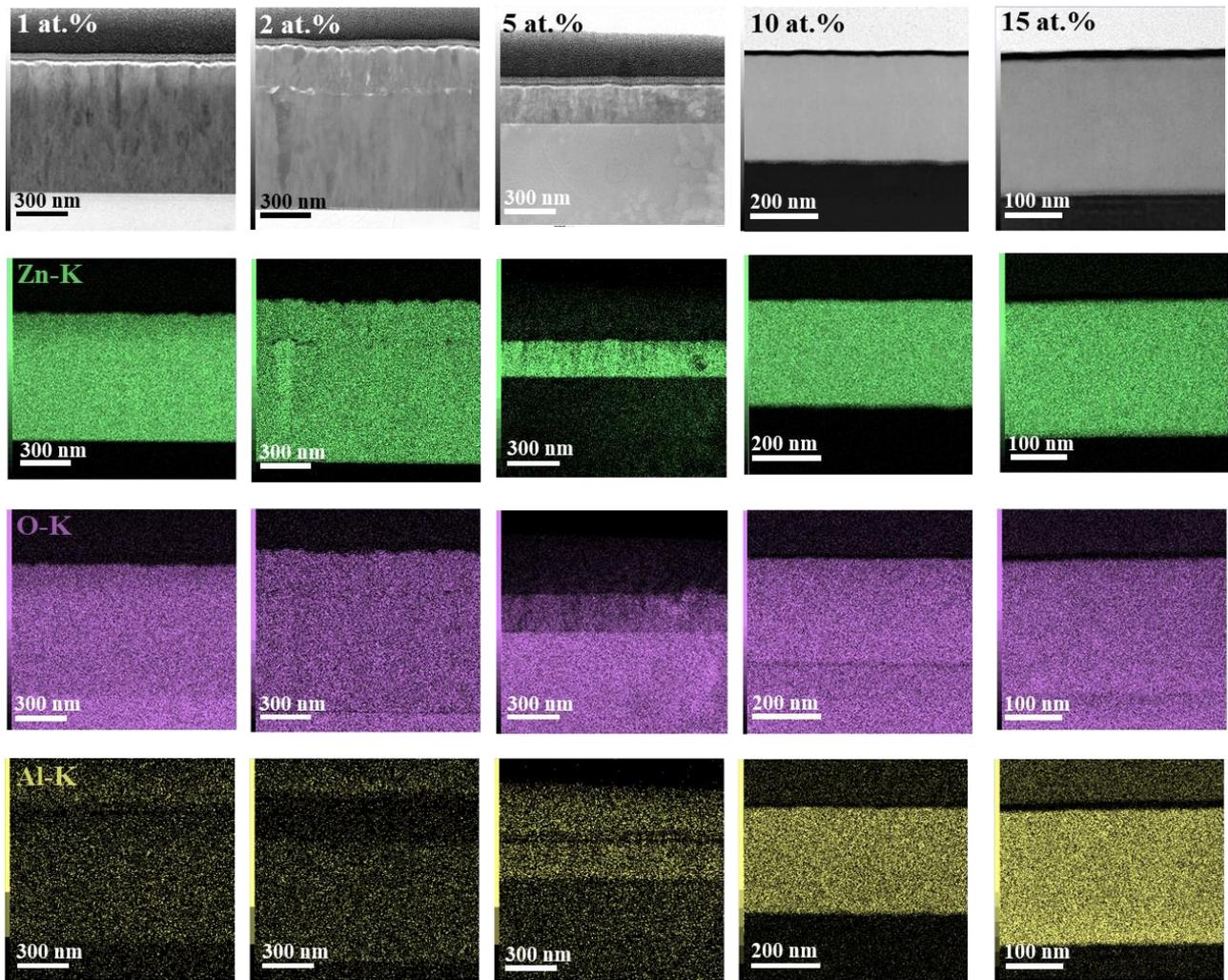
**Figure 53:** STEM images in the *in-axis* (Top) and *off-axis* (Bottom) positions of the AZO films deposited from a Zn/Al target with 1, 2, 5, 10 and 15 at.% of Al respectively and their corresponding EDS mapping of the Zn (green), O (purple) and Al (yellow) compositions.
