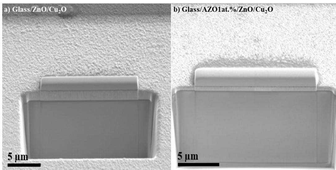
**Figure 87:** Top and cross-section SEM images taken with a FIB microscope of **a)** Glass/ZnO/Cu<sub>2</sub>O (1-A) and **b)** Glass/AZO 1 at.%/ZnO/Cu<sub>2</sub>O (1-B).
