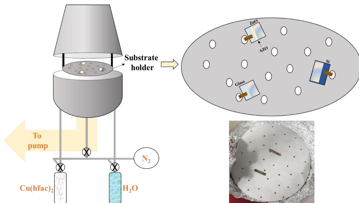
**Figure 27:** Schematic illustration of the ALD chamber showing the precursor Cu(hfac)<sub>2</sub>, reactant H<sub>2</sub>O and carrier gas N<sub>2</sub> tanks as well as an image and details of the substrate holder.
