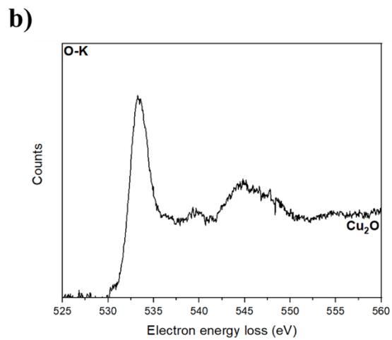
**Figure A11:** ELNES spectra from the Si-8cm/ZnO/Cu<sub>2</sub>O sample of the **a)** Cu-L<sub>2,3</sub> edge and **b)** O-K edge of the Cu<sub>2</sub>O layer.
