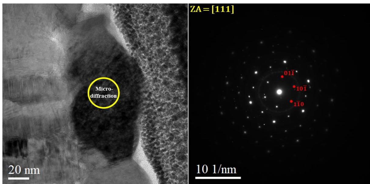
**Figure A8:** (Left) HR-TEM image of the Si-8cm/ZnO/Cu<sub>2</sub>O sample and (Right) the associated micro-diffraction of the Cu<sub>2</sub>O film (yellow).
