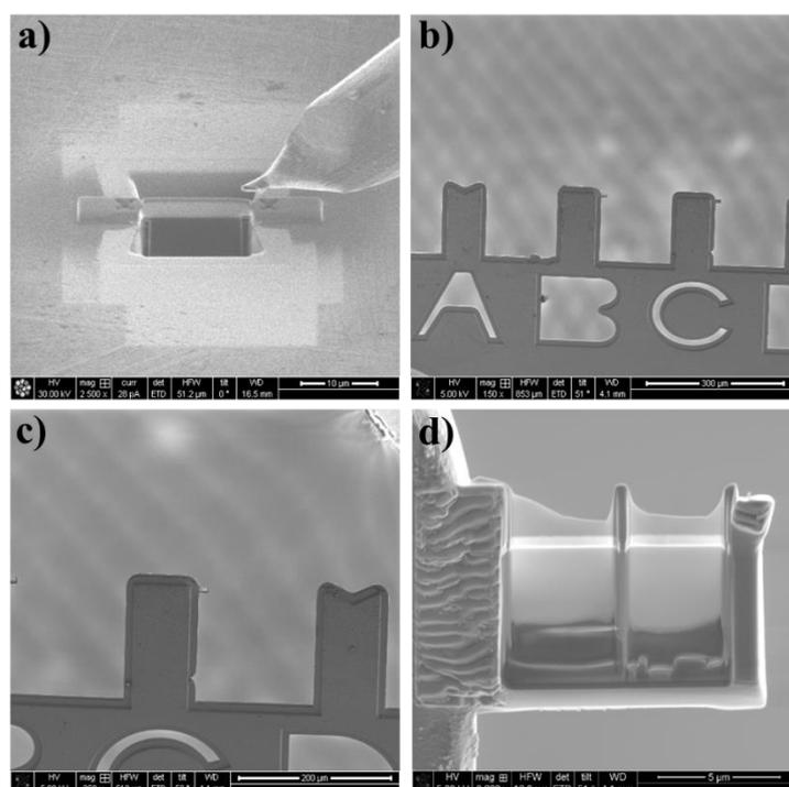
**Figure 45:** FIB images showing **a)** the transfer probe getting ready to lift the thinned sample lamella, **b)** and **c)** the FIB lamella fixed onto a copper grid and **d)** an example of a FIB lamella taken from an AZO film deposited from a Zn/Al 2 at.% target.
