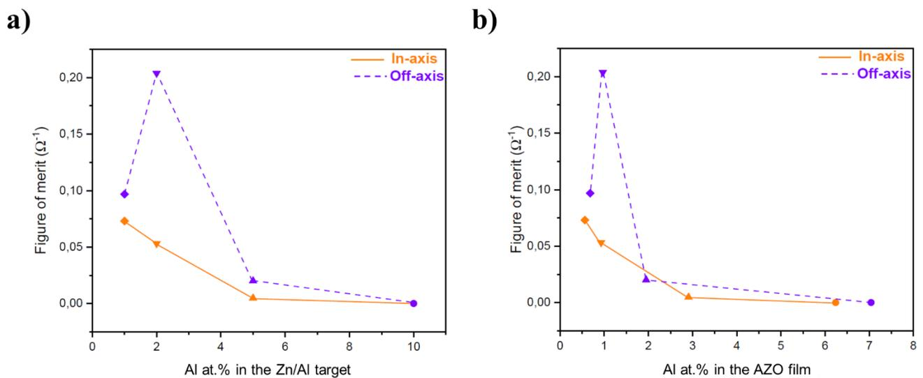
**Figure 71:** Graph of the figure of merit ( $\Omega^{-1}$ ), in the *in-axis* and *off-axis* positions, as a function of **a)** the Al content (at.%) present in the Zn/Al targets used for the deposition of the AZO films and **b)** the actual Al content present in the AZO films.
