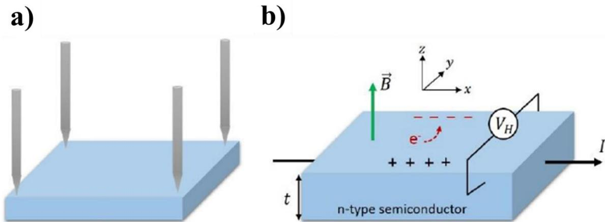
**Figure 40:** Schematic representation of a) The Van der Pauw contact configuration method used in the Hall effect measurement and b) the process that occurs during a Hall effect measurement of a thin film [14].
