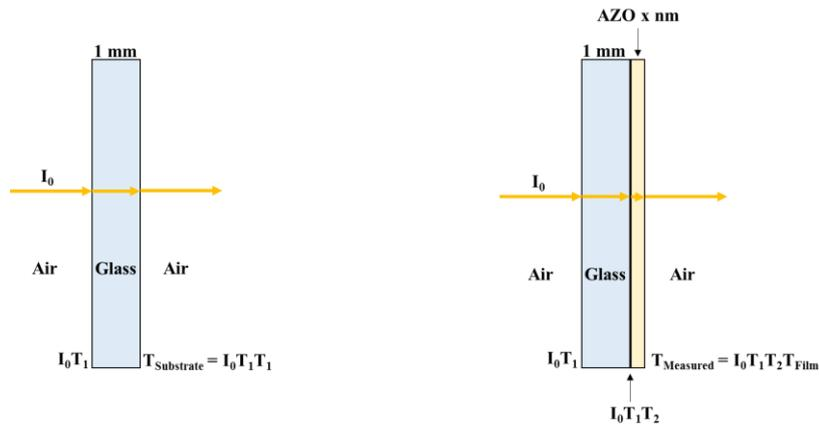
**Figure 41:** Schematic representation of light passing through (Left) a simple glass substrate and (Right) an AZO film deposited on a glass substrate. One must note that the beam intensity decreases gradually for each light penetrated layer or material.
