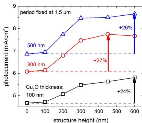
**Figure 85:** Photocurrent (mA/cm<sup>2</sup>) as a function of structure height (nm) for Cu<sub>2</sub>O layer thicknesses of 100, 300 and 500 nm. The structure period was fixed at 1.5 μm and the arrows represent the maximum relative photocurrent increase.
