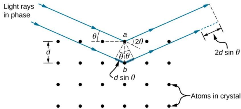
**Figure 44:** Schematic representation of X-ray diffraction from a crystal sample [167].
