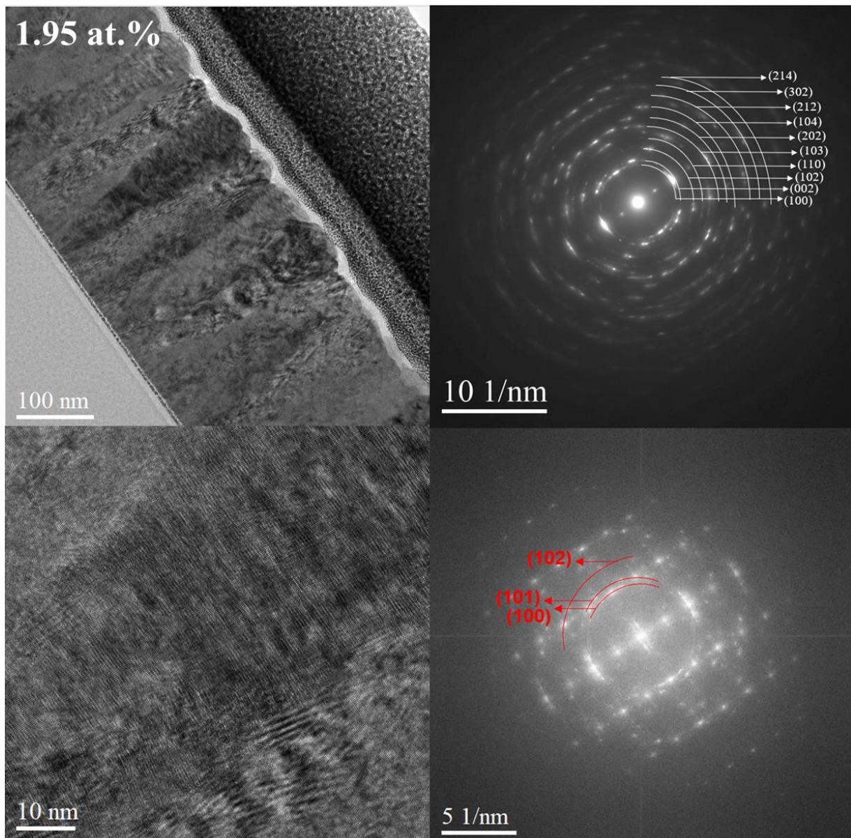
**Figure 60:** Panels of the main results obtained by TEM measurements including a TEM image, a SAED, a HR-TEM image and its indexed FFT for the AZO film containing 2.91/1.95 at.% of Al deposited from a Zn/Al 5 at.% target with the indicated content representing the measured Al concentration (at.%) in the AZO films *in-axis/off-axis* positions. ZA stands for Zone Axis.
