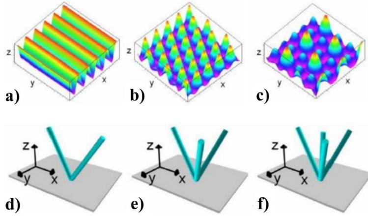
**Figure 32:** Representation of the calculated intensity distribution and the corresponding beam configurations for **a,d)** two-beam, **b,e)** three-beam and **c,f)** four-beam laser interference [156].
