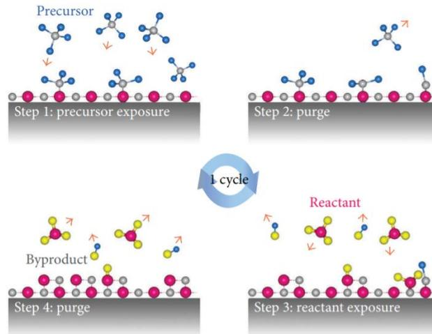
**Figure 26:** Schematic illustration of the ALD process [139].
