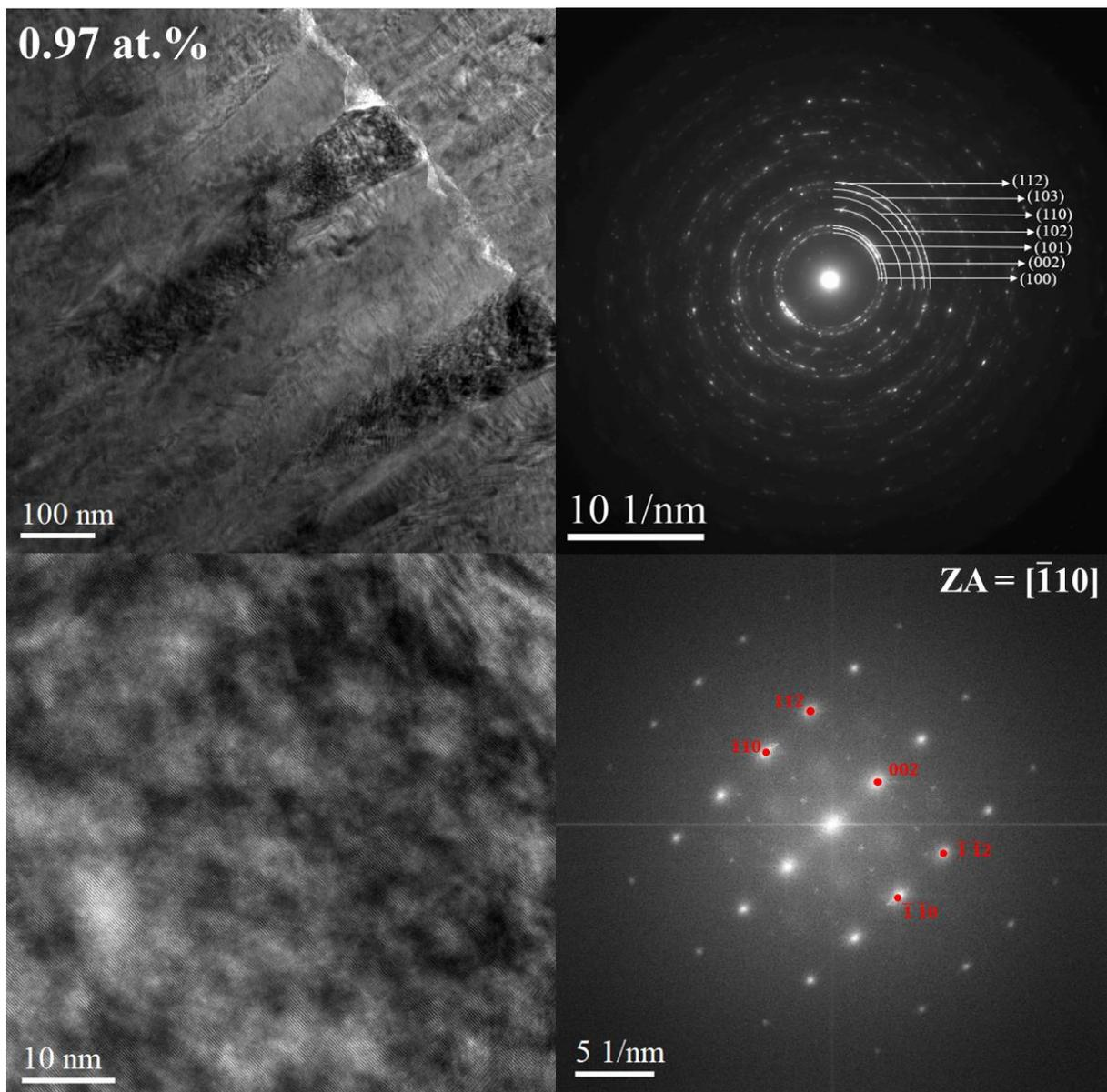
**Figure 59:** Panels of the main results obtained by TEM measurements including a TEM image, a SAED, a HR-TEM image and its indexed FFT for the AZO film containing 0.93/0.97 at.% of Al deposited from a Zn/Al 2 at.% target with the indicated content representing the measured Al concentration (at.%) in the AZO films *in-axis/off-axis* positions. ZA stands for Zone Axis.
