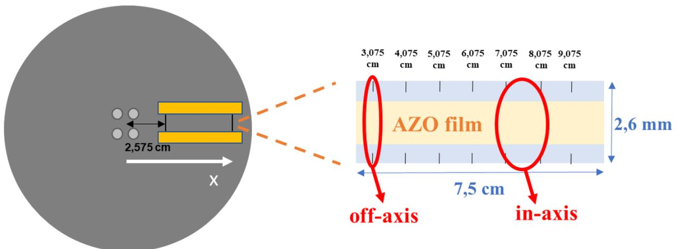
**Figure 25:** Schematic representation of the substrate-holder and the glass slide substrate positioned at 2.575 cm from the center of the substrate holder. The enlarged image shows in detail the 7 different positions on which all the characterisations were performed, as well as a highlight of the *in-axis* and *off-axis* positions.
