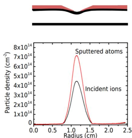
**Figure 69:** Graph showing the particle density on the target of the incident ions (black curve) and the sputtered atoms (red curve) as a function of the position from the target center for  $Y = 1.6$  atoms/ion. The top illustration shows schematically the racetrack position on the target as well as the oxide layer in red. The surface atom density is 10.9, 6.8, 5.9, 5.2 for (001), (110), (100) and (101) ZnO planes, respectively [52].
