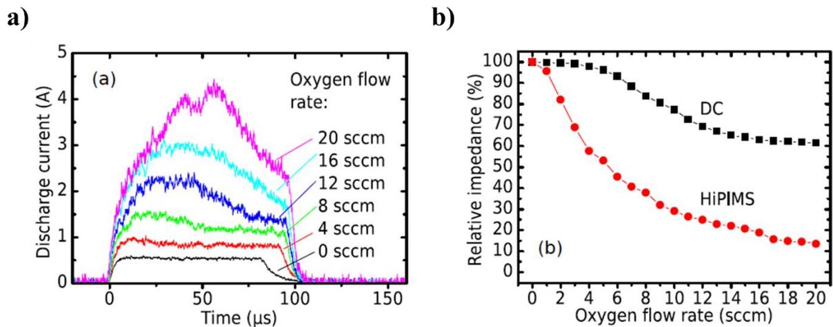
**Figure 22:** a) Discharge current waveforms of AZO films deposited by HiPIMS sputtering under a constant applied voltage of 570 V, for different oxygen flow rates; and b) Graph of the normalized relative impedance as a function of the oxygen flow rate for AZO films deposited by sputtering in a DC (black) or in a HiPIMS (red) regime. The graphs were extracted from [supplementary material of ref. 52].
