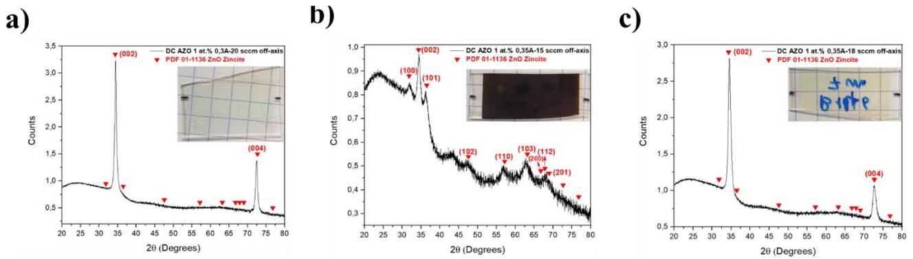
**Figure A4:** XRD diffractogram of AZO films deposited from a Zn/Al target with 1 at.% of Al at the *off-axis* position by DC sputtering at different applied currents and oxygen flow rates. The inset represents the photograph of the corresponding film.
