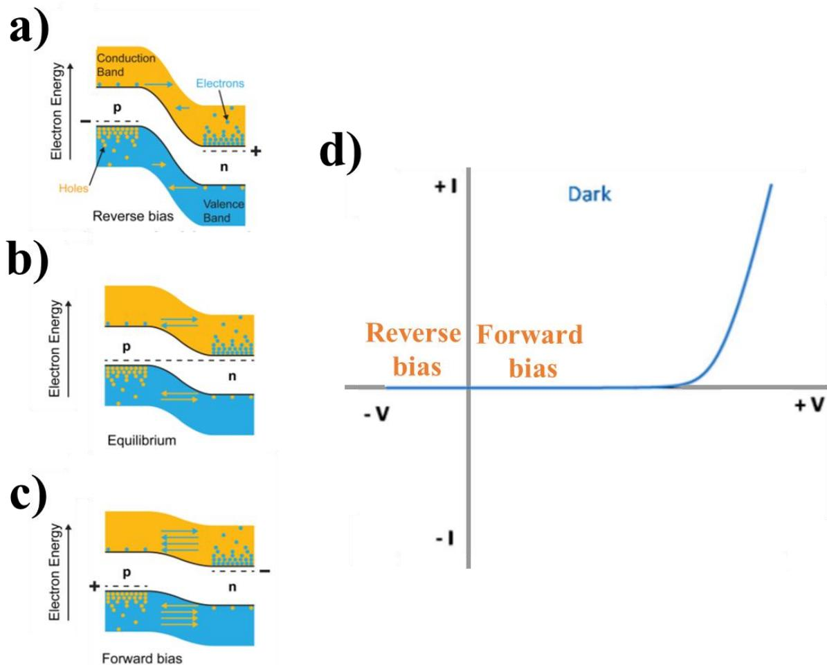
**Figure 15:** Representation of the energy band diagram of a p-n junction in dark mode during **a)** reverse bias, **b)** equilibrium and **c)** forward bias with **d)** being the corresponding I-V curve for the reverse and forward biases [Adapted from 90 and 98].
