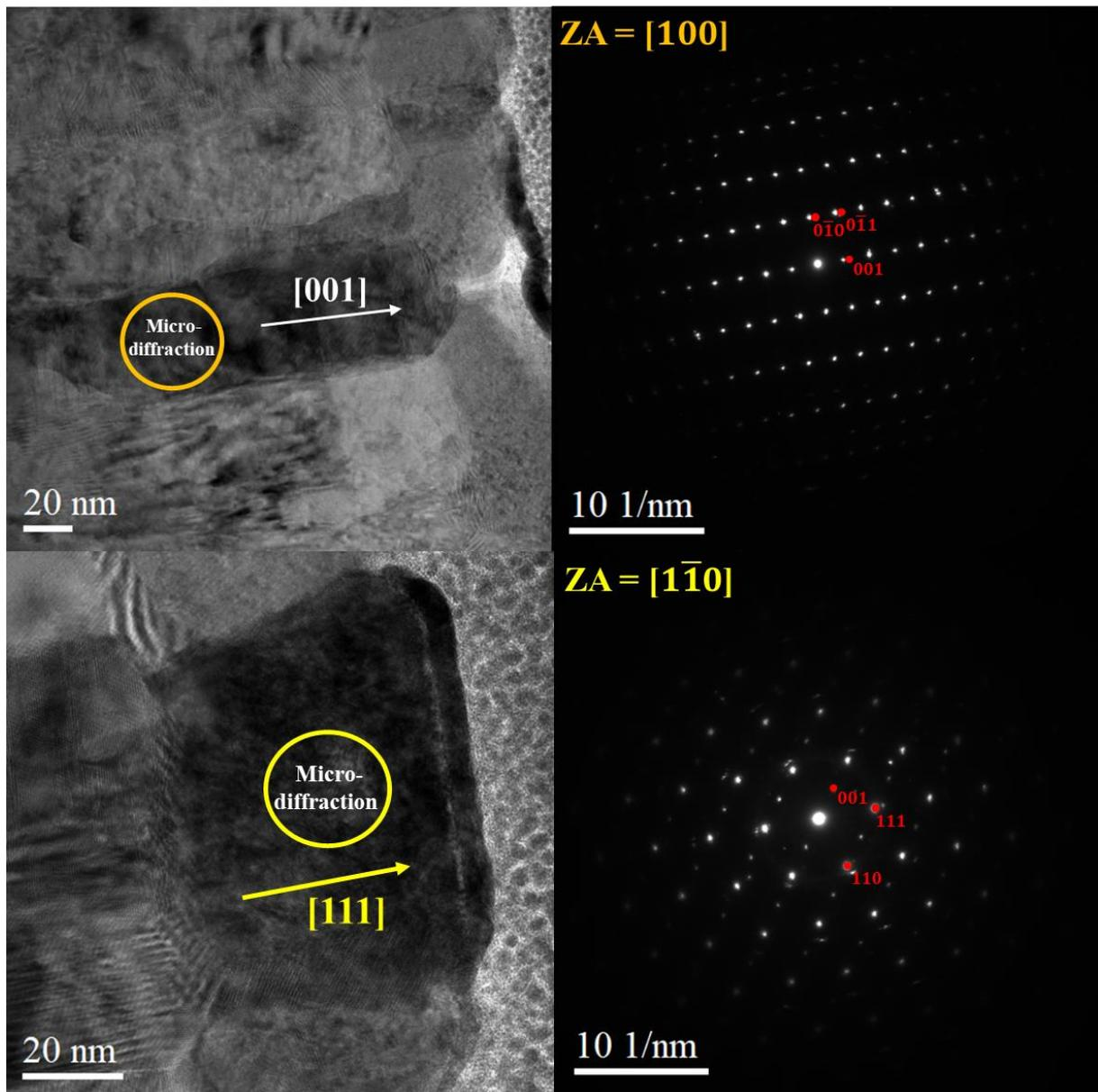
**Figure A7:** (Left) HR-TEM image of the Si-2cm/ZnO/Cu<sub>2</sub>O sample and (Right) the associated micro-diffraction of the ZnO film (orange) and Cu<sub>2</sub>O film (yellow).
