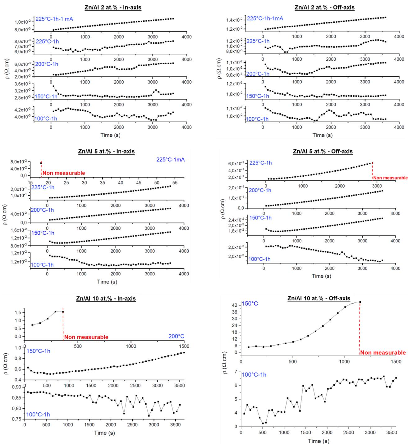
**Figure 72:** Resistivity evolution as a function of time of the AZO films deposited from Zn/Al targets with 1, 2, 5, 10 and 15 at.% of Al, at the *in-axis* and *off-axis* positions, during heat treatment in air at 100, 150, 200 and 225 °C for 1 hour at each temperature under 1  $\mu$ A of applied current. For the AZO films deposited from 1 and 2 at.% Al targets, one extra treatment at 225 °C for 1 hour was done under 1 mA of applied current.
