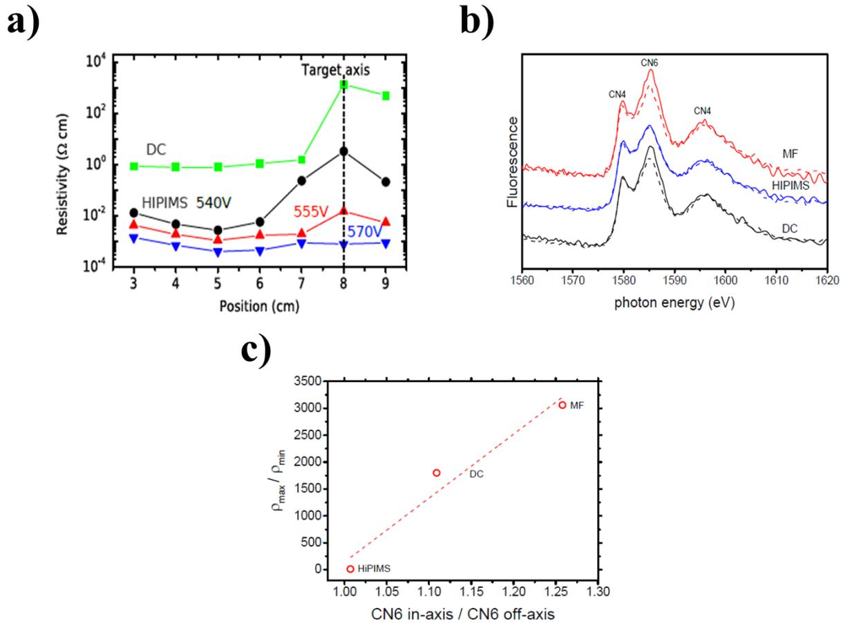
**Figure 10:** a) Resistivity of AZO films deposited by DC and HiPIMS at different applied voltages as a function of the position (cm) [52], b) Al-K edge XANES spectra of the AZO films deposited at 0 mm (solid lines) and 30 mm (dashed lines) from the target axis by reactive DC, MF and HiPIMS [3] and c) Graph of the intensity ratio of maximum (30 mm) to minimum (0 mm) resistivity as a function of the intensity ratio of aluminum (Coordination Number 6) CN6 at 0 mm to CN6 at 30 mm [3].
