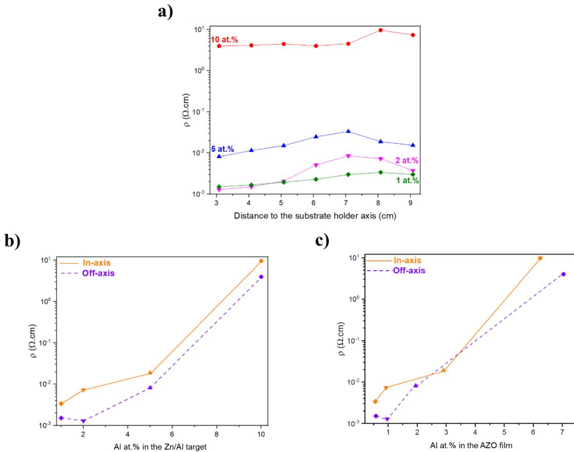
**Figure 68:** Graph of **a)** the resistivity  $\rho$  ( $\Omega\cdot\text{cm}$ ) as a function of the distance to the substrate holder axis (cm) for the AZO films deposited from Zn/Al targets with 1, 2, 5 and 10 at.% of Al. The AZO film deposited from a Zn/Al target with 15 at.% of Al was not presented because the resistivity was too high to be measured; and
