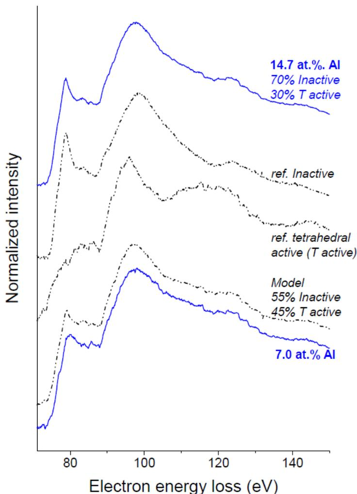
**Figure 81:** Al-L<sub>2,3</sub> edges reference spectra for electrically inactive and active Al serving as a basis to extract the proportions of inactive and active Al.
