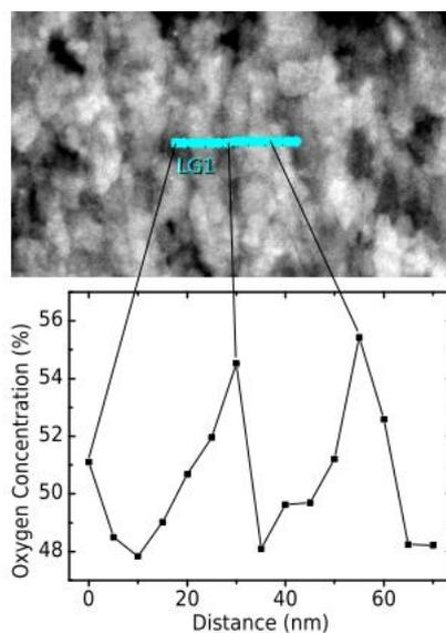
**Figure 55:** Image extracted from [52] representing a TEM image and its corresponding oxygen concentration profile measured by EDS for an AZO film deposited by HiPIMS at 8 cm from the substrate holder axis.
