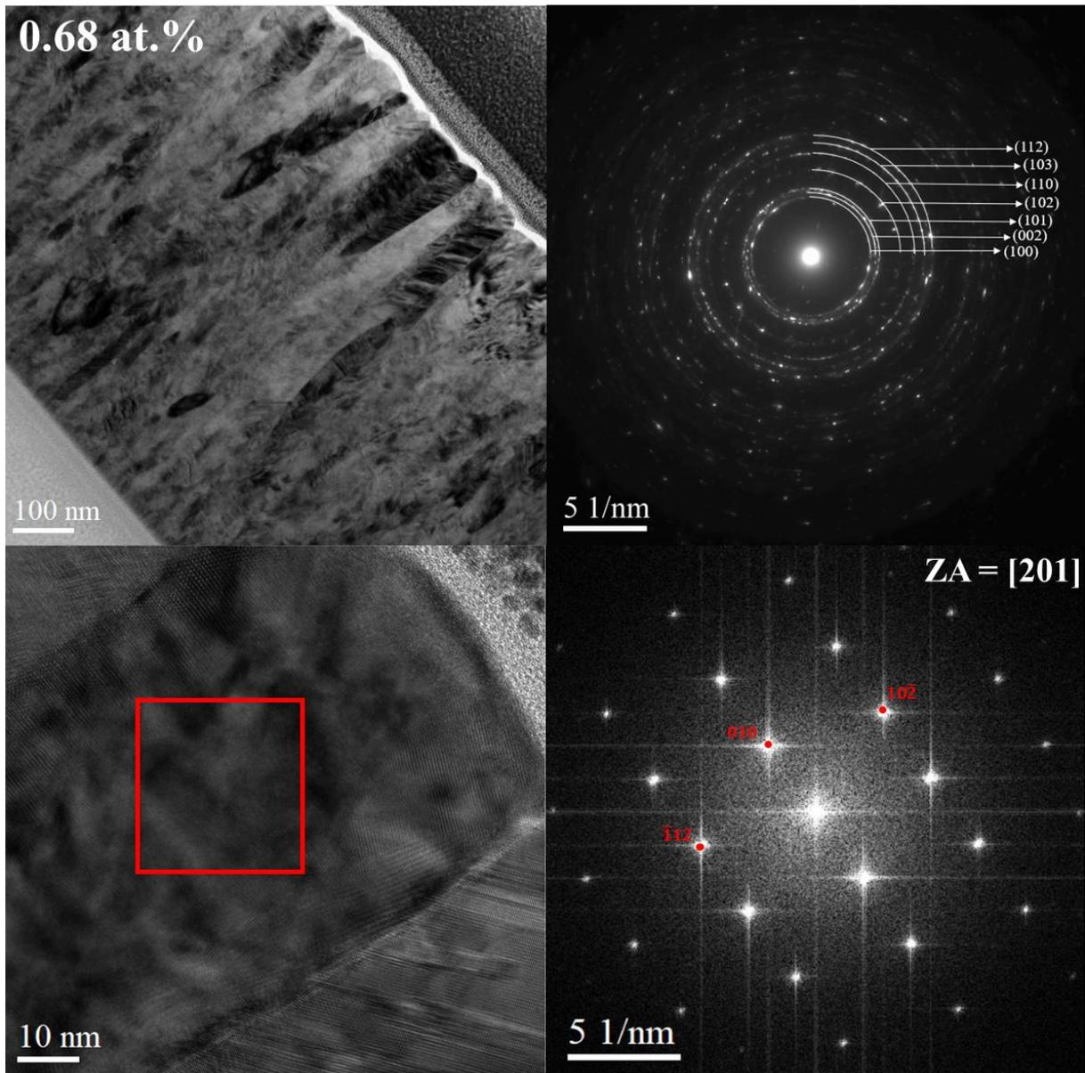
**Figure 58:** Panels of the main results obtained by TEM measurements including a TEM image, a SAED, a HR-TEM image and its indexed FFT for the AZO film containing 0.56/0.68 at.% of Al deposited from a Zn/Al 1 at.% Al target with the indicated concentration representing the measured Al content (at.%) in the AZO films *in-axis/off-axis* positions. ZA stands for Zone Axis.
