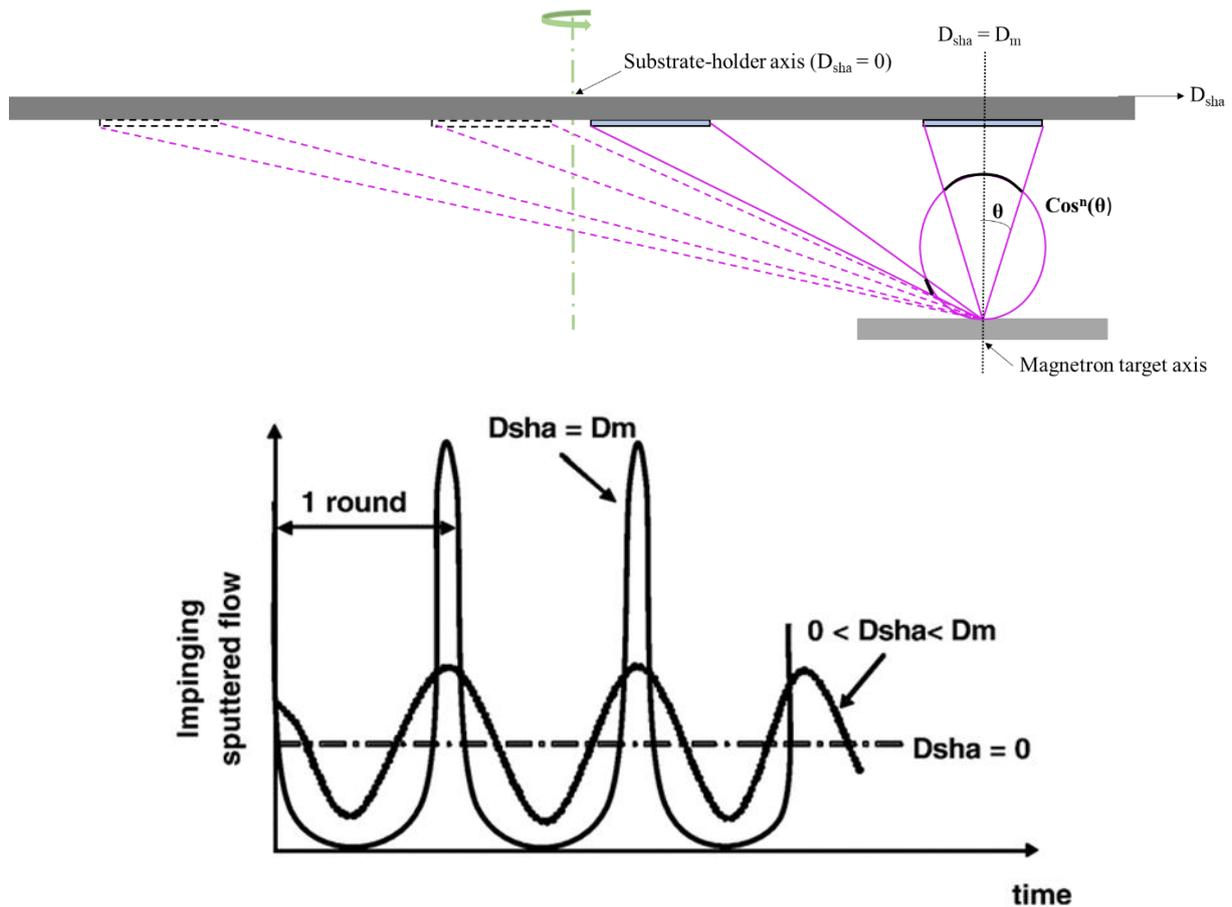
**Figure 21:** (Top) Illustration of the sputtering flux propagation from a target surface towards a rotatable substrate-holder holding a glass sample; and (Bottom) Graphic demonstration of the impinging sputtered flow as a function of time for the different possible positions of the sample in reference to the magnetron axis [118].
