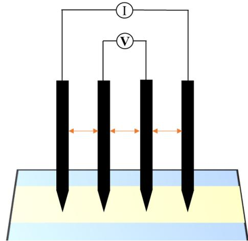
**Figure 38:** Schematic representation of **a)** the four point probe setup while measuring the resistance of an AZO film (yellow) deposited on glass (blue) and **b)** A close up on the equidistant four probes showing the applied current wiring on the outer probes and the measured voltage drop wiring on the inner probes.
