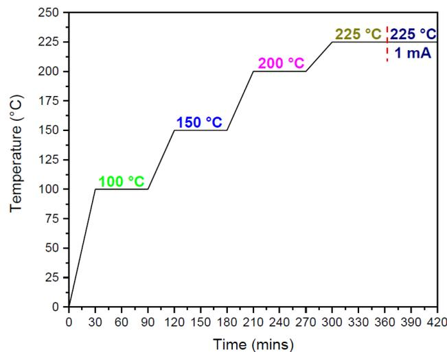
**Figure 39:** Graphical representation of the temperature (°C) as a function of time (mins) showing the heating process of the AZO films in order to study the influence of temperature on their electrical properties.
