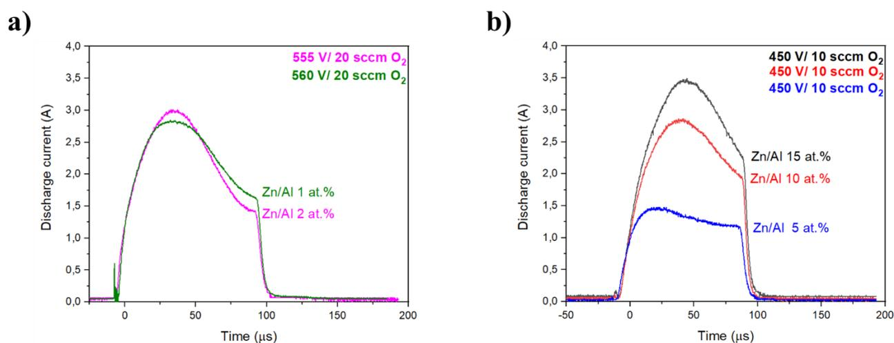
**Figure 51:** Discharge current waveforms for the AZO films deposited by HiPIMS from five Zn/Al targets: **a)** Zn/Al 1 and 2 at.% Al and **b)** Zn/Al 5, 10 and 15 at.% Al. The applied voltage and the flow of O<sub>2</sub> gas used for each film are mentioned in the top right corner of the graphs.
