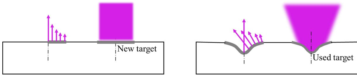
**Figure 23:** Illustration of the sputtering flux emerging from a **(Left)** new target compared to **(Right)** a used one. Dotted dashed lines represent the radius of the racetrack and arrows represent the sputtered flux.
