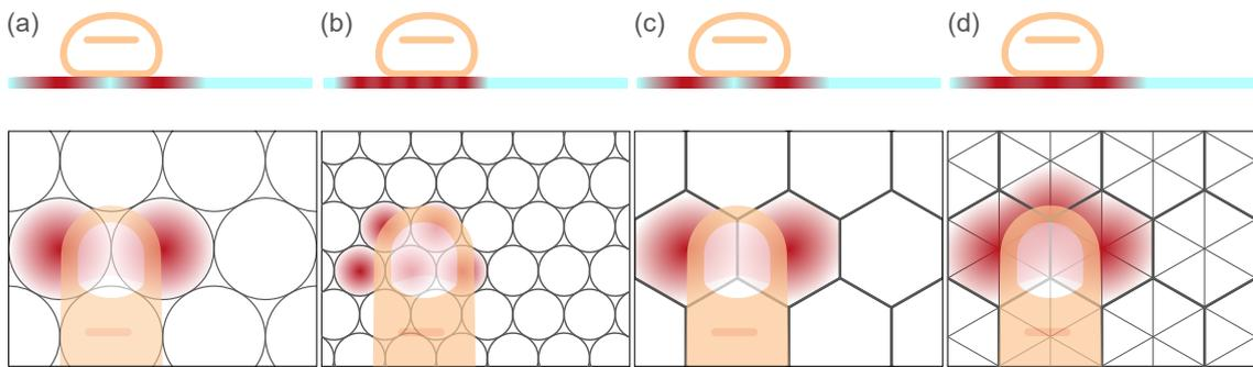
Figure 5.4: Piezoelectric distribution. a) Circular pattern. b) High density circular pattern. c) Hexagon pattern. d) Triangular pattern.
