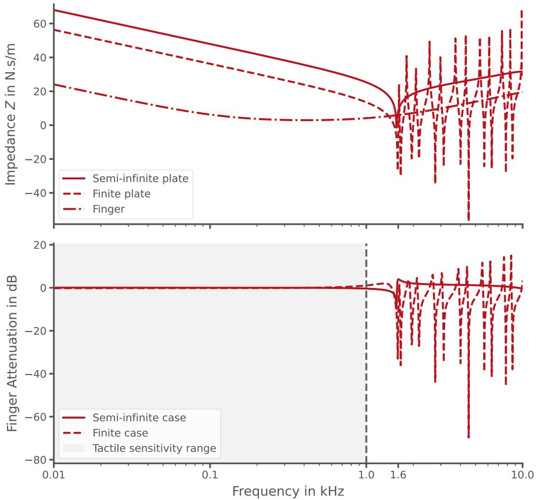
Figure 3.12: Theoretical attenuation curve  $\mu_{dB} = 20 \log_{10} |\mu|$  for semi-infinite plate (dotted line) and finite plate (solid line). On the tactile sensitivity range there's no attenuation due to the finger interaction. Mode activation causes a drop of the plate impedance implying important attenuation due to the finger.
