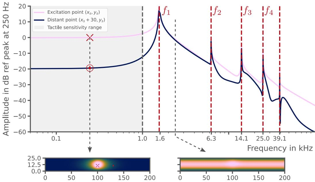
Figure 3.2: Numerical solutions of equation (3.34) in the frequency domain at the excitation point ( $x_s = 100$  mm,  $y_s = 3W/7$ ) (light pink) and at a point 30 mm away on the x-axis (dark blue). Frequencies from 0 to 1.6 kHz are said to be non-propagative. At these frequencies, amplitudes at the center of the actuator are theoretically higher than elsewhere on the plate. After the first cut-off frequency  $f_1$ , modes begin to propagate.
