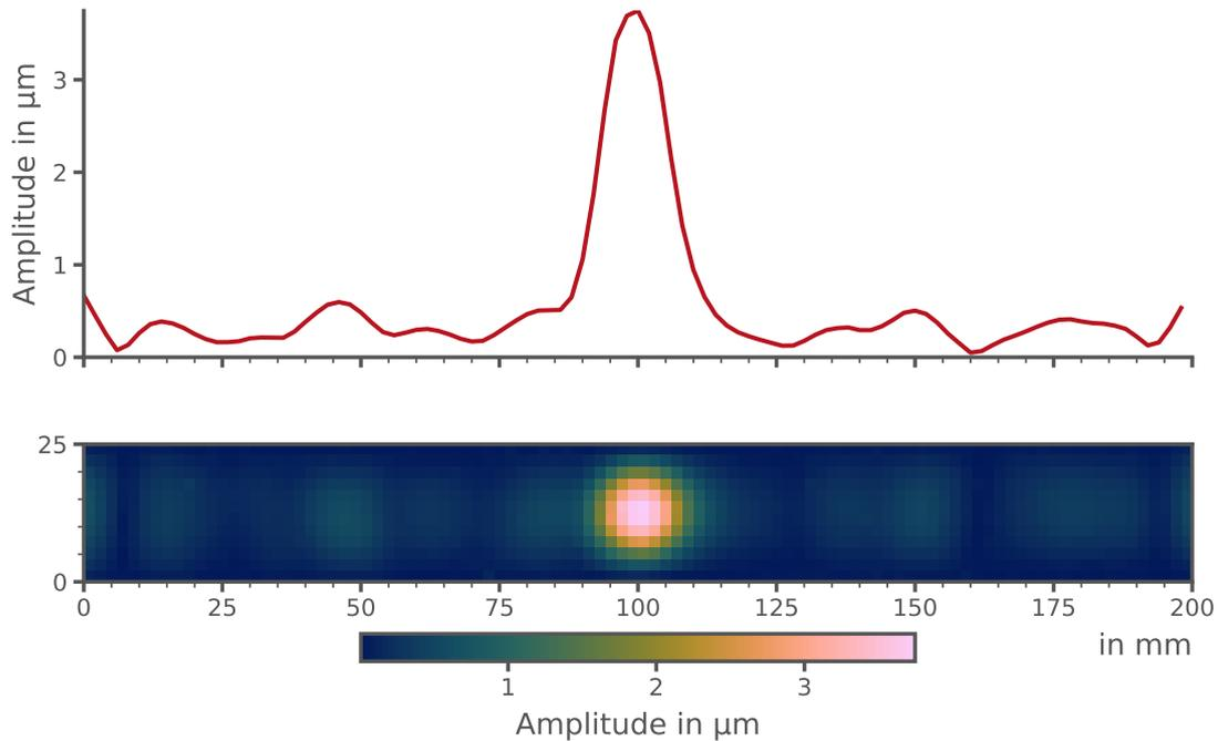
Figure 3.5: Quadratic mean of the measured displacement across the plate ( $200 \times 25 \times 0.4 \text{ mm}^3$ ) under a 250 Hz harmonic excitation of 100 V amplitude. The area above the piezoelectric actuator has an amplitude of  $4.6 \mu\text{m}$  whereas the rest of the plate stays at a negligible amplitude.
