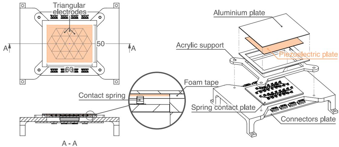
Figure 5.5: Experimental setup. A piezoelectric plate with a laserized triangular electrode pattern is glued to an aluminium plate. A plate with a set of spring assure the wiring of all 32 electrodes.
