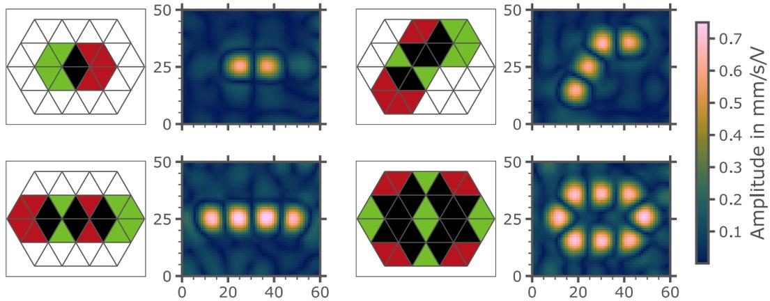
Figure 5.9: FRF mapping showing the behavior of the aluminium plate at the non-radiating frequency  $f = 25.6$  kHz. Electrodes are activated in counter phase and overlapping zone are powered with no tension (in black).
