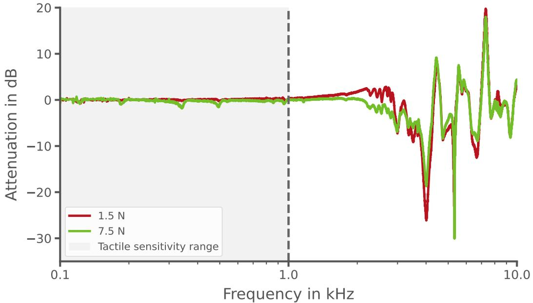
Figure 3.14: Experimental attenuation curve  $\mu_{\text{dB}} = 20 \log_{10} |\mu|$  obtain by realizing the ratio between loaded displacement  $\tilde{U}$  and free displacement  $U$  of the plate with different applied forces. As the model predicted, there's no attenuation due to the finger interaction on the tactile sensitivity range.
