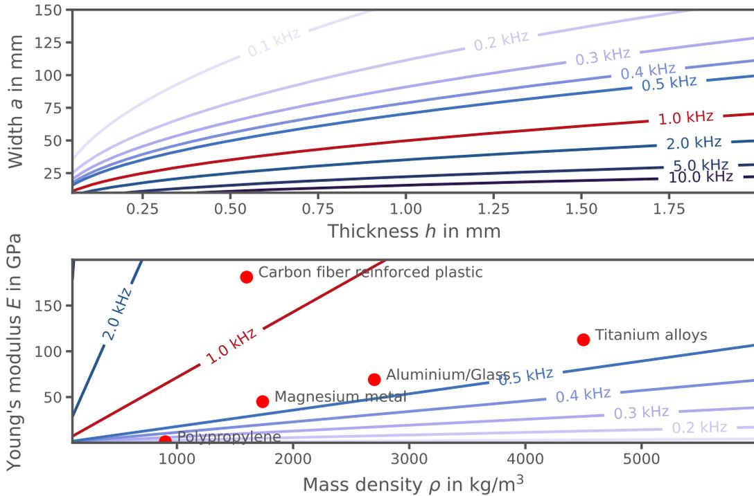
Figure 4.2: Abacus. Upper: First mode frequency abacus of a glass plate depending on its geometrical properties. Lower: First mode frequency abacus of a  $75 \times 75 \times 0.7 \text{ mm}^3$  plate depending on its material properties ( $\nu = 0.3$ ).
