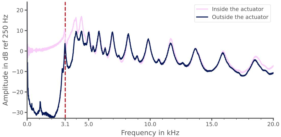
Figure 3.4: Averaged measured frequency response function (FRF)  $H_{dB} = 20 \log_{10} |H|$  inside and outside the activated actuator. The frequencies between 0 and 3.1 kHz are non-propagative. Within this range, amplitudes at the center of the actuator are about 30 dB larger than elsewhere on the plate.
