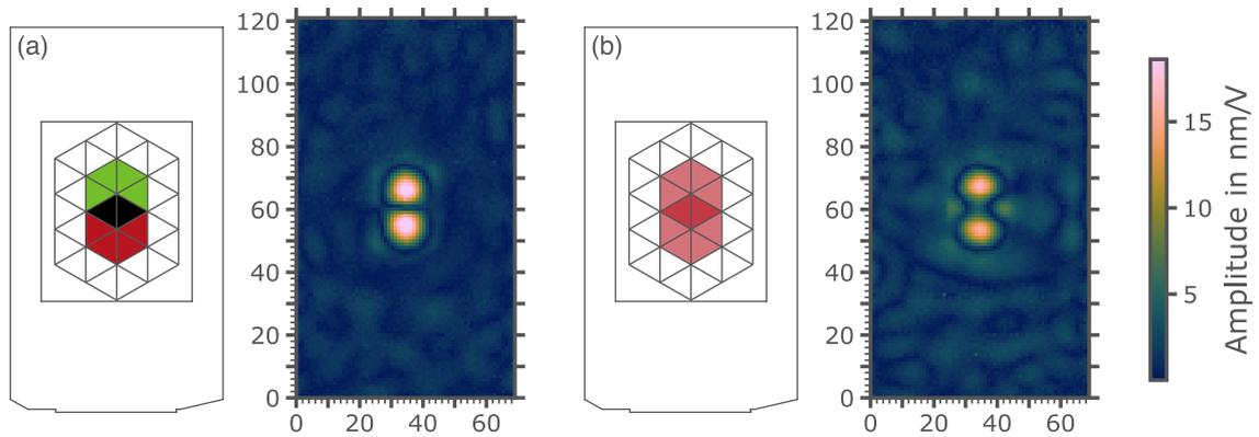
Figure 5.13: FRF mapping showing the behavior of an OLED screen at the non-radiating frequency  $f = 17.76$  kHz. (a) Electrodes are activated in counter phase and overlapping zones are powered with no tension. (b) Activated electrodes are added so that overlapping zone are powered with twice the base tension.
