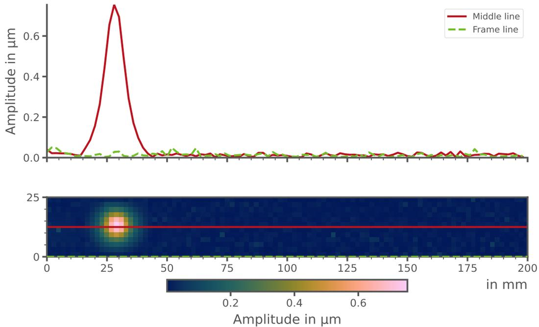
Figure 3.9: Quadratic mean of the measured displacement across the plate excited by a squared piezoelectric actuator (100 V/250 Hz) with a  $7 \times 7 \text{ mm}^2$  contact geometry. Vibrations are localized in the actuator region and reach a maximum RMS amplitude of  $0.75 \mu\text{m}$  at the center of the actuator.
