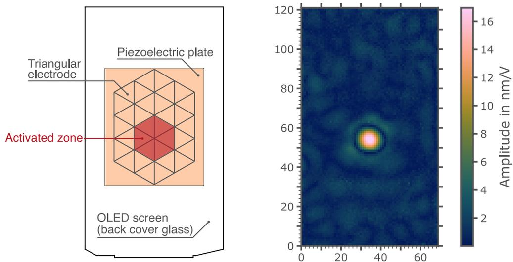
Figure 5.12: A group of 6 piezoelectric actuators forming an hexagon is powered by a sweep signal. The absolute value of the system frequency response function  $|H|$  is represented at the non-radiating frequency  $f = 17.76$  kHz and a localized effect can be observed above the activated zone.
