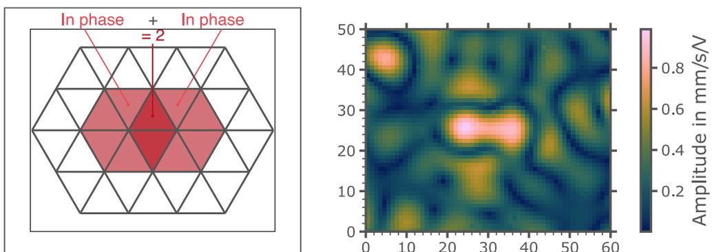
Figure 5.8: FRF mapping showing the behavior of the aluminium plate at the non-radiating frequency  $f = 25.6$  kHz. Electrodes are activated in phase and overlapping zone are powered with twice the base tension.
