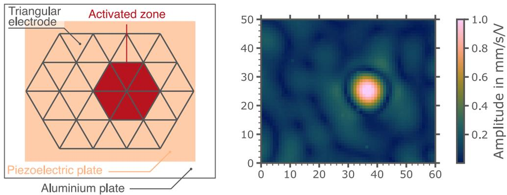
Figure 5.7: A group of 6 piezoelectric actuators forming an hexagon is powered by a sweep signal. The system frequency response function  $H$  is represented at the non-radiating frequency  $f = 25.6$  kHz and a localized effect can be observed above the activated zone.
