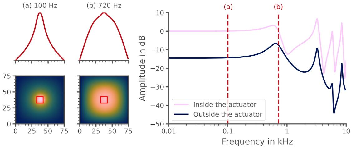
Figure 4.1: Simulation of a  $75 \times 75 \times 0.7 \text{ mm}^3$  glass plate excited with a square piezoelectric actuator in its center. The first resonance is around 580 Hz. (a) Before the first resonance, we have an evanescent behavior. (b) After the first mode, propagation occurs and we have a uniform distribution of vibration energy across the surface.
