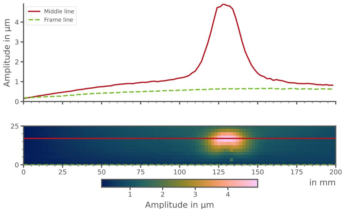
Figure 3.11: Quadratic mean of the measured displacement across the plate excited by an ERM with a contact geometry consisting of a  $10 \times 6 \text{ mm}^2$  rectangle. The plate presents a rigid body motion implied by the structure vibration which represented with a dashed line. Yet the localization effect is still present and shows a maximum rms amplitude of over  $4 \mu\text{m}$  in average.
