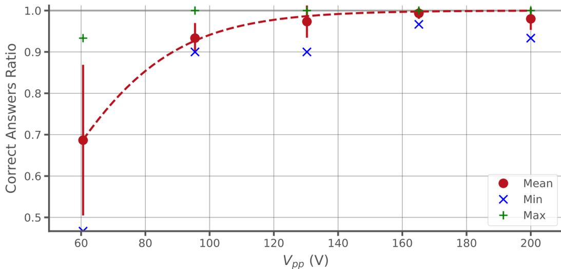
Figure 3.16: Correct answer ratio over all participants for each amplitude value. The ratio increase with the driving voltage amplitude. A high rate of correct answer ( $> 90\%$ ) is attained from  $V_{pp} = 95$  V (around  $4 \mu\text{m}$  peak-to-peak).
