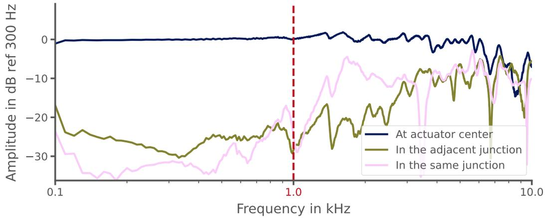
Figure 4.7: Experimental system frequency response function (FRF)  $H_{\text{dB}} = 20 \log_{10} |H|$  at the center of the activated actuator and outside in two points outside the actuator located in the adjacent junction and same junction to the actuator.
