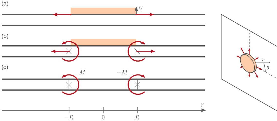
Figure 5.1: Pin force model of piezoelectric actuation. (a) A perfectly bounded piezoelectric patch (in yellow) produces two tangential forces at the plate surface localized at the actuator boundary in  $x = \pm R$ . (b) These tangential forces produce compression forces and bending moments in the plate. (c) For bending waves, the patch actuation resumes to two bending moments and an increased stiffness and density in the actuator-covered area.
