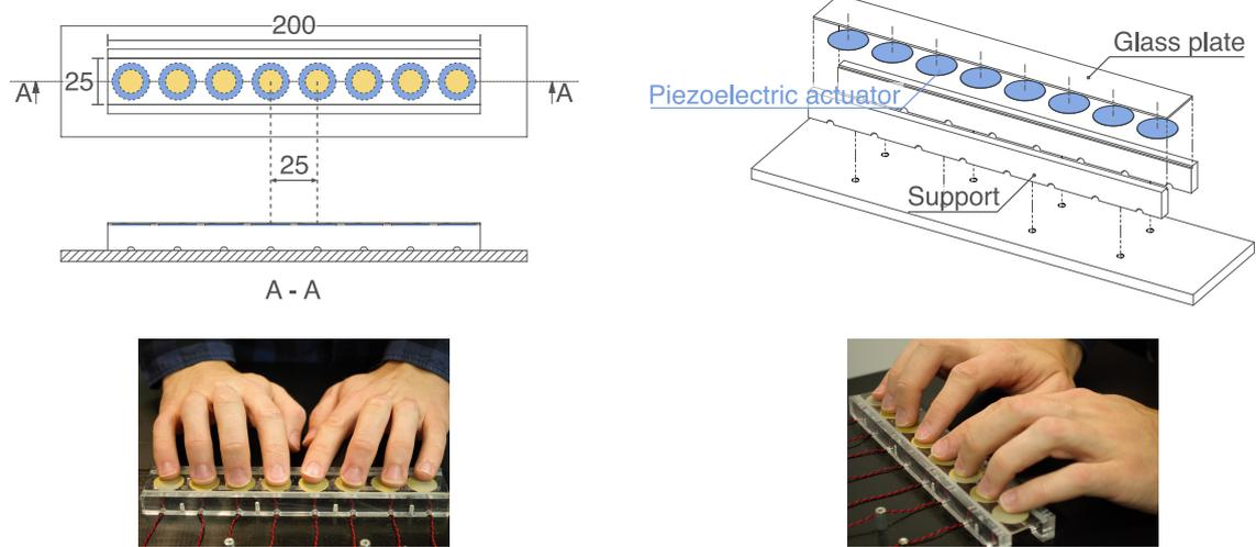
Figure 3.18: Demonstration prototype. A glass plate  $25 \times 200 \times 1 \text{ mm}^3$  is bounded on its longer edges on a rigid frame and a set of 8 piezoelectric actuators distant of 25 mm is applied on its bottom side.
