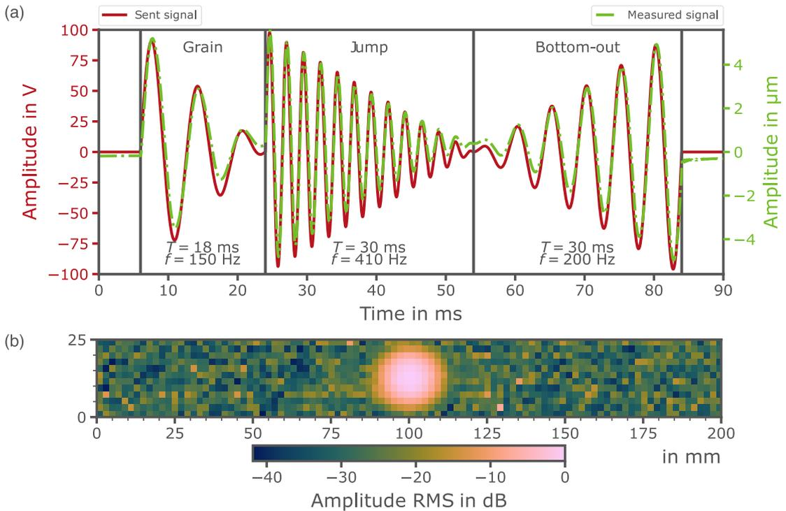
Figure 3.6: (a) Button pushing signal sent to the piezoelectric actuator (red solid line) and obtained displacement at its center (light green dashed line). Instantaneous response with high fidelity to the desired signal is obtained. (b) Quadratic mean of the measured out of plane displacement of the plate under the button pushing signal.
