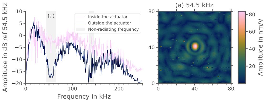
Figure 5.3: Averaged system frequency response function (FRF)  $H_{dB} = 20 \log_{10} |H|$  inside and outside the activated actuator. Around  $f = 54.5$  kHz a first drop in amplitude of  $-15$  dB can be observed, implying a higher amplitude in the center of the actuator than outside at this frequency. A second drop around 141 kHz seems to be happening but is polluted with resonances making it hard use.
