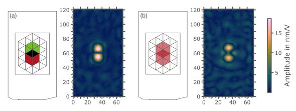
Figure 5.13: FRF mapping showing the behavior of an OLED screen at the non-radiating frequency f = 17.76 kHz. (a) Electrodes are activated in counter phase and overlapping zones are powered with no tension. (b) Activated electrodes are added so that overlapping zone are powered with twice the base tension.
