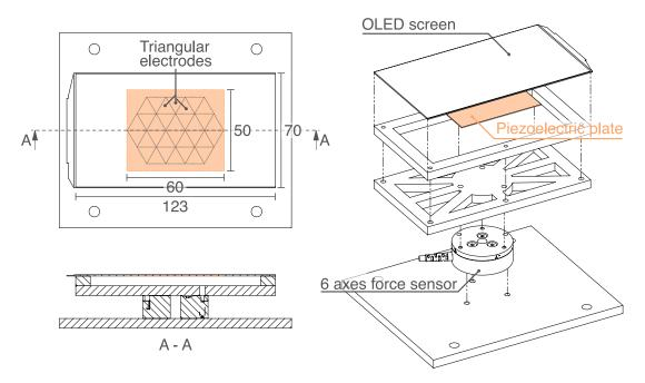
Figure 5.10: Experimental setup. A piezoelectric plate with a laserized triangular electrode pattern is glued to an OLED screen and mounted on a 6 axes force sensor.
