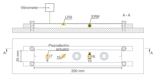
Figure 3.8: Upgraded experimental setup. Top: Three actuators are added to the bottom side of the previously used aluminum plate. The laser vibrometer measures the surface's out of plane displacement. Bottom: plate dimensions and actuator positions.
