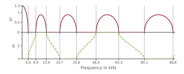
Figure 4.5: Representation of the real part (solid red line) and imaginary part (dashed green line) of the propagation constant  $\mu$  for a simply-supported semi-infinite plate of width  $L_y = 175$  mm on periodic rigid simple supports equispaced of  $L_x = 21.2$  mm. When  $\mu$  is real we have attenuation between each beam sections. When  $\mu$  is purely imaginary we have propagation. The alternation between real and imaginary part forms a set of propagation and attenuation band-gaps.
