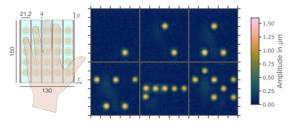
Figure 4.8: Quadratic mean of the out of plane displacement of the plate for 1, 2, 3, 5, 6 and 7 actuators activated at same time. Vibration sources are localized and reach a vibration rms amplitude above 1.6  $\mu$ m while most of the un-actuated area of the plate stays at rest.
