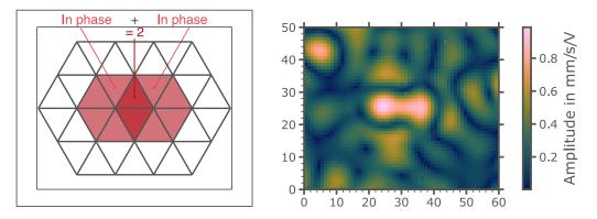
Figure 5.8: FRF mapping showing the behavior of the aluminium plate at the non-radiating frequency f = 25.6 kHz. Electrodes are activated in phase and overlapping zone are powered with twice the base tension.
