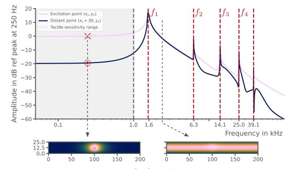
Figure 3.2: Numerical solutions of equation (3.34) in the frequency domain at the excitation point  $(x_s = 100 \text{ mm}, y_s = 3W/7)$  (light pink) and at a point 30 mm away on the x-axis (dark blue). Frequencies from 0 to 1.6 kHz are said to be non-propagative. At these frequencies, amplitudes at the center of the actuator are theoretically higher than elsewhere on the plate. After the first cut-off frequency  $f_1$ , modes begin to propagate.
