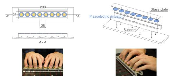
Figure 3.18: Demonstration prototype. A glass plate  $25 \times 200 \times 1 \text{ mm}^3$  is bounded on its longer edges on a rigid frame and a set of 8 piezoelectric actuators distant of 25 mm is applied on its bottom side.
