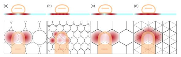
Figure 5.4: Piezoelectric distribution. a) Circular pattern. b) High density circular pattern. c) Hexagon pattern. d) Triangular pattern.
