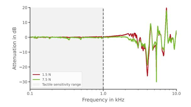
Figure 3.14: Experimental attenuation curve  $\mu_{dB} = 20 \log_{10} |\mu|$  obtain by realizing the ratio between loaded displacement  $\tilde{U}$  and free displacement U of the plate with different applied forces. As the model predicted, there's no attenuation due to the finger interaction on the tactile sensitivity range.
