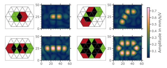
Figure 5.9: FRF mapping showing the behavior of the aluminium plate at the non-radiating frequency f = 25.6 kHz. Electrodes are activated in counter phase and overlapping zone are powered with no tension (in black).
