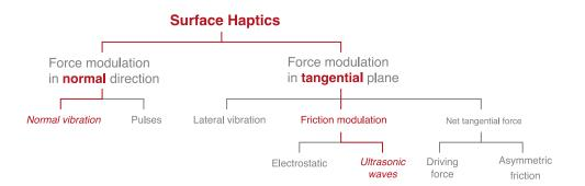
Figure 2.3: Classification of Basdogan et al. [21] of the current technologies for surface haptics displays based on the stimulation direction and method. Methods developed in this thesis are part of the highlighted elements.
