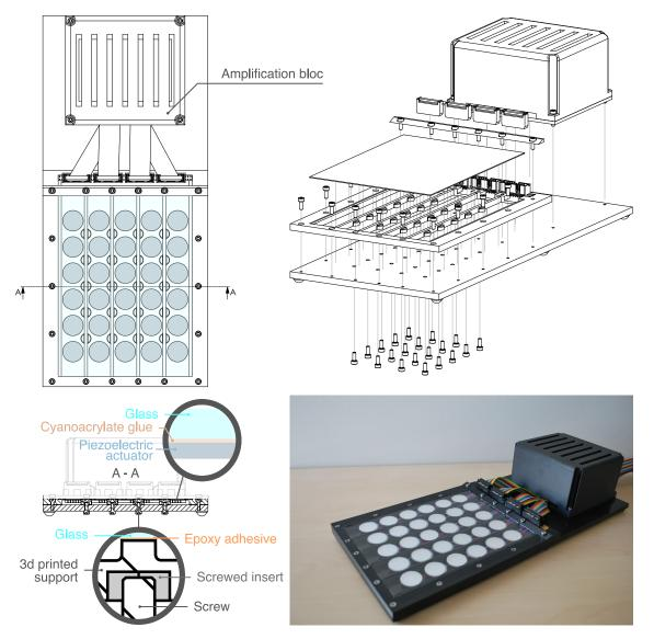
Figure 4.10: Demonstration prototype. A glass plate  $175 \times 130 \times 0.7 \text{ mm}^3$  is bounded to periodic rigid supports forming 5 sub-areas with a waveguide form. In each 5 sections 6 piezoelectric actuators were applied thus forming an array of 30 actuators with a spatial resolution of 25 mm.
