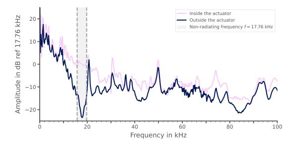
Figure 5.11: Averaged system frequency response function (FRF)  $H_{dB} = 20 \log_{10} |H|$  inside and outside the activated actuator. Around f = 17.76 kHz a drop in amplitude of -20 dB can be observed, implying a higher amplitude in the center of the actuator than outside at this frequency.
