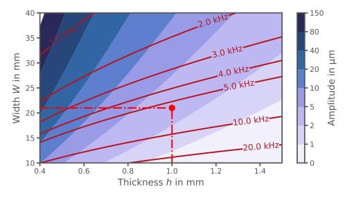
Figure 3.17: Analytic sizing map of a glass waveguide. A waveguide of width 21 mm and thickness 1 mm was chosen as it assured safety (for travel and during user interaction) as well as sufficient amplitude around 3  $\mu$ m and a high cut-off frequency around 6 kHz.
