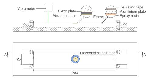
Figure 3.3: Experimental setup. Top: A piezoelectric actuator is glued to the bottom side of an aluminum plate. The laser vibrometer measures the surfaces out of plane displacement. Bottom: plate dimensions and actuator position.
