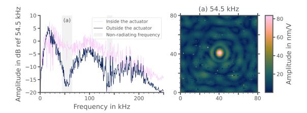
Figure 5.3: Averaged system frequency response function (FRF)  $H_{dB} = 20\log_{10}|H|$  inside and outside the activated actuator. Around f = 54.5 kHz a first drop in amplitude of -15 dB can be observed, implying a higher amplitude in the center of the actuator than outside at this frequency. A second drop around 141 kHz seems to be happening but is polluted with resonances making it hard use.
