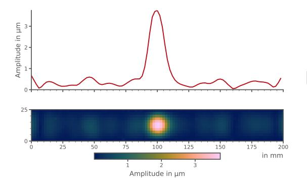
Figure 3.5: Quadratic mean of the measured displacement across the plate  $(200 \times 25 \times 0.4 \text{ mm}^3)$  under a 250 Hz harmonic excitation of 100 V amplitude. The area above the piezoelectric actuator has an amplitude of 4.6  $\mu$ m whereas the rest of the plate stays at a negligible amplitude.
