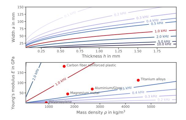
Figure 4.2: Abacus. Upper: First mode frequency abacus of a glass plate depending on its geometrical properties. Lower: First mode frequency abacus of a  $75 \times 75 \times 0.7$  mm<sup>3</sup> plate depending on its material properties ( $\nu = 0.3$ ).
