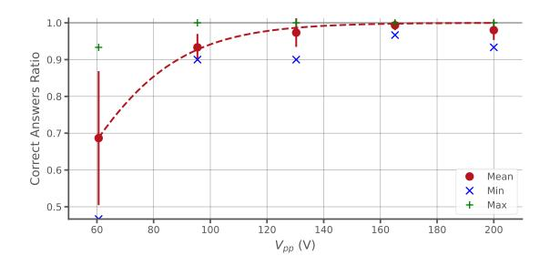
Figure 3.16: Correct answer ratio over all participants for each amplitude value. The ratio increase with the driving voltage amplitude. A high rate of correct answer (> 90%) is attained from  $V_{pp}$  = 95 V (around 4  $\mu$ m peak-to-peak).
