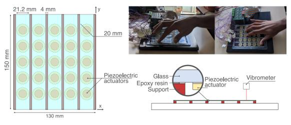
Figure 4.6: Experimental setup. A glass plate is bounded onto a set of 6 equidistant supports with epoxy resin. The actuators are glued to the bottom of the plate, 5 per area between each rib, for a total of 25 actuators.
