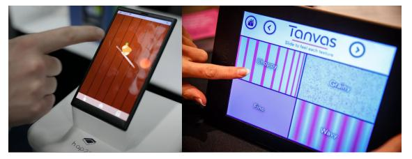
Figure 2.6: Left: Startup Hap2U using modal-based friction modulation to provide in-game haptic feedback on a smartphone-like demonstrator. Right: Startup Tanvas using electrostatic-based friction modulation to simulate texture to a user's finger (Josh Miller/CNET).
