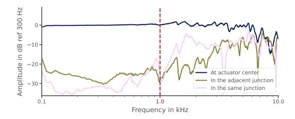
Figure 4.7: Experimental system frequency response function (FRF)  $H_{dB} = 20 \log_{10} |H|$  at the center of the activated actuator and outside in two points outside the actuator located in the adjacent junction and same junction to the actuator.
