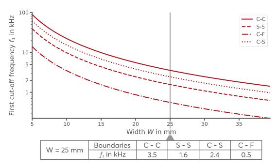
Figure 3.1: Cut-off frequency value depending on the width of the plate and the boundary conditions.
