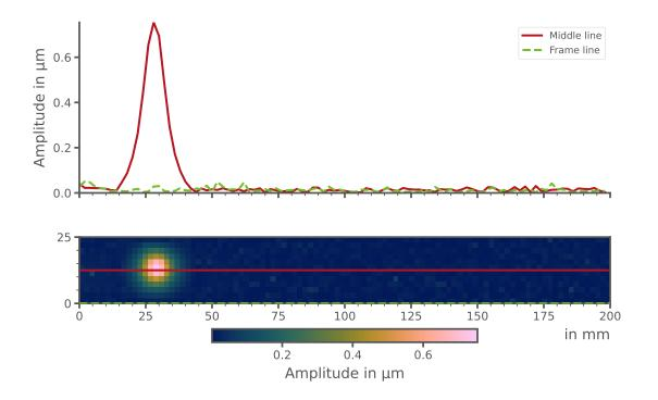
Figure 3.9: Quadratic mean of the measured displacement across the plate excited by a squared piezoelectric actuator (100 V/250 Hz) with a  $7 \times 7 \text{ mm}^2$  contact geometry. Vibrations are localized in the actuator region and reach a maximum RMS amplitude of 0.75  $\mu$ m at the center of the actuator.
