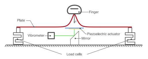
Figure 3.13: Setup for the measurement of the peak displacement attenuation in the center of the actuated area due to finger contact. The vibrometer laser beam was deflected by a mirror and reflected back on the bottom side of the piezoelectric actuator. Two load cells measured the force exerted by the finger.
