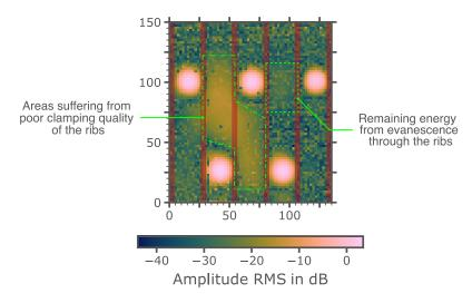
Figure 4.9: Quadratic mean with a logarithmic scale of the plate submitted to 5 activated actuators. Most of the energy is localized above each piezoelectric actuator but leaks due to poor bounding conditions can be noticed.
