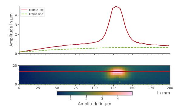
Figure 3.11: Quadratic mean of the measured displacement across the plate excited by an ERM with a contact geometry consisting of a  $10 \times 6 \text{ mm}^2$  rectangle. The plate presents a rigid body motion implied by the structure vibration which represented with a dashed line. Yet the localization effect is still present and shows a maximum rms amplitude of over 4  $\mu$ m in average.
