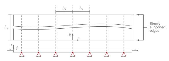
Figure 4.4: Plate bounded to a set of equispaced identical supports in the *y*-direction and simply-supported on its *x*-wise edges.
