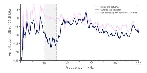
Figure 5.6: Averaged system frequency response function (FRF)  $H_{dB} = 20 \log_{10} |H|$  inside and outside the activated actuator. Around f = 25.6 kHz a drop in amplitude of 15 dB can be observed, implying a higher amplitude in the center of the actuator than outside at this frequency.
