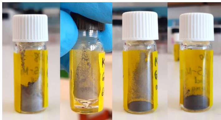
Figure 2 Samples made with Mo(+VI) precursor, from left to right: x = 0.05, 0.18, 0.25 and 0.43 . Their colors go darker from left to right, from brown to very dark brown, close to black.
