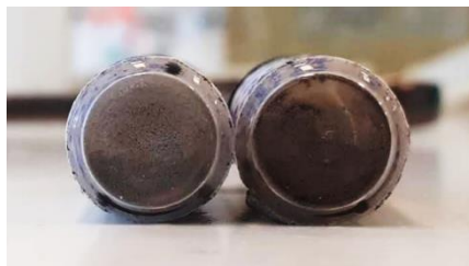
Figure 4 Samples made with Mo(+III) precursor: x from left to right: 0.05, 0.18. Their colors are much darker than powders made with 2 other precursors: very dark brown for sample x = 0.05 and black for sample x = 0.18 .
