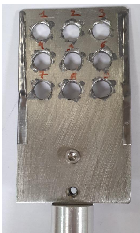
Figure 4 Pellets on holder for measurements on SAMBA Beamline.
