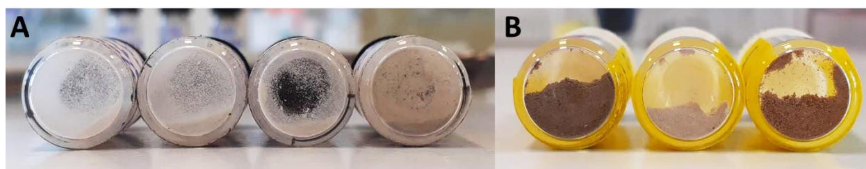
Figure 3 Samples made with Mo(+I) precursor: (A) x from left to right: 0.05, 0.11, 0.18, 0.25. The sample color becomes darker when x increase from 0.05 to 0.30, from off-white to light brown. (B) x from left to right: 0.43, 1, 2.03. The color does not go darker from left to right: from brown to light brown then brown but it is coherent with the elemental analysis result which will be discussed later in this chapter.
