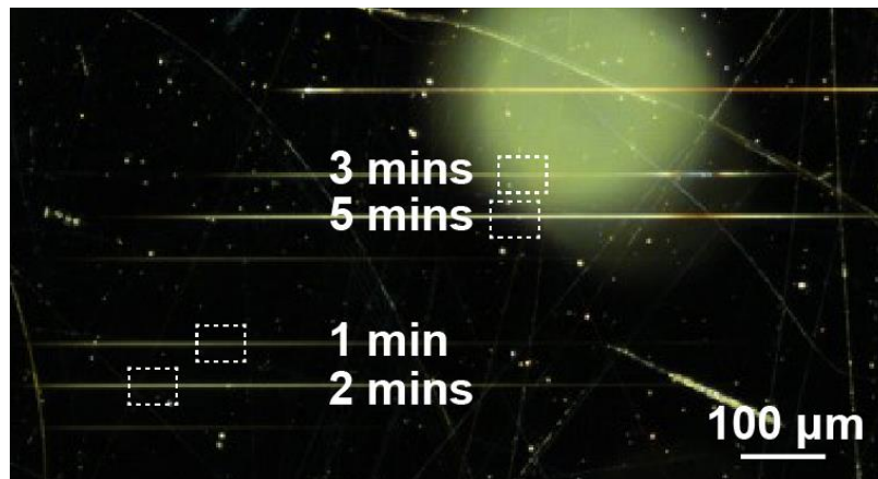
Figure 2-10 CCD image of polymer ridges made with mixture R 1 with different exposure times.
