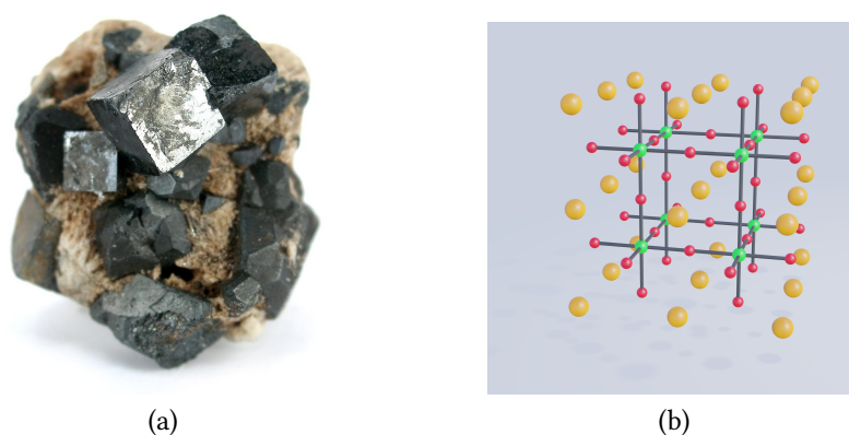
Figure 2.1 – (a) Crystals of perovskites in mineral matrix from Magnet Cove, Arkansas, USA. The cubic structure, particularly unusual for a natural compound, is clearly visible. (credits Wikimedia Commons) (b) 3D Structure of a perovskite ( \text{ABX}_3 ): in red the X atoms, cations, in green the B atoms and in yellow the A atoms. Both A and B are metal cations, with B atoms smaller than the A ones.
