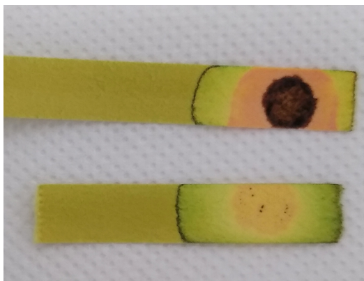
Figure 2.13: Drops of GO suspensions in water deposited onto strips of pH indicator paper. Top: [GO] = 8.5 mg/mL. Bottom: [GO] = 85 \mu g/mL.
