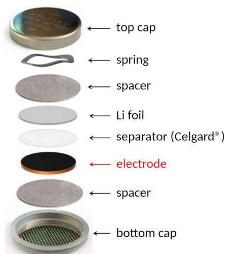
Figure 3.18: Exploded view drawing of a coin cell battery used for electrochemical tests, displaying all the components employed.
