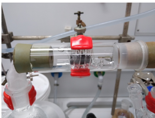
Figure 2.21: Part of the experimental setup used for reduction with N_2H_4 vapors, showing the cylinder with the aerogel mounted on a glass spiral.
