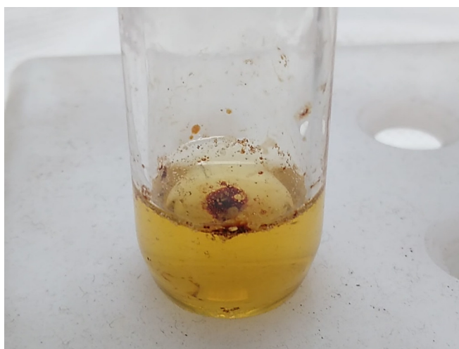
Figure 4: A photograph showing nitrogen bubbles forming on the interface between \text{H}_2\text{N-EMI}^+\text{TFSI} and water during a nitrous acid test.
