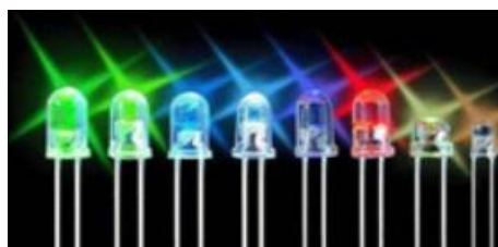
Figure 1-4 : Puces à LED DIP [8]
