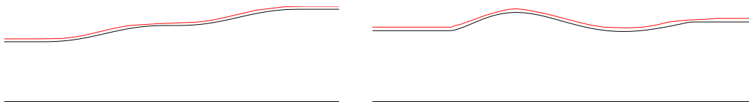
Figure 1.16 – Reconstruction of width defects in slowly varying waveguides given surface measurements. Black lines represent the initial shape of \Omega , and red ones the reconstruction of \Omega , slightly shifted for comparison purposes.
