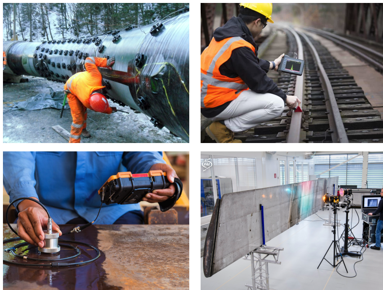
Figure 1.1 – From [89, 106, 108]: Practitioners non-destructive health monitoring of waveguides. Top left: monitoring of a pipeline. Top right: monitoring of train tracks. Bottom left: monitoring of a metal plate. Bottom right: monitoring of a large aircraft part.
