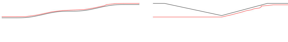
Figure 1.17 – Reconstruction of width defects in slowly varying waveguides given section measurements. Black lines represent the initial shape of \Omega , and red ones the reconstruction of \Omega , slightly shifted for comparison purposes.
