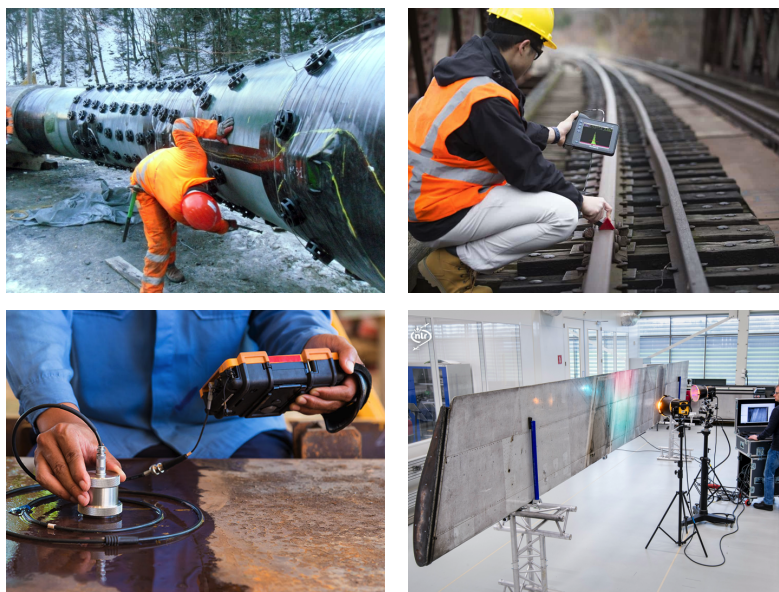
Figure 1.1 – From [89, 106, 108]: Practitioners non-destructive health monitoring of waveguides. Top left: monitoring of a pipeline. Top right: monitoring of train tracks. Bottom left: monitoring of a metal plate. Bottom right: monitoring of a large aircraft part.
