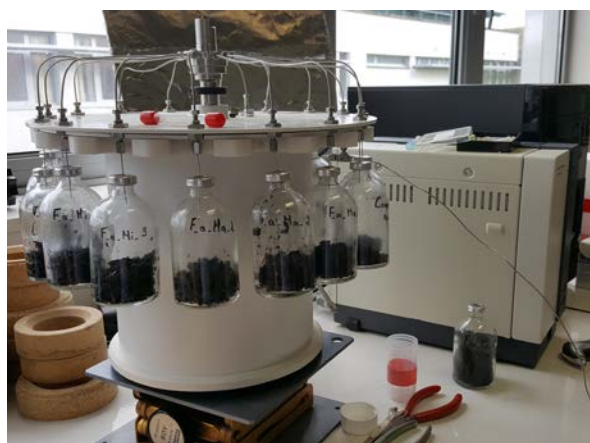
Figure 29 Measure of the CO 2 -C released by the samples during the incubation, using a micro-GC.
