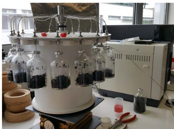
**Figure 29** Measure of the CO<sub>2</sub>-C released by the samples during the incubation, using a micro-GC.
