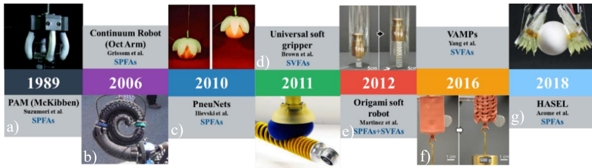
Figure 2.3. Timeline showing major production advances in the field of SFAs: a) PAM mechanism developed by Suzumori et al. [97], b) OctArm [98], c) PneuNets [99], d) Universal gripper [100], e) Origami soft structure [101], f) VAMPs design [102], and g) HASEL actuator [72].
