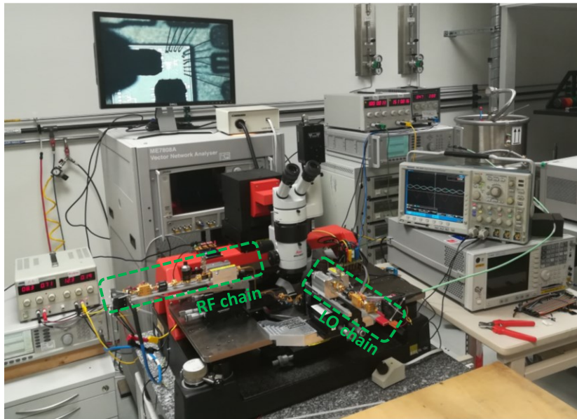
Figure 2-29: 60-90 GHz RF-probe measurement bench.
