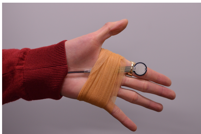
Figure 3.4: A force-sensing resistor used as a rhythm interface, to be used combined with a theremin. The sensor is held in place in the hand that also controls intensity, with the combination of a ring and a fabric strip.
