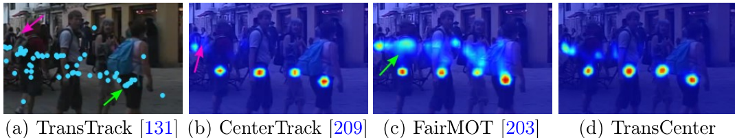
Figure 3.7: Detection outputs of state-of-the-art MOT methods: (a) shows the bounding-box centers from the queries in TransTrack [131]; (b), (c) are center heatmaps of CenterTrack [209], FairMOT [203], and (d) is from TransCenter.
