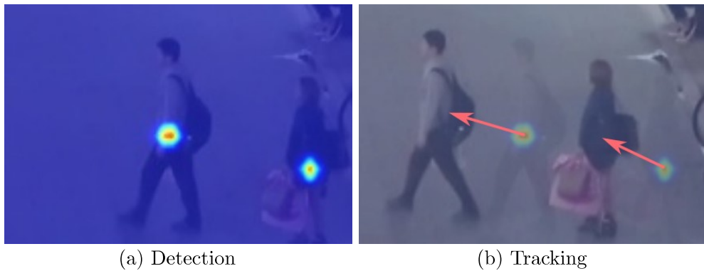
Figure 3.1: In our TransCenter, we propose to tackle the multiple-object tracking problem with transformers in an accurate and efficient manner: the dense non-overlapping representations provide sufficient and accurate detections through dense heatmap outputs as shown in (a); The sparse tracking queries, obtained from sampled features in object positions at the previous frame, efficiently produce the displacements of objects from the previous to the current time step, as shown in (b).
