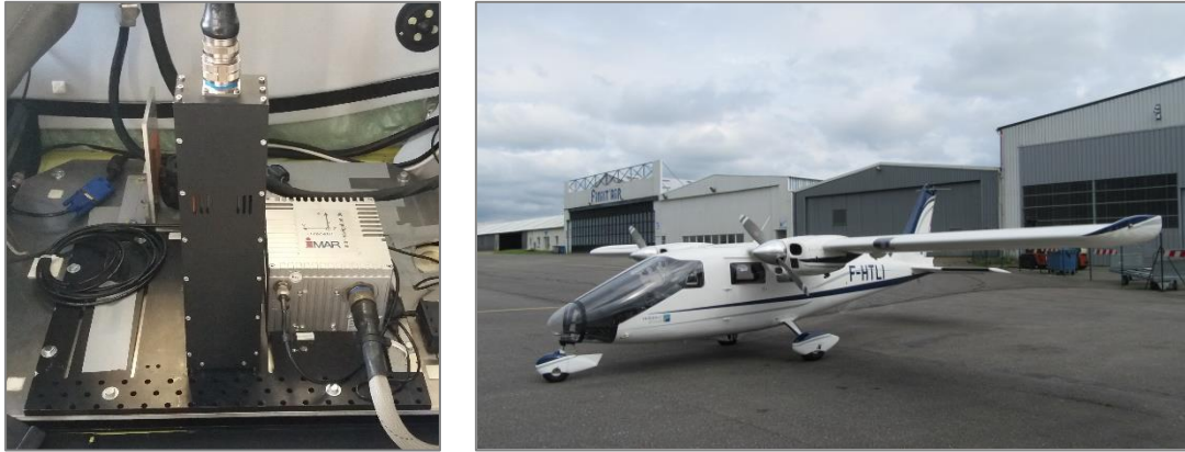
Figure 3.13. VNIR-1600 HySpex sensor and IMAR iTrace-RT-F200 navigation system (left), P68-Partenavia aircraft (right) used for the hyperspectral survey (credit: Hytech-imaging)
