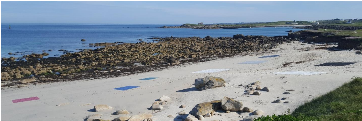
Figure 3.16. Calibration tarps positioned on the area of interest during the survey of site 2 and used for improving the atmospheric correction through empirical line fit
