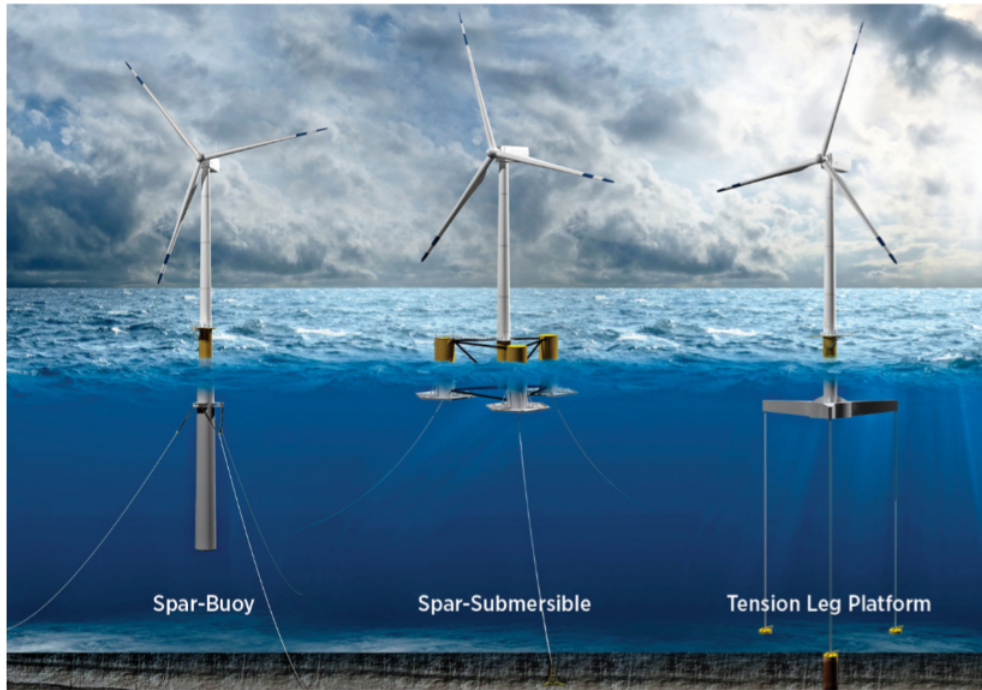
Figure 1.7 – Floating offshore wind turbines [Freeman et al., 2016]
