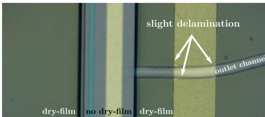
Figure 7.29: Slight delamination around the metal patterns even when using an adhesion promoter.
