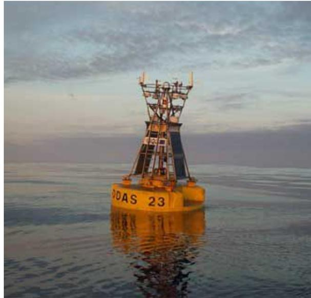
FIGURE 4.1 – *Non-directional Biscay buoy (station 62001) located at 45.230 N 5.000 W in the Bay of Biscay (at 4500 m depth) operated by UK Met Office and Meteo France (credits : [www.ndbc.noaa.gov](http://www.ndbc.noaa.gov)).*
