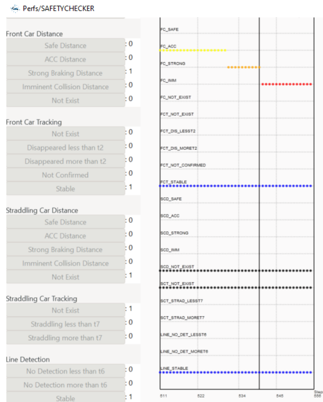
Figure 6.37: SAFETYCHECKER window showing states triggered for properties for step=2594.
