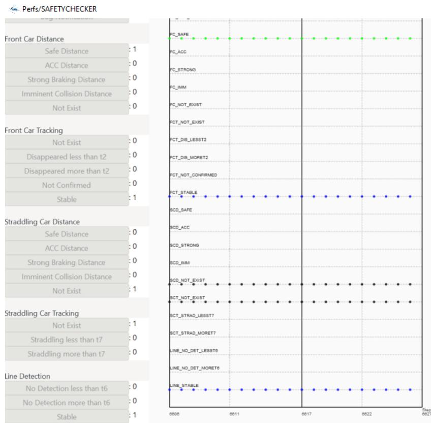
Figure 6.41: SAFETYCHECKER window showing states triggered for properties.
