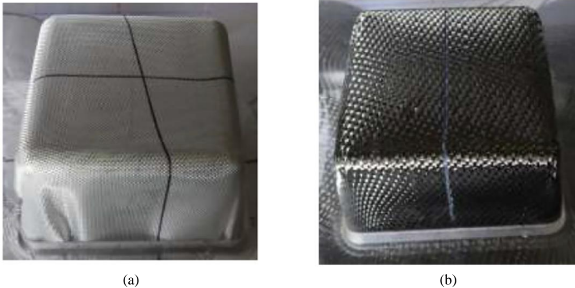
Fig. 4.3. Square box forming of a single layer oriented at 0^\circ/90^\circ . (a) Glass plain weave. (b) Carbon plain weave [J. Huang et al., 2021].
