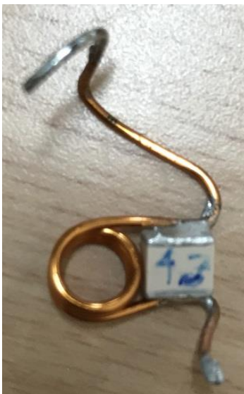
Figure 2.3- Actual view of the home-built ^1\text{H} trap tuned at approximately 40 MHz below the ^1\text{H} frequency.
