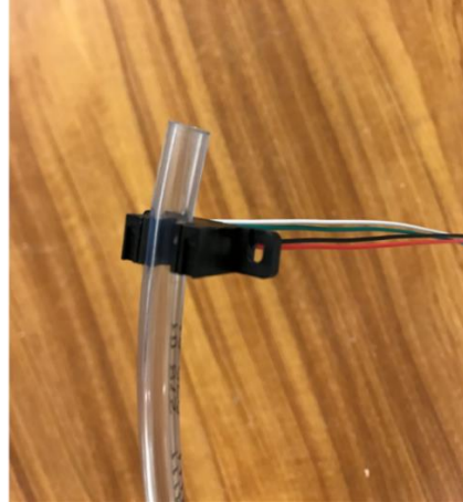
Figure 4.6- One of the two optical sensors for the measurement of the sample position and transfer speed which is fixed around the transfer tube.
