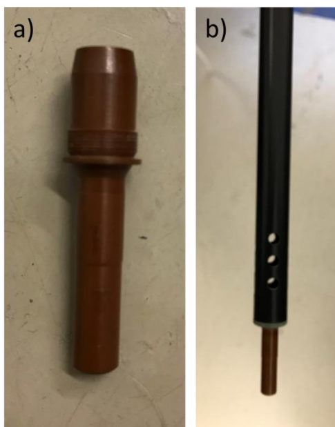
Figure 1.4- a) Low-temperature sample container made of PEEK. b) Sample container connected to the sample stick ready for insertion into the polarizer.
