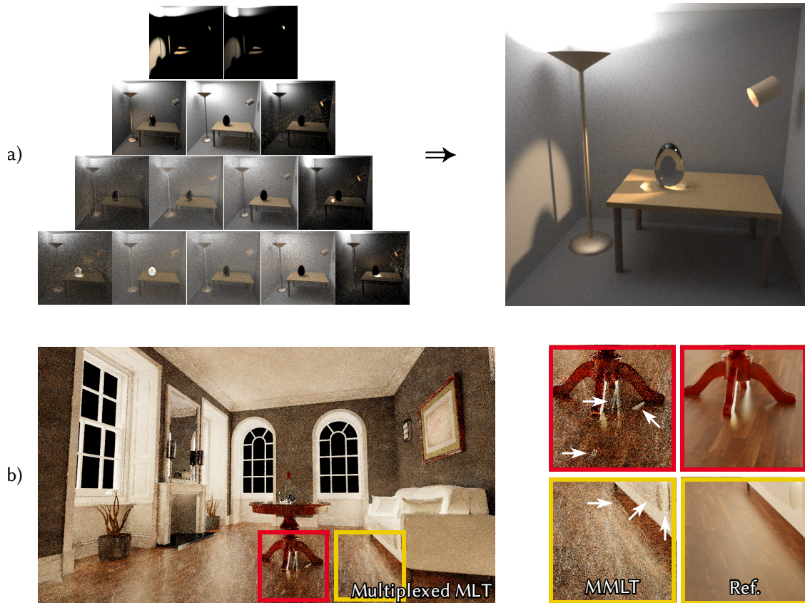
Figure 3.1: a) The images on the left are the result of connecting different vertices of the light and camera path in BDPT. All these images must be carefully weighted using multiple importance sampling to form the image on the right. Image from [111]. b) The splochiness inherent in MLT is visible on the diffuse walls of the living room and artifacts that MLT can produce are pointed with arrows on the right. Image from [10].
