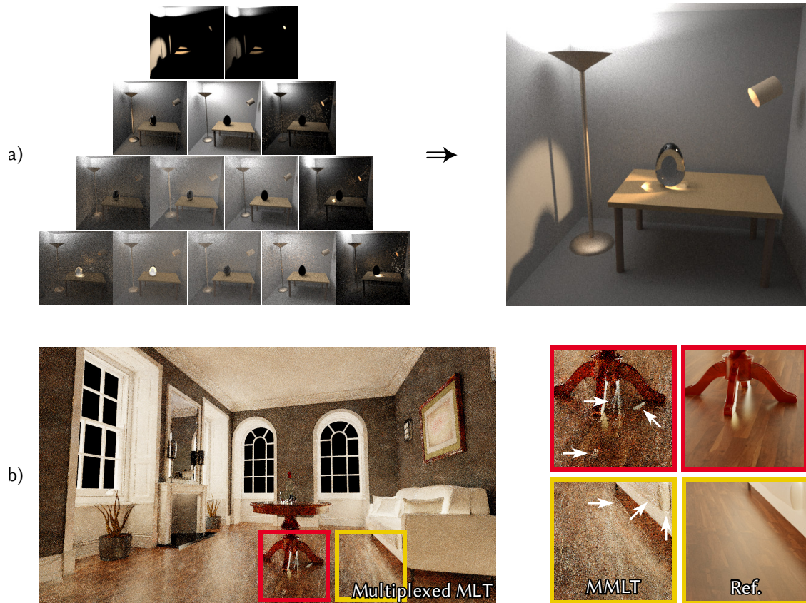
Figure 3.1: a) The images on the left are the result of connecting different vertices of the light and camera path in BDPT. All these images must be carefully weighted using multiple importance sampling to form the image on the right. Image from [111]. b) The splochininess inherent in MLT is visible on the diffuse walls of the living room and artifacts that MLT can produce are pointed with arrows on the right. Image from [10].
