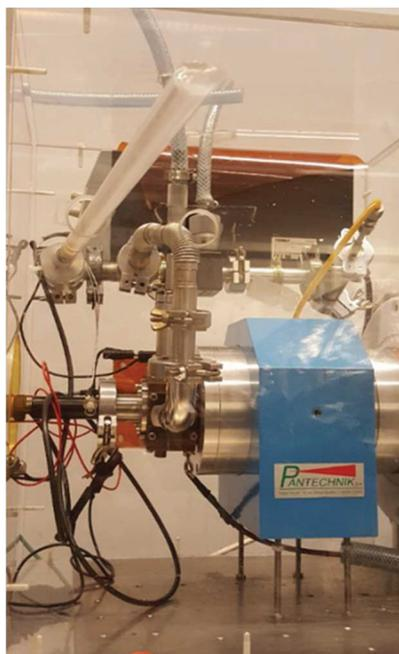
Figure 3-6: Photograph of the Nanogan I ECR ion source used in the present work.
