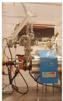
Figure 3-6: Photograph of the Nanogan I ECR ion source used in the present work.
