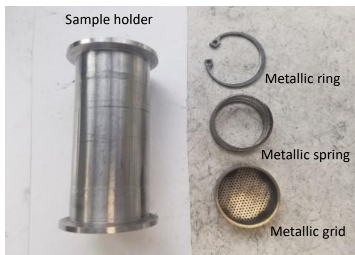
Figure 34. Different components for AC sample preparation
