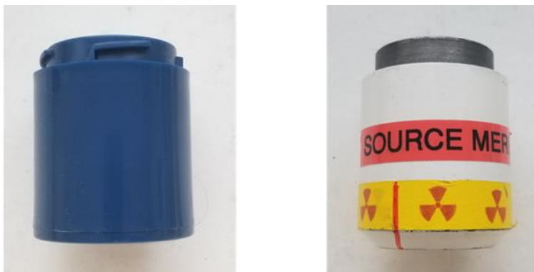
Figure S19. Different lead supports with different thickness for activity measurements
