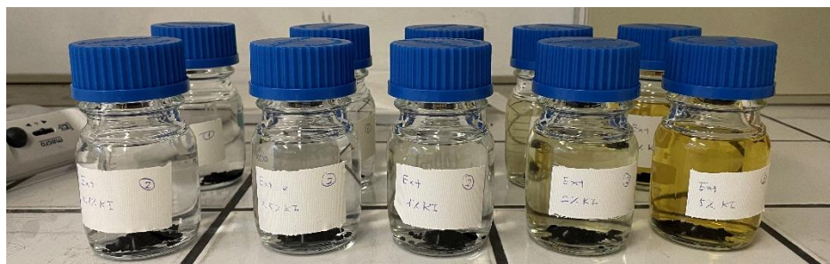
Figure S1. Yellow coloration during KI extraction (KI concentration increases from left to right)
