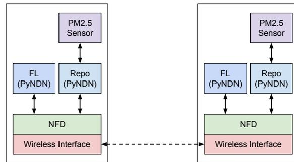
Figure 4.4 – The node architecture of ActiveNDN prototype
