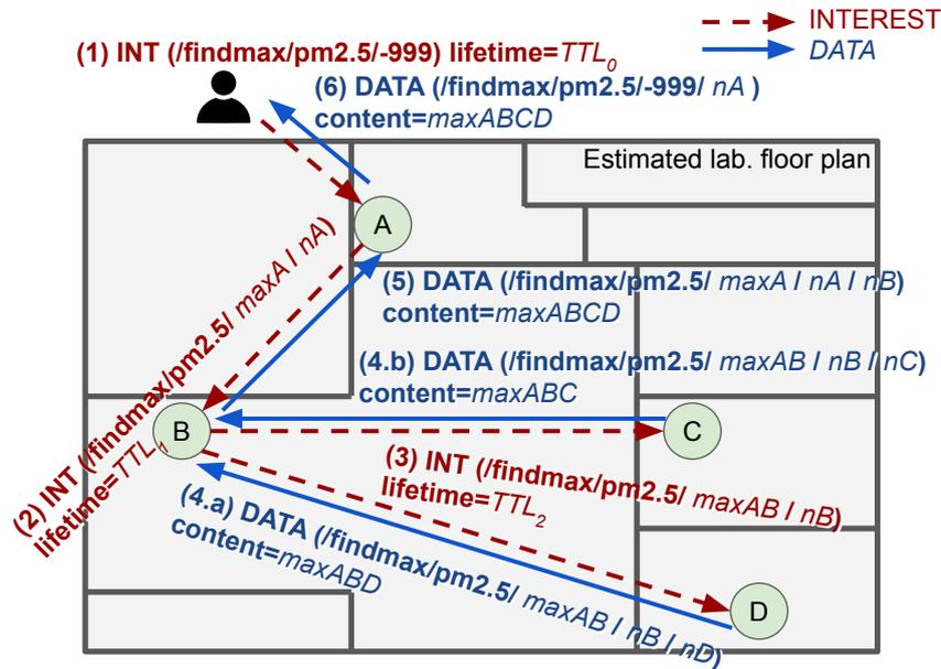
Figure 4.7 – Testbed node placement and visualized packets
