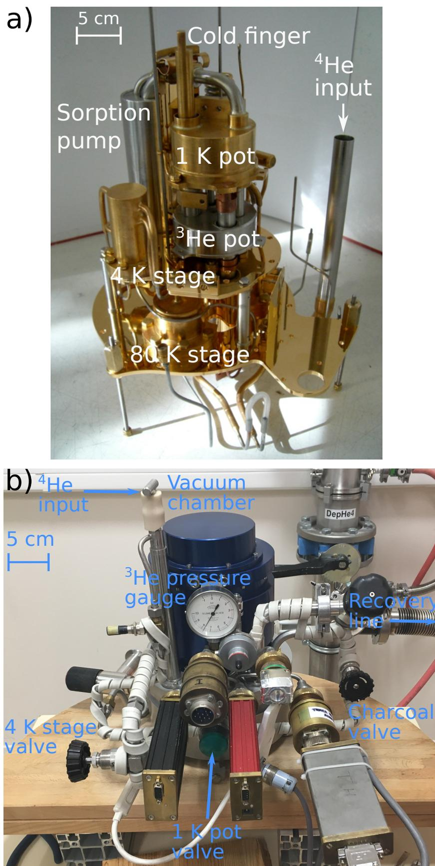
Figure 4.1 – Photos of the  $^3\text{He}$  Table-top cryostat (a) The internals of the cryostat without the shields, the sample stage or outer vacuum seal with important internal components labeled. (b) In place in the laboratory. The valves used to manipulate the  $^4\text{He}$  flow rate as well as other components are labeled.
