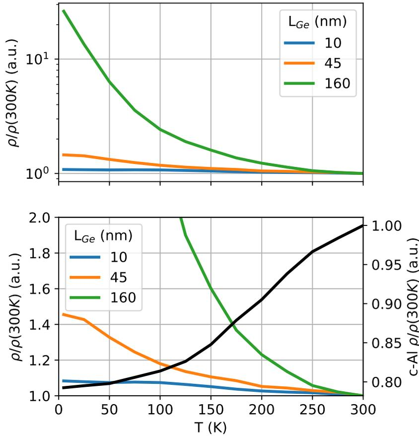
Figure 5.11 – Normalised resistivity ( $\rho/\rho(300\text{K})$ ) versus temperature ( $T$ ) of selected Al-Ge-Al devices from Figure 5.10, highlighting the temperature evolution of shorter devices. *Upper* Figure has a semilog scale whereas *lower* Figure has a linear scale with the c-Al NW device plotted in black whose scale is on the right axis.
