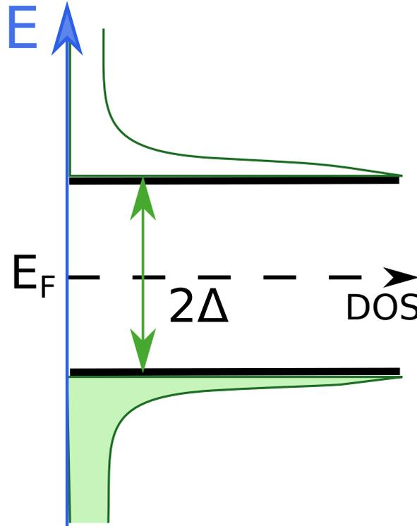
Figure A.1 – Quasiparticle spectrum of the superconducting ground state in the one-particle representation. In the ground state, all the quasiparticle states below  $E_F$  are filled, whereas all states above  $E_F$  are empty. Notably, all quasiparticle states of energy  $|E - E_F| < \Delta$  are forbidden. This defines the superconducting gap.
