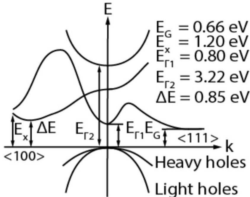
Figure 2.2 – Band structure of bulk germanium at 300 K. We can see the indirect band-gap labeled  $E_G$  and the direct band gap labeled  $E_{\Gamma}^x$ . We also observe light hole and heavy hole bands, which are degenerate near  $\vec{k} = 0$ . Figure taken from Ref. [39].
