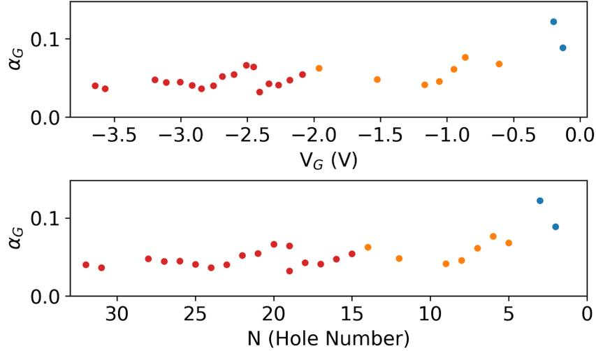
Figure 5.19 – **Gate lever arm**  $\alpha_G$  versus  $V_G$  &  $N$  for three independently measured datasets.  $\alpha_G = 0.49$  calculated by averaging  $\alpha_G$  in the gate region of ( $-3.75$  V <  $V_G$  <  $-2$  V)
