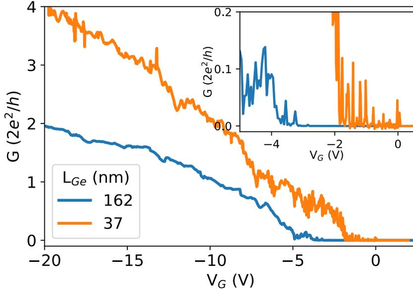
Figure 5.13 – **Transport overview** Conductance plotted in units of  $G_0$  as a function of back-gate voltage ( $V_G$ ) of an Al-Ge-Al heterostructure with a Ge segment of  $L_{Ge} \approx 162$  nm (blue) and  $L_{Ge} \approx 37$  nm (orange) for a bias voltage of 0.5 mV and 1 mV recorded at  $T = 350$  mK and  $T = 400$  mK, respectively. The inset shows a zoom of the conductance features just after pinch-off ( $-5.0$  V  $< V_G < 0.5$  V).
