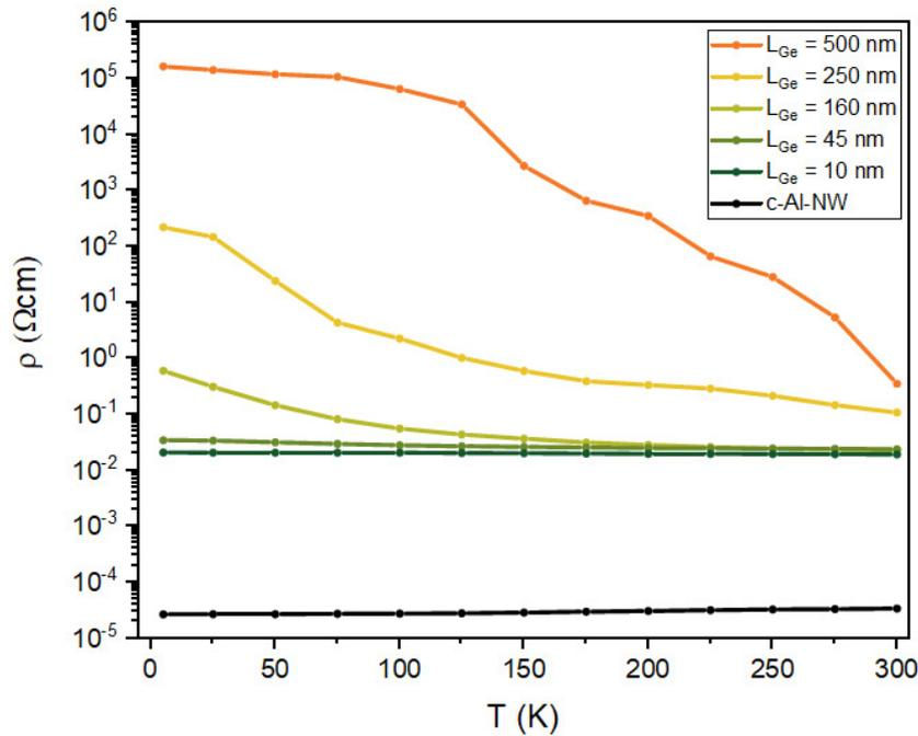
Figure 5.10 – Resistivity ( $\rho$ ) versus temperature ( $T$ ) of Al-Ge-Al devices with a range of Ge segment lengths ( $L_{Ge}$ ). The resistivity was calculated by taking a linear fit of an  $I_D-V_D$  curve measured at  $V_G = 0$  V. Also plotted is  $\rho$  vs  $T$  for a fully exchanged NW device (c-Al-NW).
