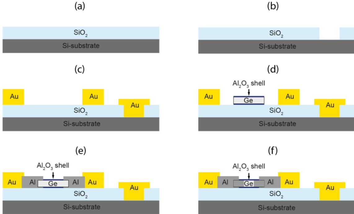
Figure 3.3 – Schematic of the fabrication process used to integrate Ge NWs into a FET architecture. (a) The highly *p*-doped Si substrate with a 100 nm SiO<sub>2</sub> insulating layer on-top. (b) Etched SiO<sub>2</sub> facilitating back-gate contact. (c) Au bonding pads deposited on the substrate. (d) Ge NW transfer by drop-casting. (e) Al contacts deposited to connect Ge NW to Au pads. (f) Formation of Al-Ge-Al NW heterostructure after thermal annealing process. Figure taken from Ref. [39]
