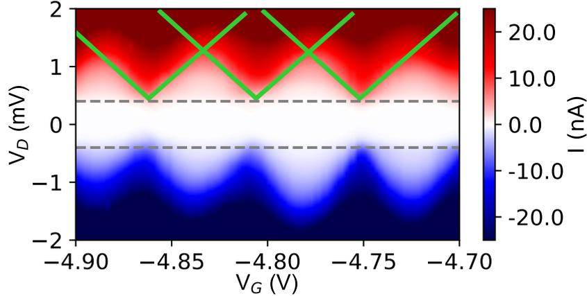
Figure 5.17 – **Coulomb diamond zoom** A zoom onto a few diamonds of Sample L1 revealing with greater clarity the transport gap due to the superconducting leads. The gap is traced by two grey dashed lines. Green lines that depict the extracted slopes used to calculate the capacitances are superimposed on the stability diagram.
