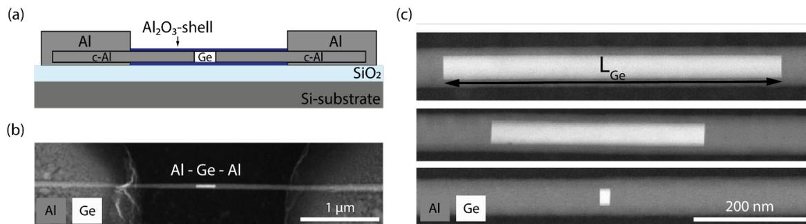
Figure 3.6 – (a) Schematic representation of the FET architecture after the annealing process. (b) STEM image of the architecture after the annealing process showing a monolithic Al-Ge-Al NW heterostructure coupled to large polycrystalline pads. (c) STEM image showing various Ge segments lengths achieved through the annealing process.
