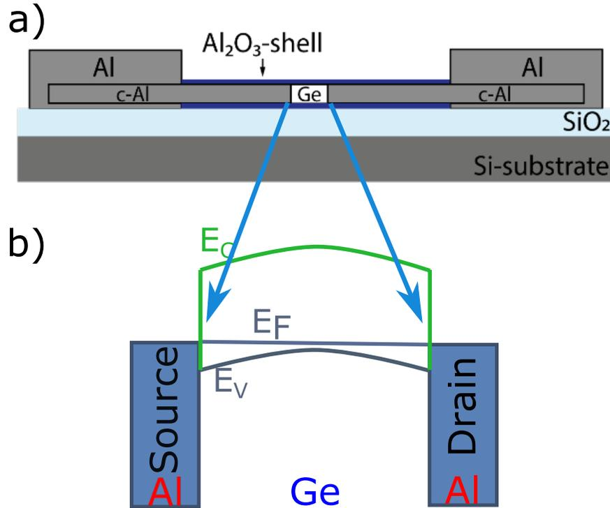
Figure 5.6 – (a) Schematic of an Al-Ge-Al nanowire heterostructure implemented into a back-gated field effect transistor (FET) with a band diagram (b) depicting the back-to-back Schottky barriers associated with the two Al-Ge interfaces. The valence band is pinned close to  $E_F$  of the Al leads due to Fermi level pinning.
