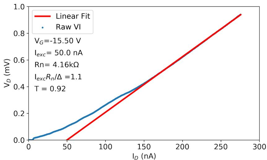
Figure 5.32 – Raw  $V_D$ - $I_D$  curve at  $V_G = -15.5$  V and linear fit of the curve in the normal regime  $V_D > 2\Delta/e$ . From the linear fit,  $R_N$  and  $I_{exc}$  is determined.  $R_N = 4.16$  k $\Omega$  is the gradient of linear fit and  $I_{exc} = 50$  nA is the x-axis intercept.
