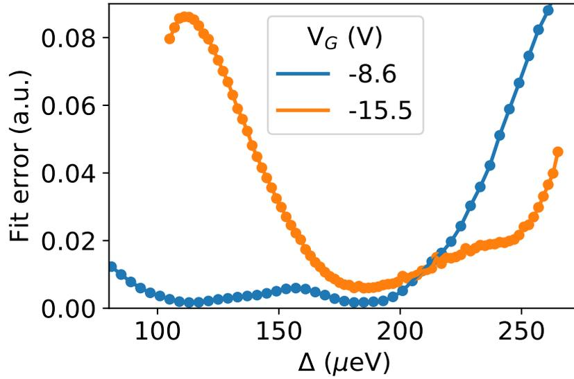
Figure 5.29 – Plot of fit error versus  $\Delta$  for fits of  $I_D$ - $V_D$  curves at  $V_G = -8.6$  V and  $V_G = -15.5$  V. The data was obtained from the *Gap search* to of the Monte-Carlo based fitting program.
