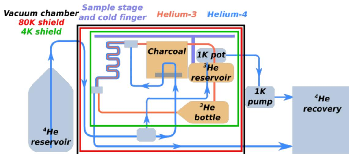
Figure 4.2 – Simplified schematic of the internal circuitry of the  $^3\text{He}$  Table-top cryostat. The  $^4\text{He}$  line is depicted in blue. Whereas, the  $^3\text{He}$  line is depicted in orange. The 80 K shield and 4 K shield are depicted in red and green, respectively. The sample stage and cold finger are depicted in purple. In this schematic the  $^3\text{He}$  pot is labeled as the  $^3\text{He}$  reservoir. The  $^3\text{He}$  Figure taken from Ref. [114].
