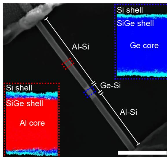
Figure 3.7 – STEM image of a monolithic Al-Ge-Al NW heterostructure core with a Si shell after the annealing process. Insets shows EDX measurements of the Ge segment and *c*-Al segment where Ge and Al cores with high purity are observed in the respective segments, which are wrapped by a continuous SiGe and Si shell. The scale bar is 200 nm.
