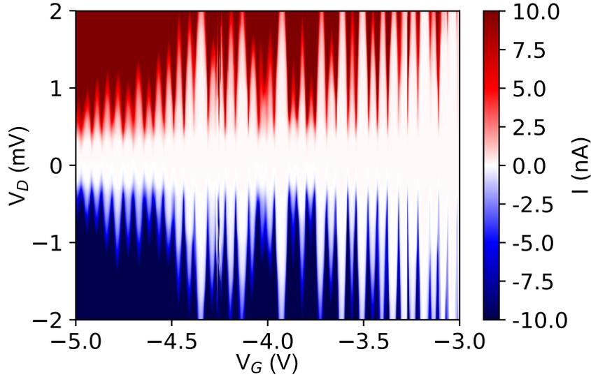
Figure 5.15 – **Stability diagram** Showing the measured current versus  $V_D$  and  $V_G$  of an heterostructure device with  $L_{Ge} = 162$  nm (Sample L1) recorded at  $T = 350$  mK.
