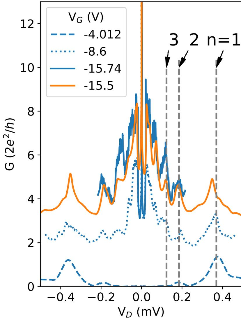
Figure 5.28 –  $G(V_D)$  curves for four  $V_G$  slices. For comparison both Sample 1 (blue curves) and Sample 2 are shown (orange curve). We see clear conductance peaks which we associate with MAR. The vertical grey dashed lines indicate the expected voltage position  $V_n = 2\Delta/ne$  of the first three MAR peaks for  $\Delta = 185\mu\text{eV}$ .
