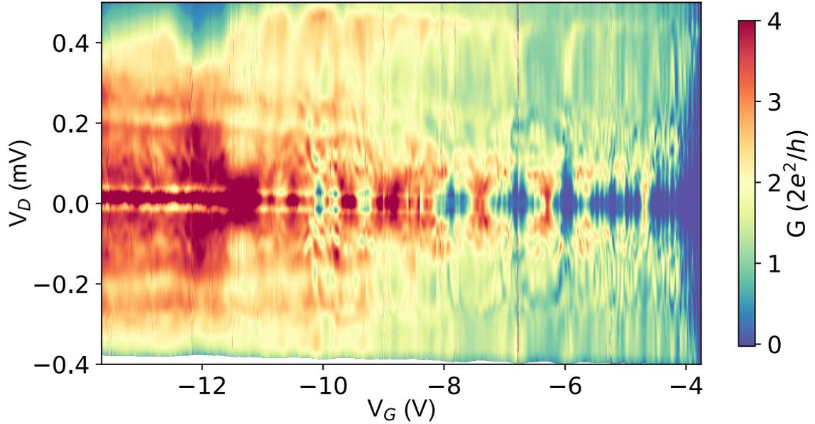
Figure 5.37 – **Intermediate regime transport overview:** Colorplot of differential conductance ( $G$ ) vs bias voltage ( $V_D$ ) and back gate voltage ( $V_G$ ). We observe large sub-gap conductance with Coulomb blockade like features at low  $V_D$  bias evolving into large zero-bias conductance peaks as  $V_D$  decreases.
