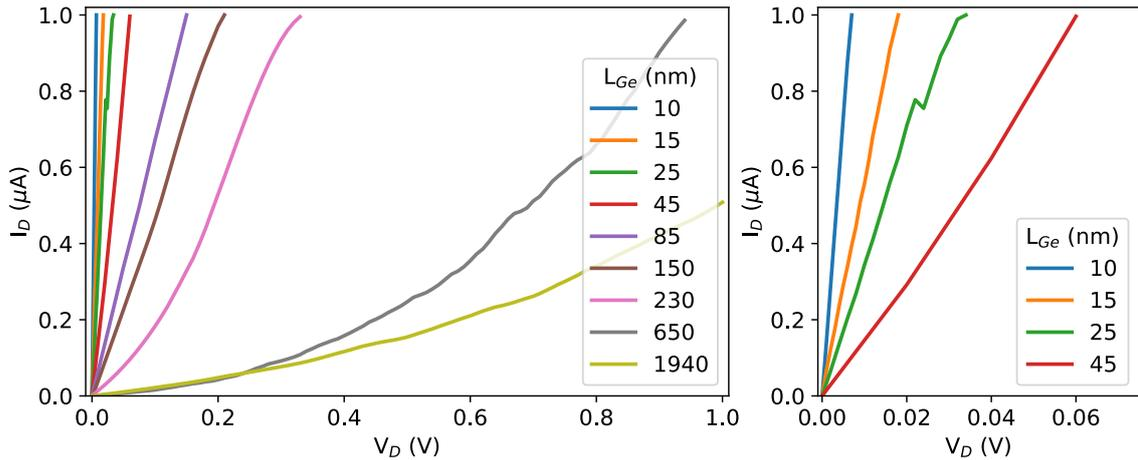
Figure 5.8 –  $I_{\text{D}}-V_{\text{D}}$  curves of Al-Ge-Al devices with a range of Ge segment lengths at room temperature ( $T \approx 300$  K) with  $V_{\text{G}} = 0$  V. *Right* shows a zoom of the  $I_{\text{D}}-V_{\text{D}}$  curves of the Al-Ge-Al devices with  $L_{\text{Ge}} < 45$  n. Data taken from Ref. [39].
