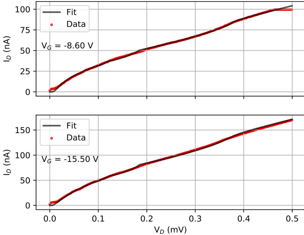
Figure 5.30 – **MAR fits** Shows fits (black) of I-V curves (red) at selected gate voltages. The fits were made using a program developed by Ref (AevCarlo) which uses Monte Carlo to converge to a fit of smallest error. The program provides an estimate of the number of conducting channels involved in the transport and the transparency of each channel (see Figure 5.31).
