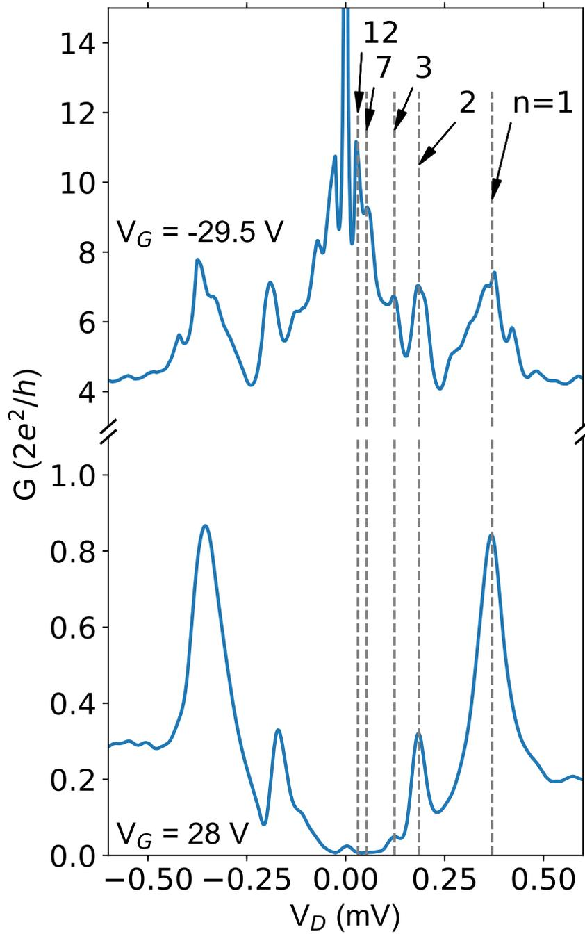
Figure 6.10 – Differential conductance slices ( $dI_D/dV_D$ ) with respect to  $V_D$  for  $V_G = -29.5$  V and 28 V measured at 450 mK. Vertical dashed lines at  $V_D = \frac{2\Delta}{ne}$  show the expected position of conductance peaks due to MAR for  $\Delta = 185\mu\text{eV}$ .
