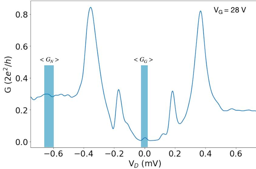
Figure 6.7 – Differential conductance slice ( $dI_D/dV_D$ ) with respect to  $V_D$  for  $V_G = 28 \text{ V}$  measured at  $450 \text{ mK}$ . The highlighted regions show where the average conductance is taken for each  $V_G$  slice to calculate the *gap hardness*.
