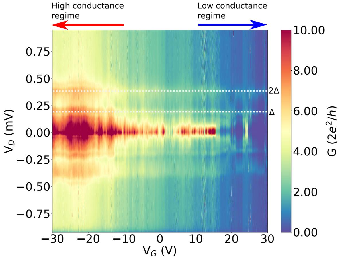
Figure 6.1 – **Transport Overview.** Density plot of differential conductance ( $dI_D/dV_D$ ) with respect to bias voltage ( $V_D$ ) and gate voltage ( $V_G$ ) of (a) Ge/Si core/shell NW sample recorded at 390 mK. We observe two distinct regimes: A low conductance regime  $V_G > 20$  V and a supercurrent (high conductance) regime ( $V_G < 10$  V).
