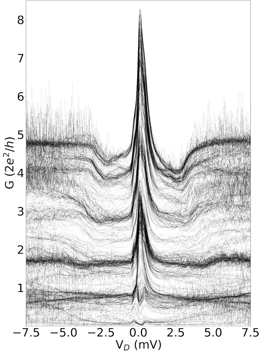
Figure 6.4 – Differential conductance ( $G$ ) with series resistance of  $370 \Omega$  subtracted waterfall plot from  $V_G = 30 \text{ V}$  to  $-30 \text{ V}$  in  $167 \mu\text{V}$  steps measured at  $T = 450 \text{ mK}$ .
