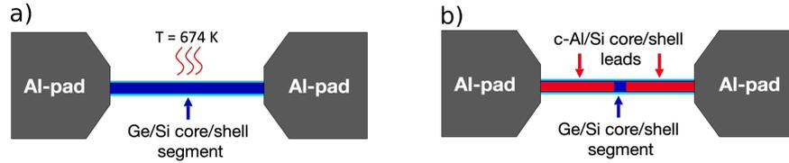
Figure 3.5 – Schematics presenting the thermal annealing process (a) that results in the diffusion of Ge out of the nanowire and into the Al pads. The diffused Ge is replaced by Al (b), forming monolithic Al-Ge-Al and Al-Ge/Si-Al core/shell NW heterostructures.
