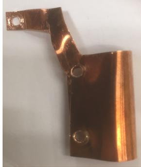
Figure 4.4 – Copper bracket encapsulating the charcoal sample.
