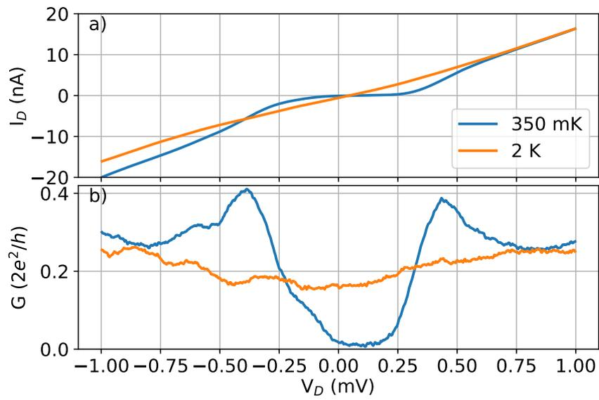
Figure 5.26 – (a)  $I_D$ - $V_D$  curves of Sample L1 taken from the density plots at  $V_G = -4.866$  V at  $T = 350$  mK (blue curve) and  $T = 2$  K (orange curve). (b)  $G$ - $V_D$  curves, where  $G$  is the numerical differential conductance calculated from the  $I_D$ - $V_D$  curves.
