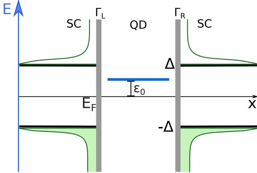
Figure 2.14 – Energy diagram of a S-QD-S junction in the non-interacting approximation. In this approximation the QD is modeled as a single orbital with position  $\epsilon_0$  with respect to the Fermi energy  $E_F$ .
