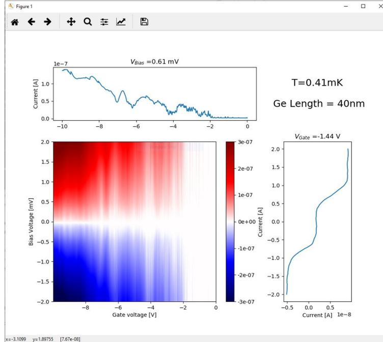
Figure 4.11 – Graphical User Interface (GUI) produced by the python script `'diamonds.py'` showing a density plot of  $I_D(V_G$  with  $V_G$  and  $V_D$  slices plotted to the right and top, respectively. A user can click on the density plot to select  $V_G$  and  $V_D$  slices.
