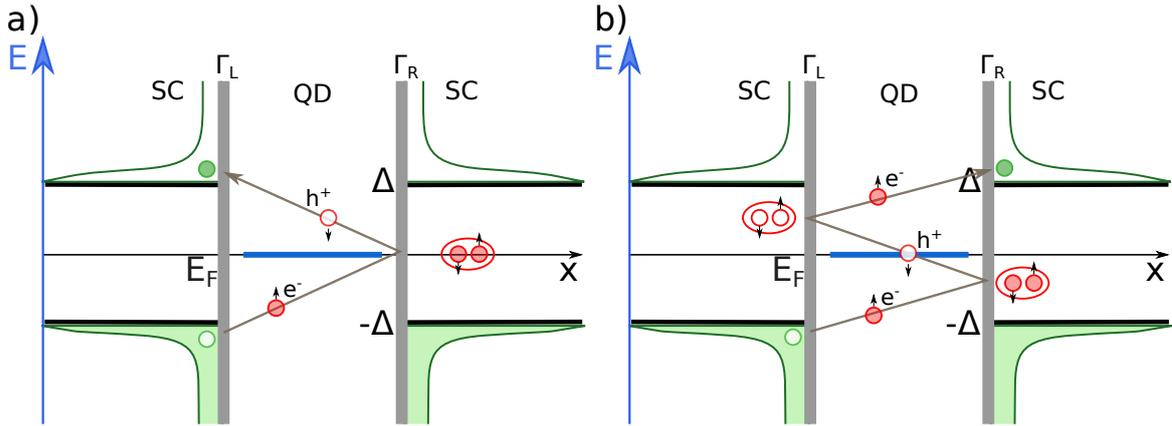
Figure 2.18 – Schematic showing resonant MAR processes of 2nd (a) and 3rd (b) order MAR through a S-QD-S junction. The QD orbital  $\epsilon_0$ , defined by the thick blue line, is on resonance with  $E_F$  of the leads. In (a) the 2nd order MAR does not align with  $\epsilon_0$  as such the usual MAR current jump is suppressed. However, in (b) the 3rd order MAR process does align with  $\epsilon_0$  as such the current jump is enhanced and we observe a current peak.
