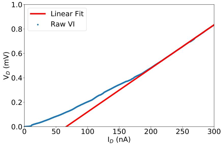
Figure 6.11 – Raw  $V_D$ - $I_D$  curve at  $V_G = -29$  V and linear fit of the curve in the normal regime  $V_D > 2\Delta/e$ . From the linear fit,  $R_N$  and  $I_{exc}$  is determined.  $R_N = 3.6$  k $\Omega$  is the gradient of linear fit and  $I_{exc} = 66$  nA is the x-axis intercept.
