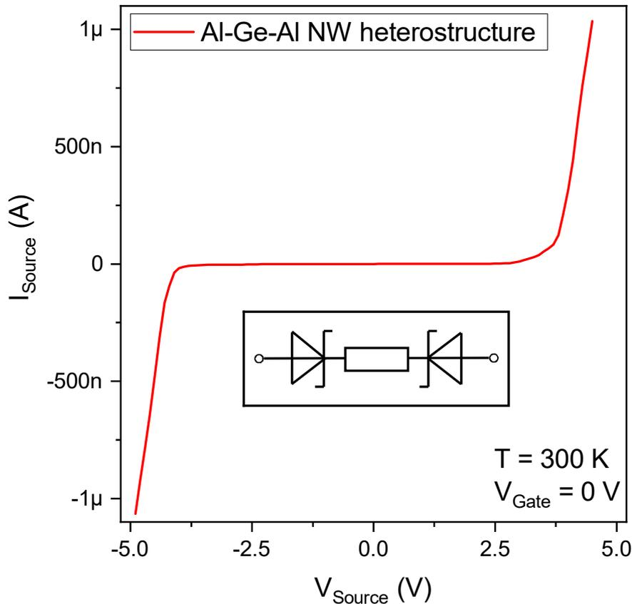
Figure 5.5 – Characteristic  $I_D$ - $V_D$  curve of a Al-Ge-Al nanowire heterostructure with a Ge segment length of 550 nm after the annealing process measured at room temperature ( $T \approx 300$  K) and  $V_G = 0$  V. Figure taken from Ref. [39].
