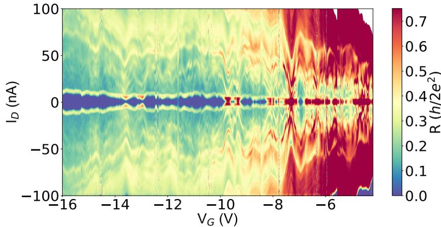
Figure 5.27 – **Overview of the superconducting regime:** Colorplot of differential resistance ( $R$ ) vs bias current ( $I_D$ ) and back gate voltage ( $V_G$ ). We observe the zero-bias resistance peaks due to low bias blockade evolving into low bias zero resistance region due to superconducting transport as  $V_G$  decreases. This superconducting region results from the proximity effect of the Al contacts and the removal of Schottky barrier by the large negative back gate voltage.
