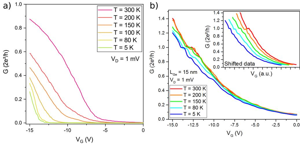
Figure 5.12 – Characteristic  $G-V_G$  curves measured for  $V_D = 1$  mV over a range of temperatures ( $T$ ) of Al-Ge-Al devices with (a) long ( $L_{\text{Ge}} = 250$  nm) and (b) short ( $L_{\text{Ge}} = 15$  nm) Ge segment lengths. Figure taken from Ref. [104].
