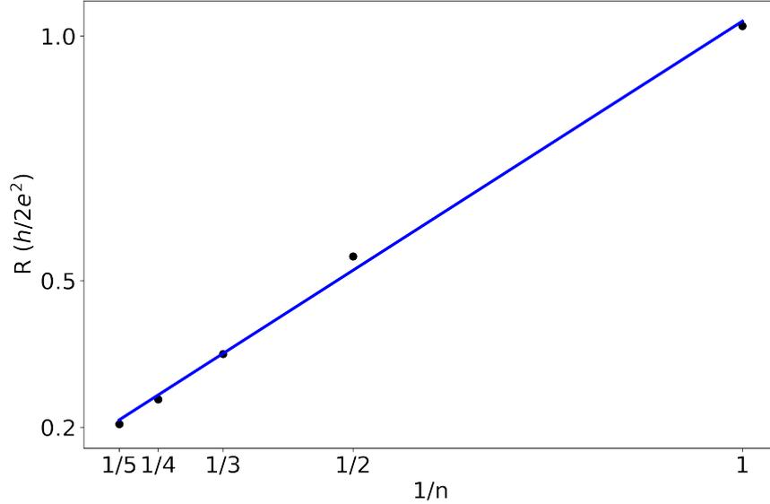
Figure 6.3 – Resistance ( $R$ ) of the quantised conductance plateaus of Fig. 6.2 vs the inverse of the conducting channel number ( $1/n$ ). The linear fit is used to estimate the interface transparency.
