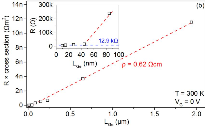
Figure 5.9 – Resistance, calculated from  $I_D$ - $V_D$  curves of Figure 5.8 and multiplied by the Ge NW's cross sectional area, versus  $L_{\text{Ge}}$ . Inset shows a zoom of actual resistance  $R$  versus  $L_{\text{Ge}}$  of devices with  $L_{\text{Ge}} < 100$  nm. Figure taken from Ref. [104].
