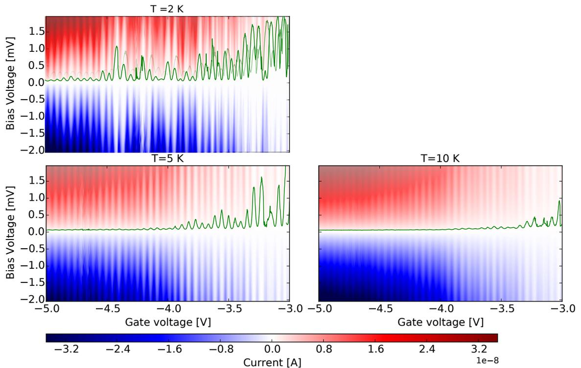
Figure 5.25 – Stability diagrams showing Coulomb diamonds of the device at different temperatures. Showing the measured current versus  $V_D$  and  $V_G$  of an heterostructure device with  $L_{Ge} = 162$  nm recorded at  $T = 350$  mK, 2 K, 5 K and 10 K. Green lines are iso-current curves extracted from the 2D plots. For these curves the current through the nanowire is equal to 0.5 nA.
