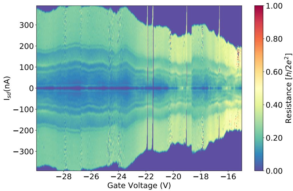
Figure 6.8 – Transport overview of superconducting regime. Density plots of differential resistance  $R = dV_D/dI_D$  plotted in units of the quantum resistance versus  $I_D$  and  $V_G$ .
