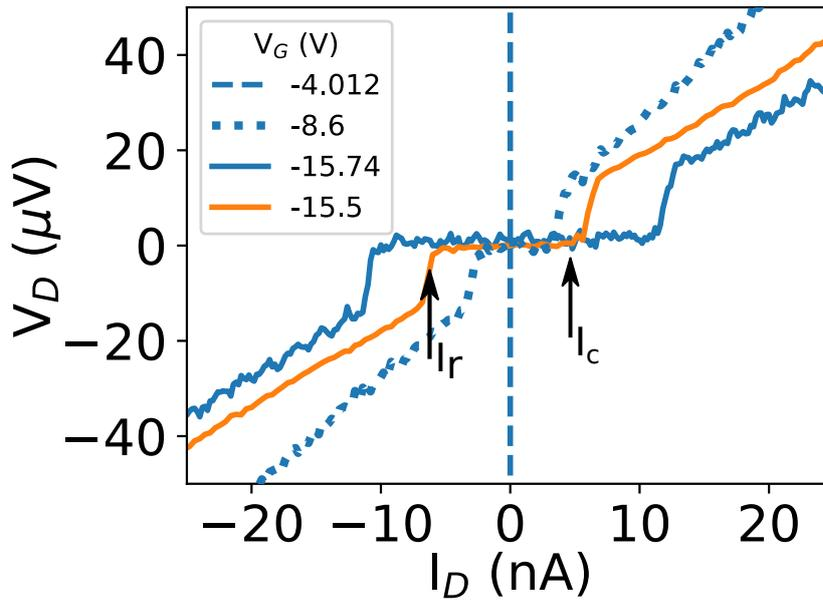
Figure 5.33 –  $V_D$  versus  $I_D$  for four  $V_G$  slices showing the onset of supercurrent. For comparison both Sample 1 (blue curves) and Sample 2 are shown (orange curve). Retrapping  $I_r$  and critical current  $I_c$  are labeled.
