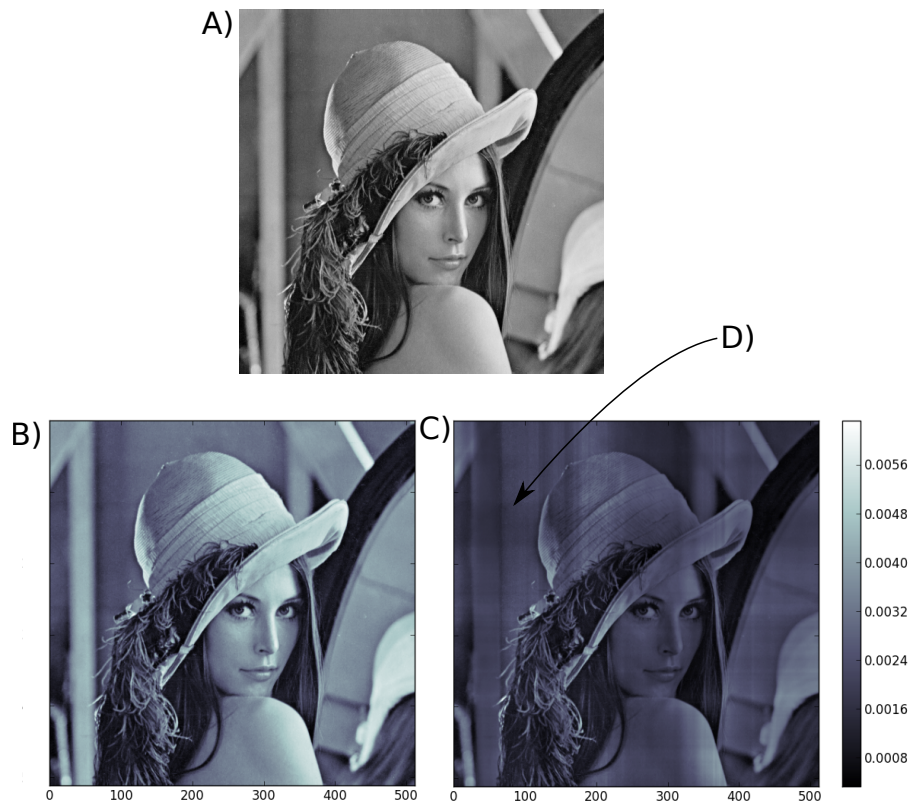
Figure 3.1: Iterative normalization procedure. A) The raw image. C) is the normalized image while B) is just a scaled version of A) so that B) and C) have the same global intensity. There are no details lost by the process but there are artifacts generated, as displayed in D), and the overall contrast of the image is lowered.
