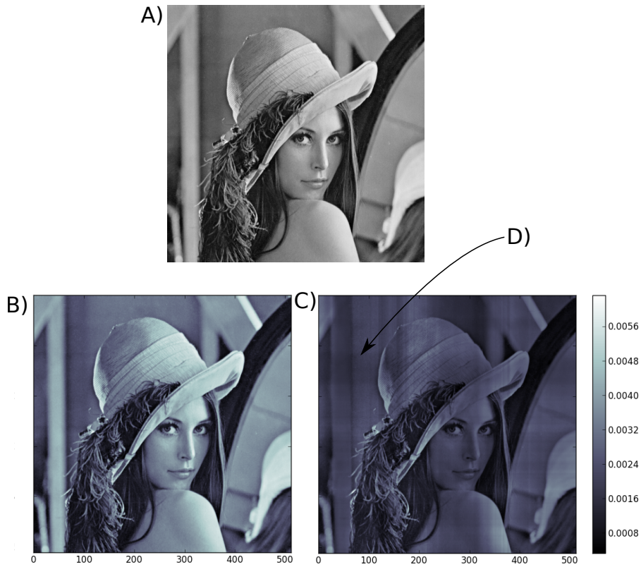
Figure 3.1: Iterative normalization procedure. A) The raw image. C) is the normalized image while B) is just a scaled version of A) so that B) and C) have the same global intensity. There are no details lost by the process but there are artifacts generated, as displayed in D), and the overall contrast of the image is lowered.
