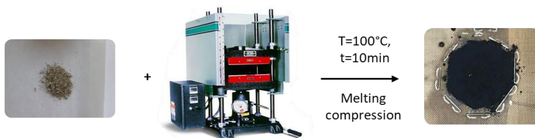
Figure 47. Preparation process for the PCL and PCL- g -PDA films by melting compression
