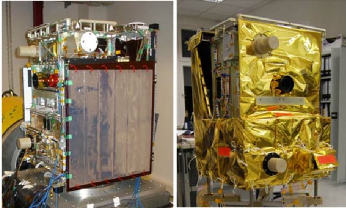
Figure 1.6: Satellite before and after adding Multi-Layer Insulation (MLI) to protect it from extreme radiation. Taken from Fockersperger et al [FLK + 10].
