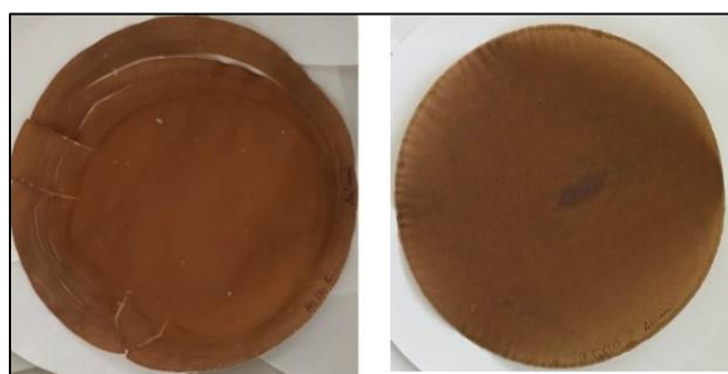
Figure IV. 19: Nanopaper cracking at temperatures above 45°C (left) and a nanopaper dried at 45°C (right)
