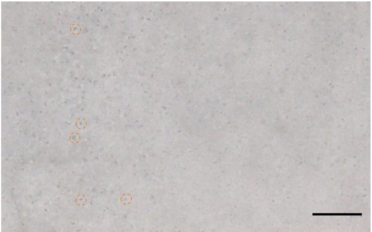
Figure A. 4 - Optical micrograph (AM) of bulk species underneath the film at 35 min of reaction. The dark dots, highlighted by orange dashed circles, are distributed in the depth of the solution.
