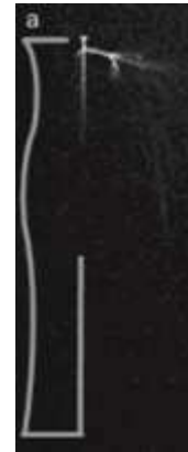
Fig. 22: Photographs of streamers and breakdown on porcelain insulating surface at 77 kV [50].
