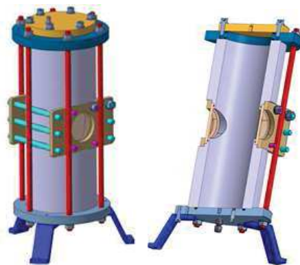
Fig. 10: Second test cell for pressure measurements.
