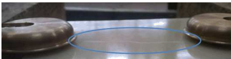
Fig. 1: Photograph of Schneider Electric electrodes for breakdown measurements with solids.
