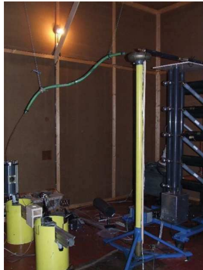
Fig. 6: Marx generator, test cell, and optical bench within the Faraday cage.
