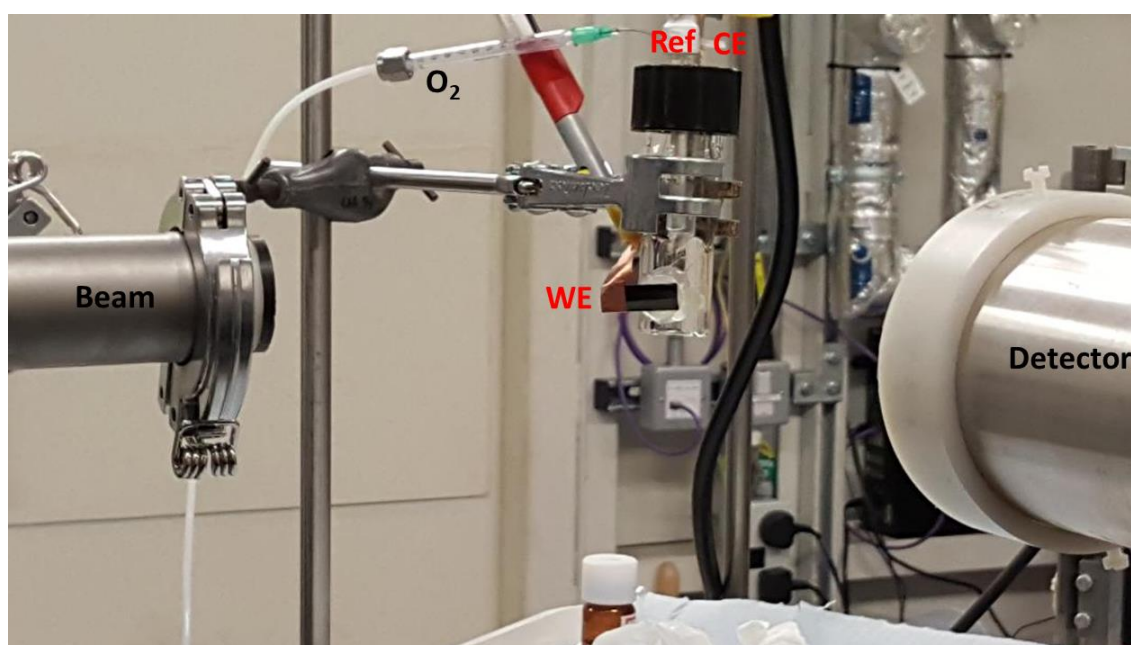
Appendix Figure 5 Simplified scheme of the side view of the in situ electrochemical cell.
