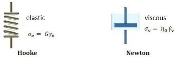
Figure 2.3. Analogical representations and material relationships for the elastic element Hooke and the viscous element Newton [BA06].
